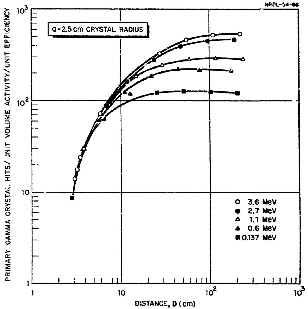
Fig. 4 Response of 2.5 cm radius crystal to gamma ray emitters at unit activity per unit volume, at unit efficiency.
