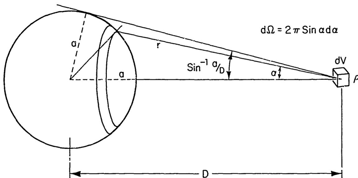
Fig. 1 Solid angle of acceptance on sphere.
