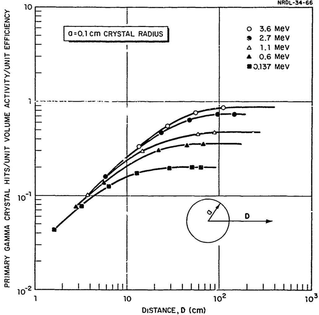
Fig. 2 Response of 0.1 cm radius crystal to gamma ray emitters at unit activity per unit volume, at unit efficiency.
