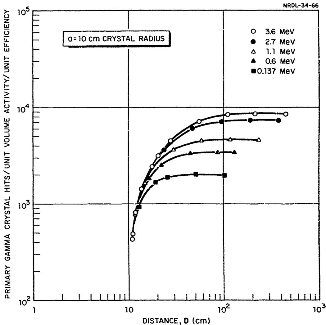
Fig. 6 Response of 10.0 cm radius crystal to gamma ray emitters at unit activity per unit volume, at unit efficiency.
