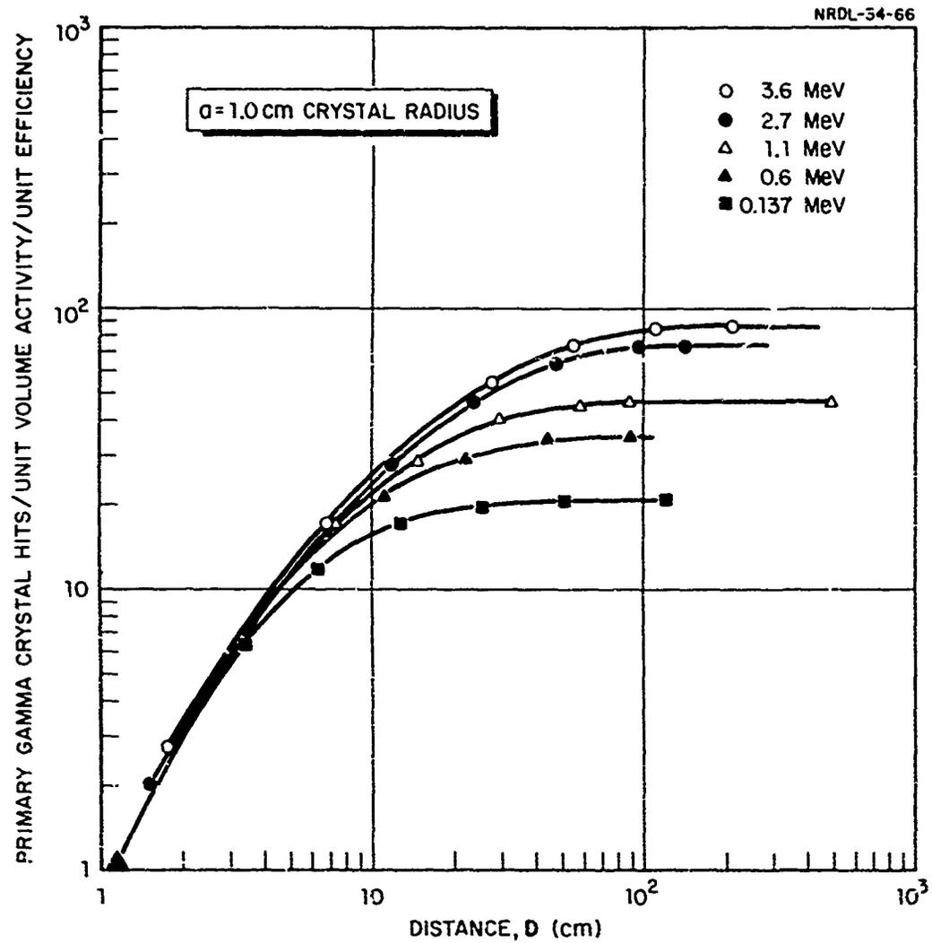
Fig. 3 Response of 1.0 cm radius crystal to gamma ray emitters at unit activity per unit volume, at unit efficiency.
