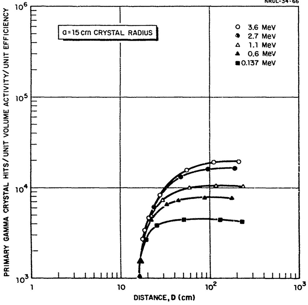
Fig. 7 Response of 15.0 cm radius crystal to gamma ray emitters at unit activity per unit volume, at unit efficiency.
