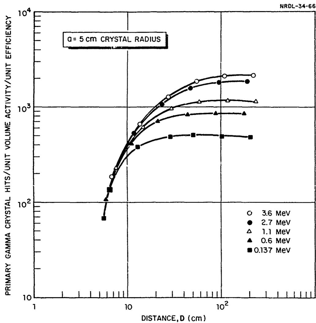
Fig. 5 Response of 5.0 cm radius crystal to gamma ray emitters at unit activity per unit volume, at unit efficiency.
