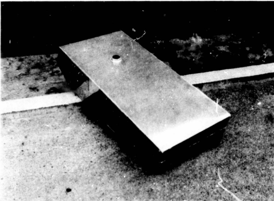
Figure 58. Experimental Aluminum Tank, T-17, Material 0.040-Inch 6061-T4.
