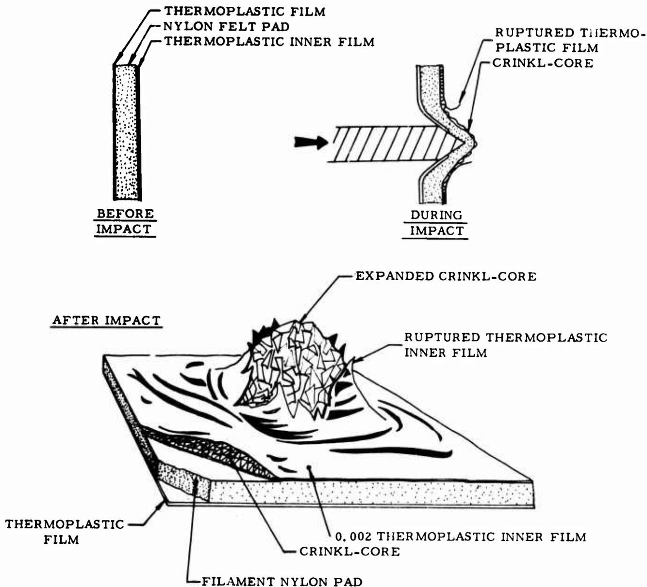
Figure 5. Operational Principle of Crinkl-Core.
