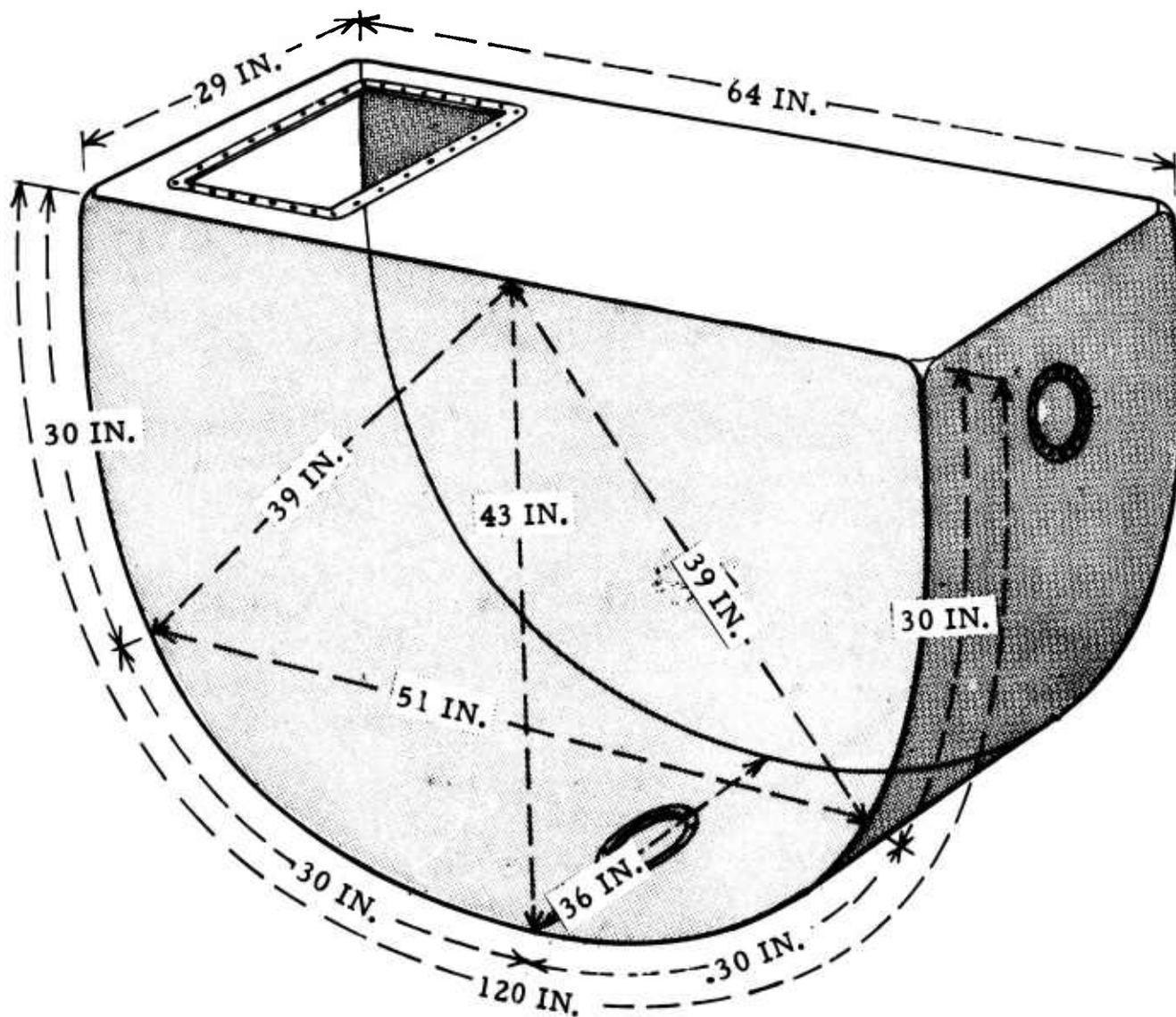
Figure 9. Dimensional Cutaway of Fuel Cell.
