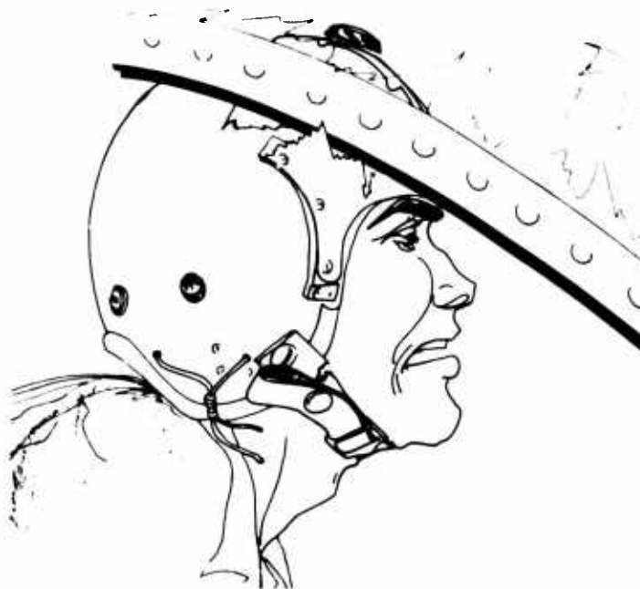
Figure 1. Artist's Sketch Illustrating How a Helmet Can Be Removed by Impact with Cockpit Structure.
