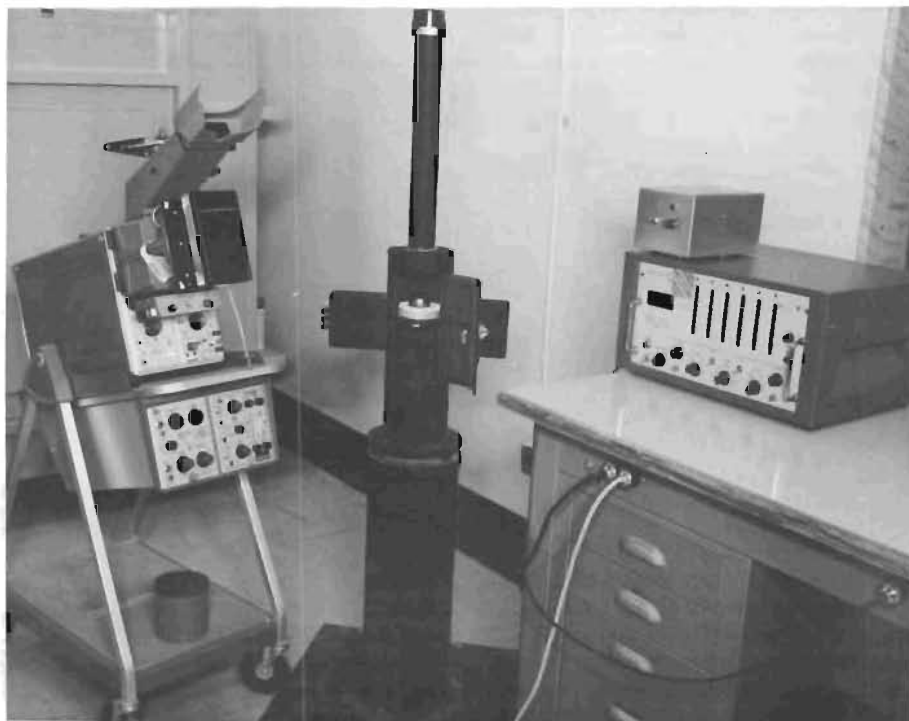
Fig. 7. Shock calibrator for determining accelerometer resonance
