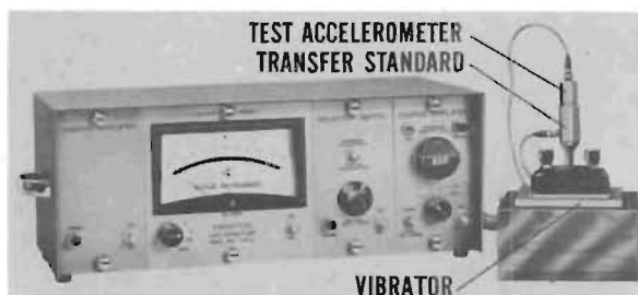
Fig. 6. Precision back-to-back vibration calibrator
