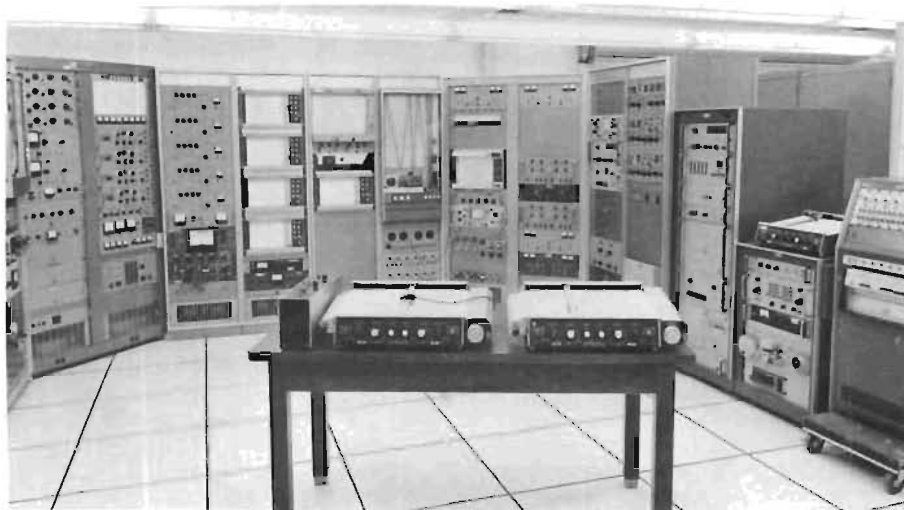
Fig. 1. The analog cross spectral density analyzer system
