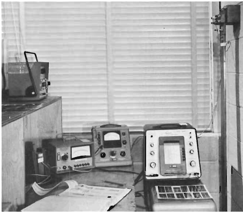
Fig. 1. Instrumentation used for base strain sensitivity measurements
