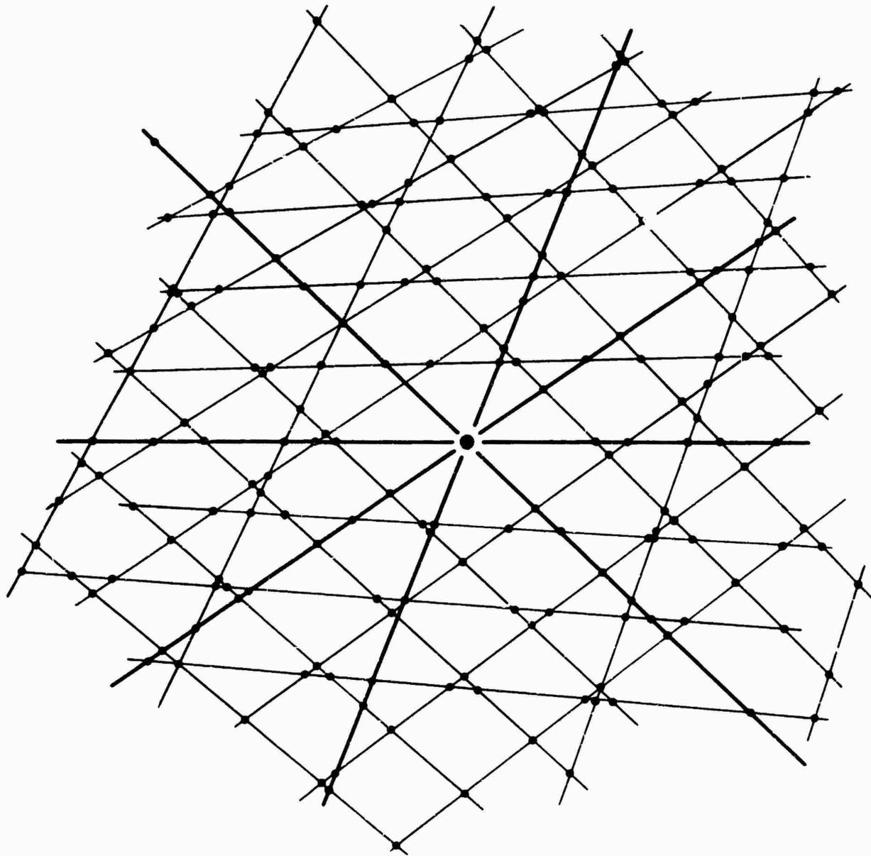
FIGURE 2.4-4. AMBIGUITY RESOLUTION BY MULTIPLE INTERSECTION
