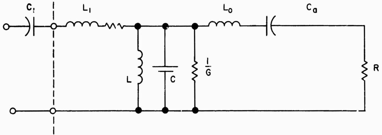
FIG. 6.5-1 ANTENNA COUPLING CIRCUIT AND EQUIVALENT CIRCUIT
