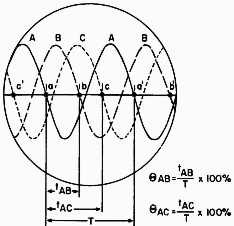
FIGURE 8.2-1. OSCILLOSCOPE PHASE INDICATOR
