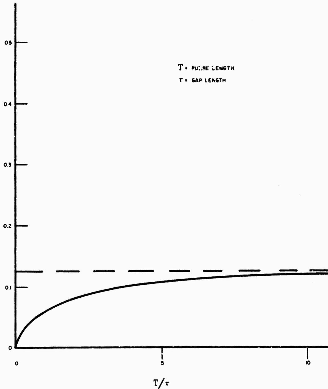
FIGURE 2.3-2. MULTIPLEX DUTY RATIO
