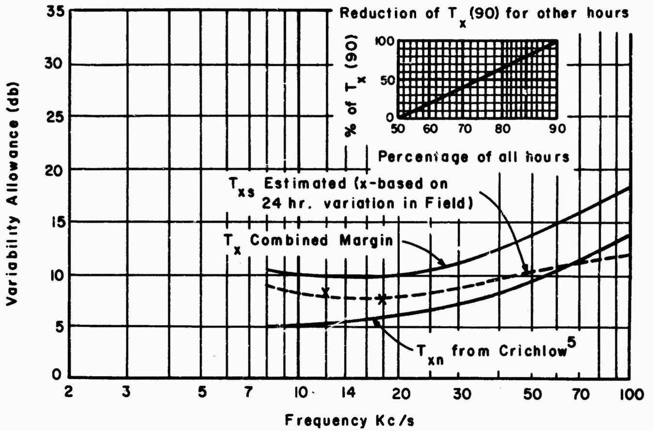
FIGURE 6.2-5. SIGNAL FADING AND NOISE VARIATION MARGIN FOR 90% OF ALL HOURS
