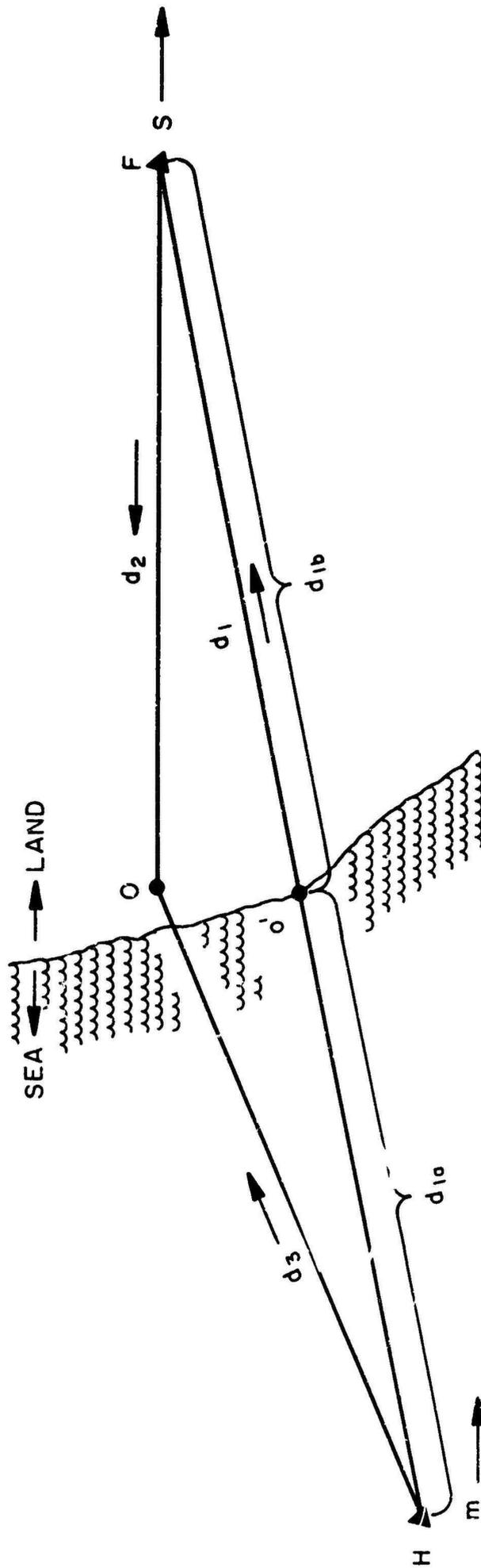
FIGURE 3.2-1. TYPICAL PATH GEOMETRY SHOWING MASTER, SLAVE, AND OBSERVER POSITIONS FOR PROPAGATION INCLUDING BOTH SEA AND LAND PATHS
