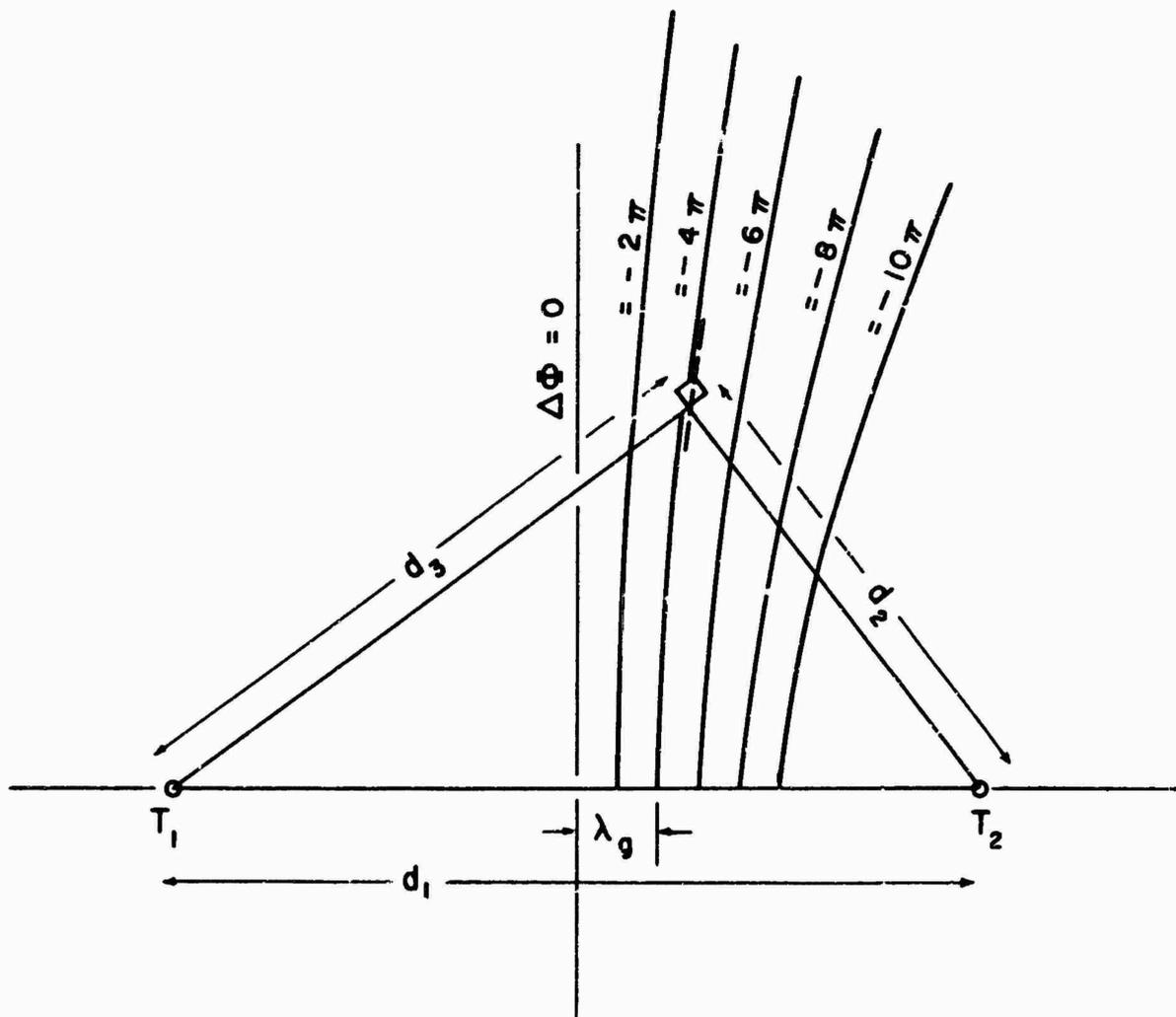
FIGURE 3.4-1. HYPERBOLIC GEOMETRY SHOWING ERROR IN LINE OF POSITION CAUSED BY VELOCITY ERROR
