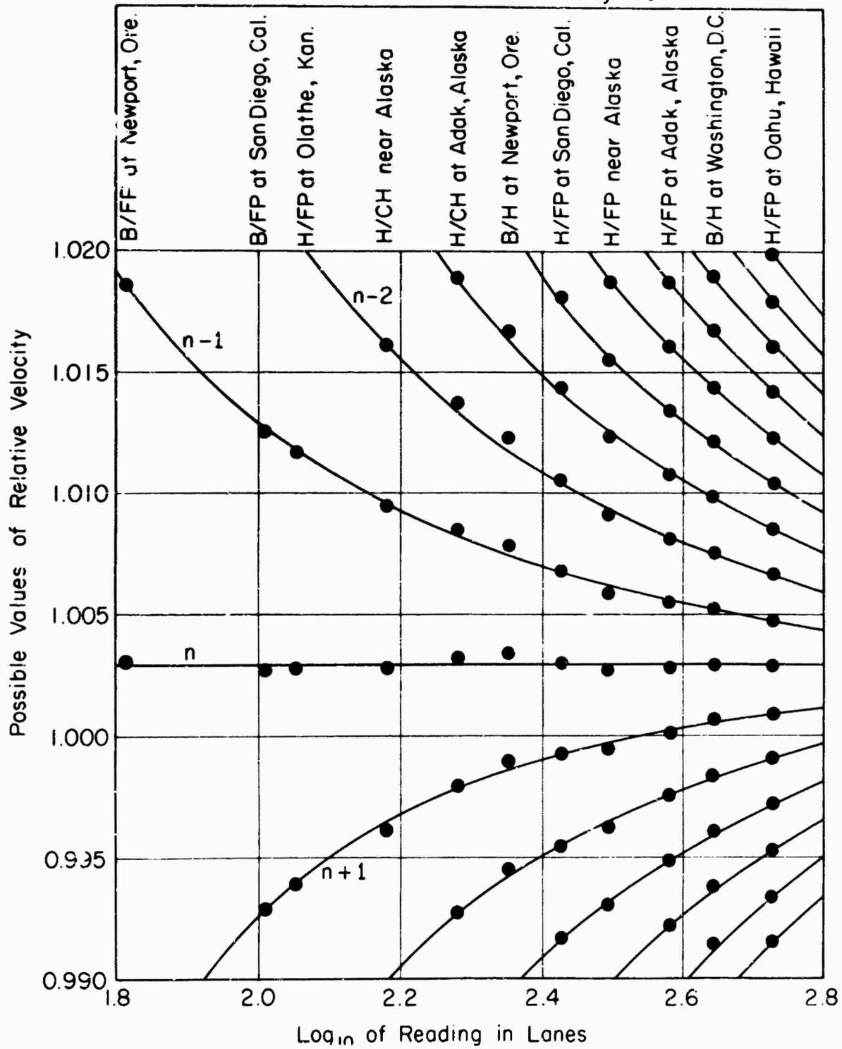
FIGURE 3.2-2. PLOT OF EXPERIMENTAL DATA IN THE FORM OF VARIOUS POSSIBLE VALUES OF RELATIVE VELOCITY IN ORDER TO DETERMINE THE TRUE PHASE VELOCITY FOR DAYTIME PROPAGATION OF 10.2 KC SIGNALS (FROM PIERCE AND NATH)
