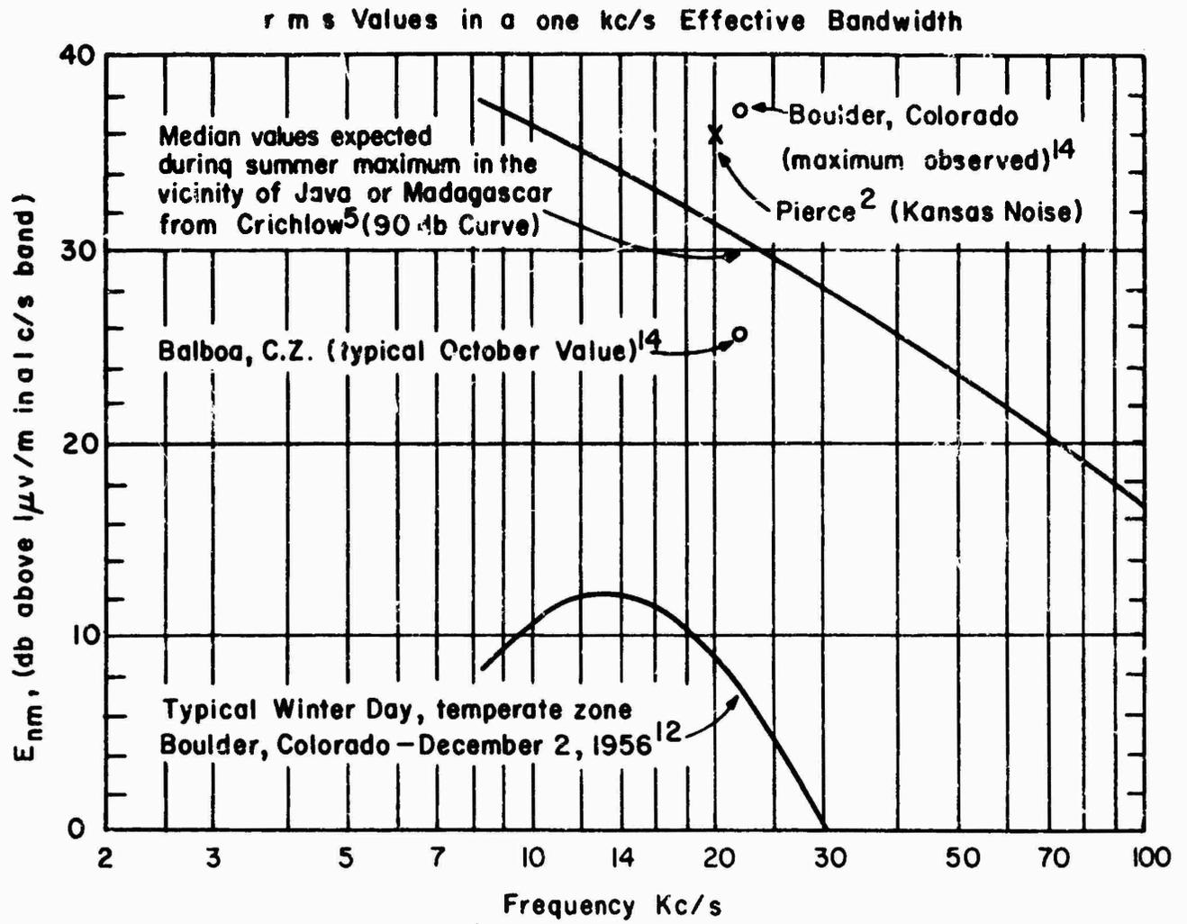
FIGURE 6.2-4. TYPICAL ATMOSPHERIC NOISE FIELD STRENGTHS
