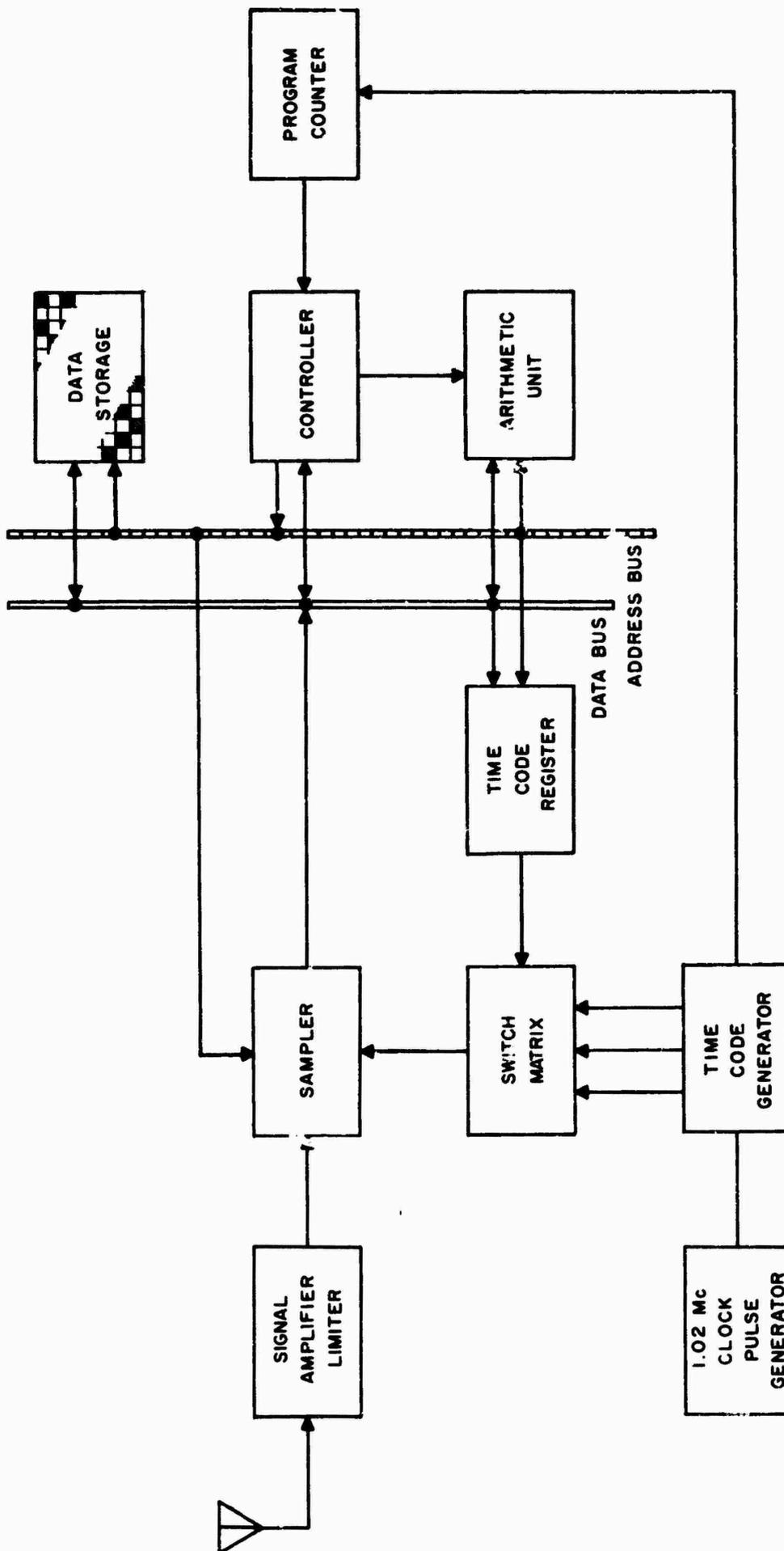
FIG. 8.7-4 COMPUTER DATA PROCESSOR
