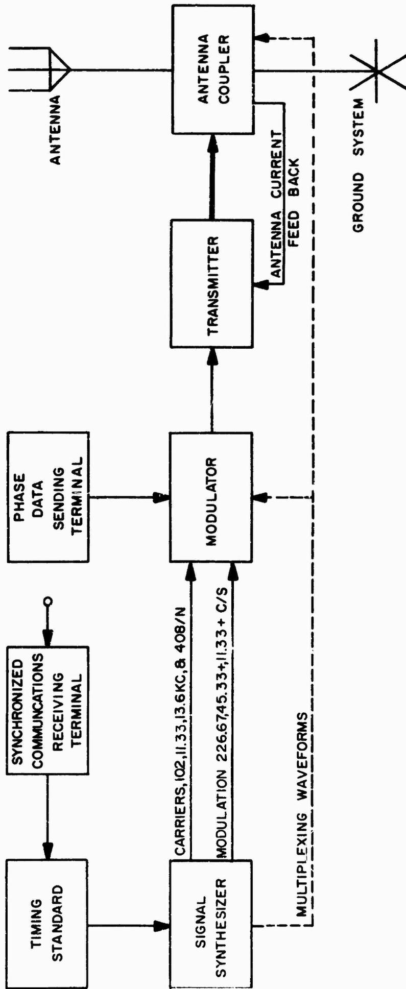
FIG. 6.6-1 TRANSMITTER TIMING SYSTEM
