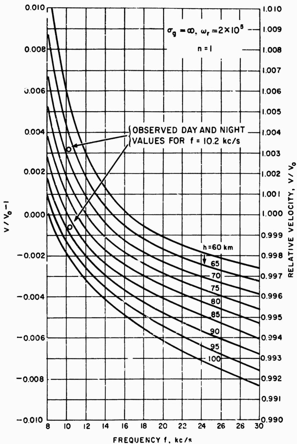
FIGURE 3.2-4. THEORETICAL VALUES OF RELATIVE PHASE VELOCITY FROM WAIT (1962) SHOWING RELATIVE PHASE VELOCITY AS A FUNCTION OF FREQUENCY FOR VARIOUS EFFECTIVE IONOSPHERIC HEIGHTS. EXPERIMENTAL DAY AND NIGHT VALUES FROM THE PRECEDING FIGURE FOR OVER SEA WATER PROPAGATION ARE ALSO SHOWN AT 10.2 KC
