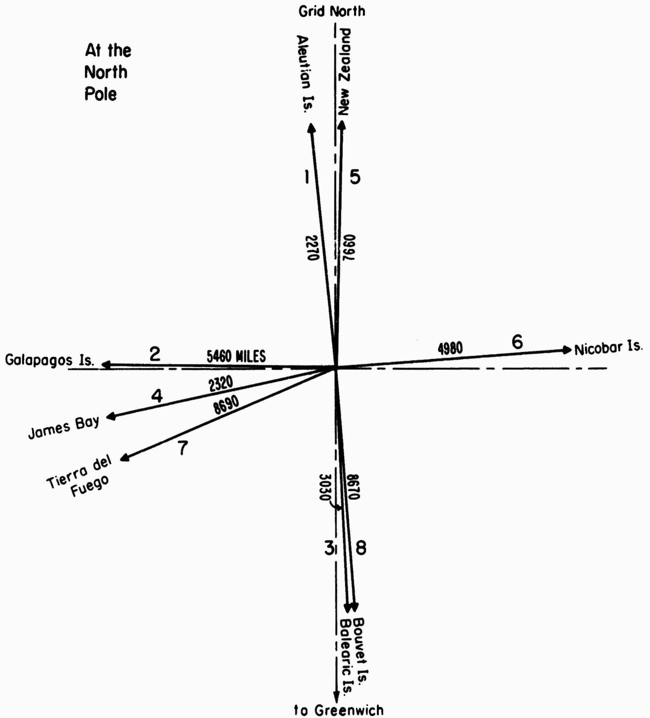
FIGURE 2.2-9. DIRECTIONS AND DISTANCES OF EIGHT STATIONS FROM THE NORTH POLE
