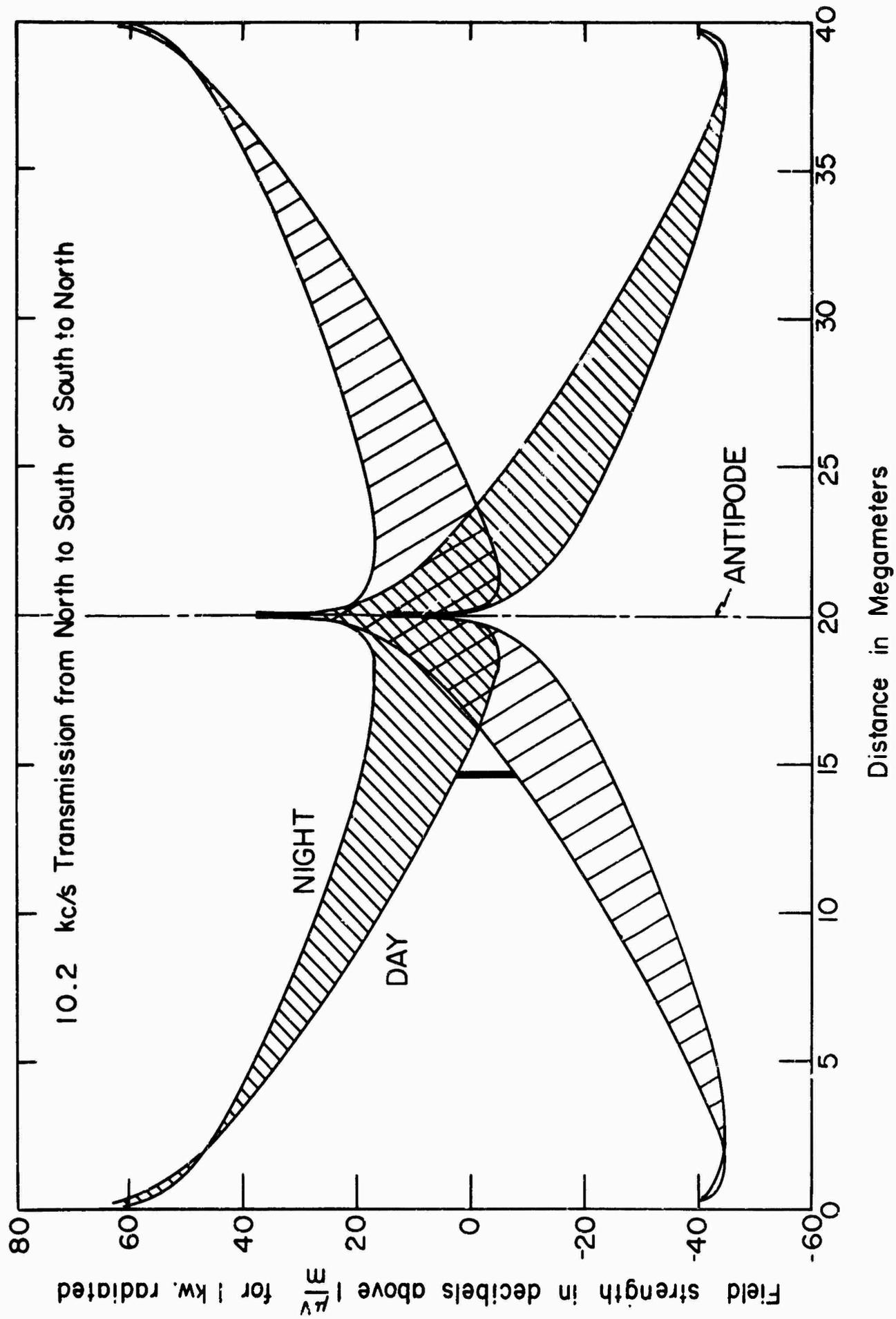
FIG. 6.2-1 10.2 KC TRANSMISSION FROM NORTH TO SOUTH OR SOUTH TO NORTH
