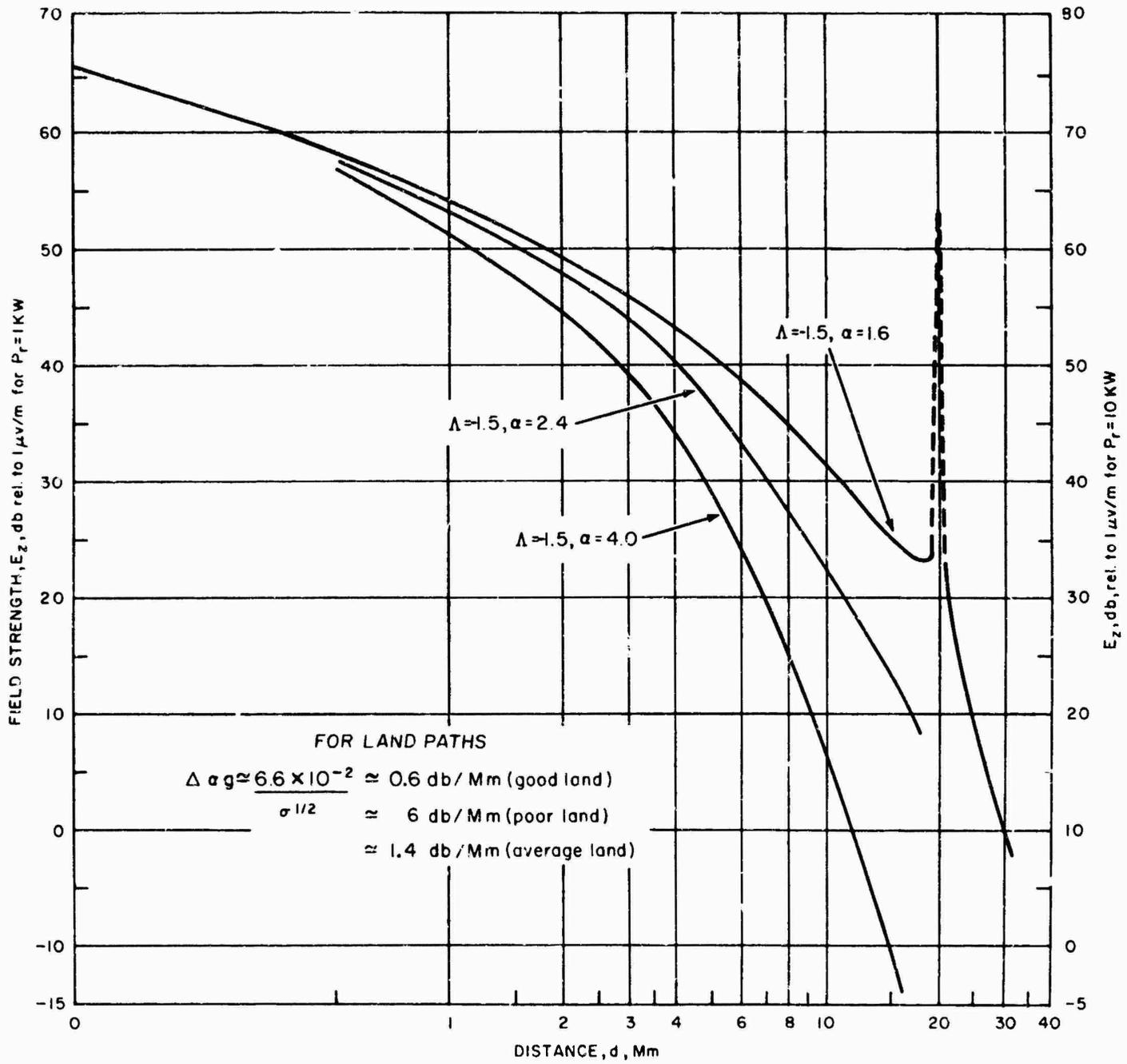
FIGURE 3.1-3. DAYTIME FIELD STRENGTH VERSUS DISTANCE AT 10.2 KC
