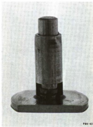
Fig. 23. Assembly fixture for Madel 1 laser element.
