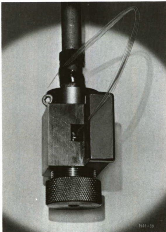
Fig. 42. Cartridge containing laser array with fiber optics.
