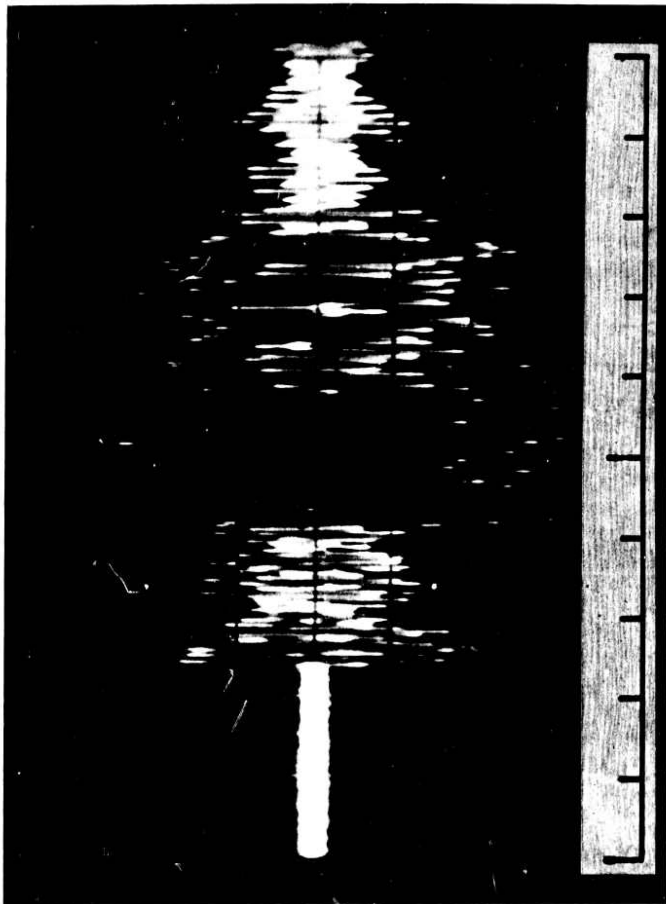
Figure 34. Oscillogram: IMC Mine, F-IV Units, Transmitter at 4N-150, Receiver at R-18-81 Units at Right Angle to Each Other.
