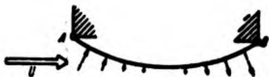
Fig. 19.1. Panel under influence of flow of gas; distribution of normal pressure.
