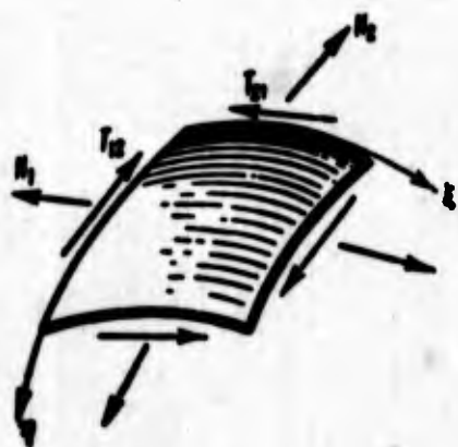
Fig. 10.24. Positive directions of forces in middle surface.
