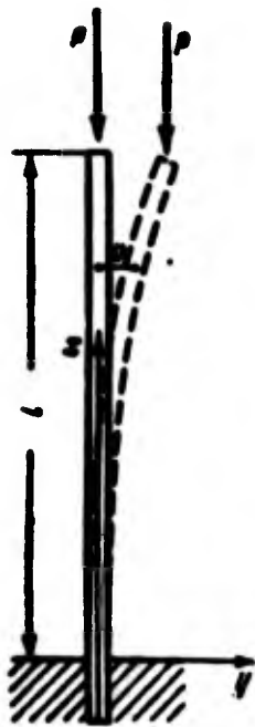
Fig. 1.7. Bar, clamped at one end and free at the other.
