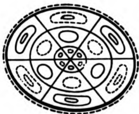
Fig. 9.8. Asymmetric buckling of circular plate.
