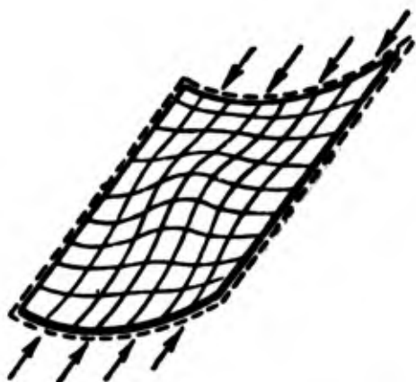
Fig. 10.4. Cylindrical panel "prefers" to buckle toward the center of curvature.
