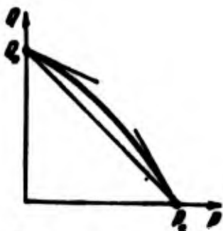
Fig. 21.9. Approximate determination of boundary line for zone of stability.
