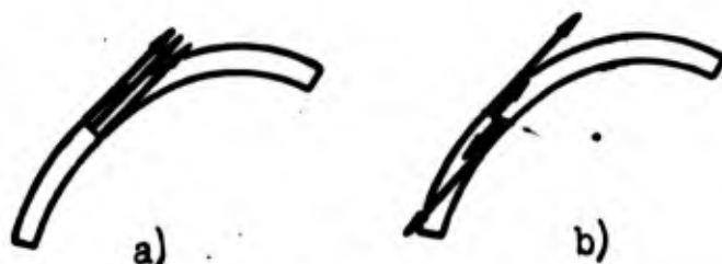
Fig. 4.3. Tangential stresses. a) of constrained torsion, b) of free torsion.
