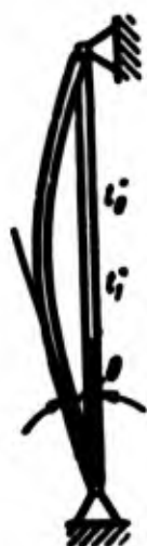
Fig. 5.2. Bar with fixed ends with vari- able tem- perature.
