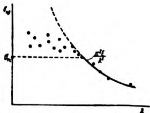
Fig. 2.1. Scattering of experimental values of critical stresses in plastic region.
