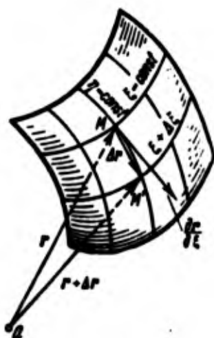
Fig. 10.9. Radius-vector of a point of a surface as a function of curvilinear coordinates.
