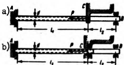
Fig. 3.15. Calculation of feed spindle of lathe-screw machine.
