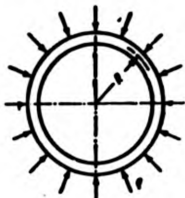
Fig. 3.31. Ring under action of radial load.
