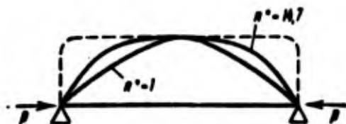
Fig. 9.17. Deflection surface of circular plate at different stages of postcritical deformation.
