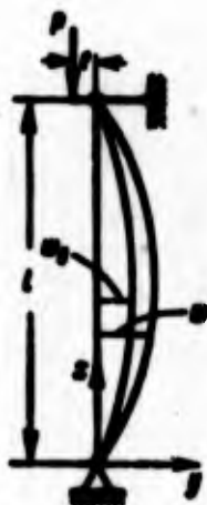
Fig. 20.7. Bar with initial deflection, subjected to eccentric compression.
