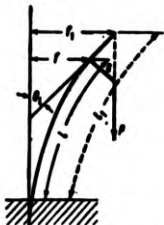
Fig. 1.28. Exact solution of problem of eccentric compression of bar.
