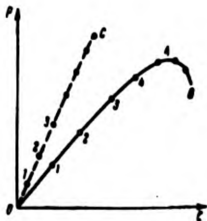
Fig. 15.10. Diagrams "load-deflection" according to calculations on digital computers.
