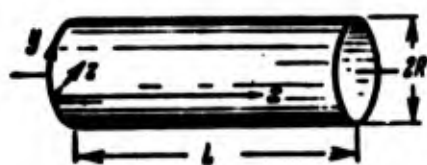
Fig. 11.1. Coordinate lines for examining cylindrical shell.
