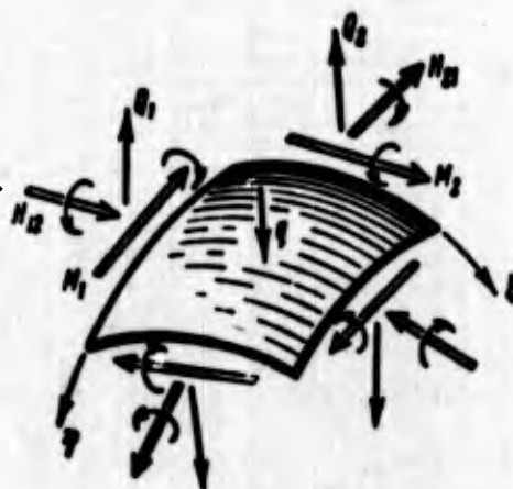
Fig. 10.25. Positive directions of moments, transverse forces and lateral load.
