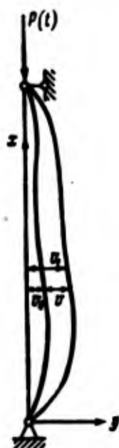
Fig. 6.1. Bar with initial deflection receiving dynamic load.
