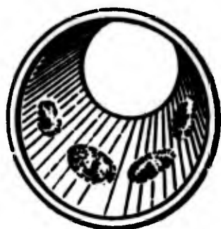
Fig. 11.69. Character of wave formation during local application of external pressure.
