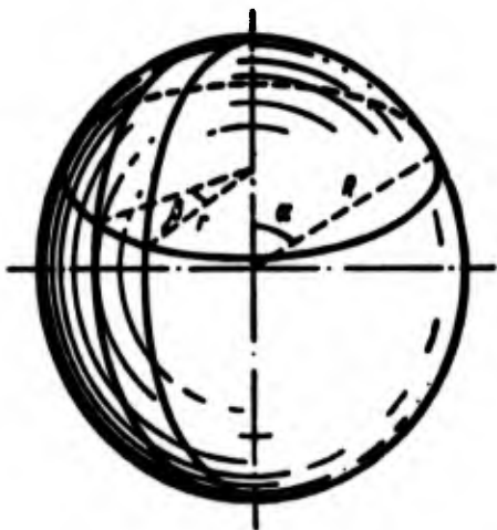
Fig. 14.4. Coordinate lines for examining spherical shells.
