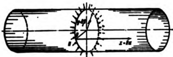
Fig. 11.70. Calculation for stability of shell in zone of application of concentrated load.
