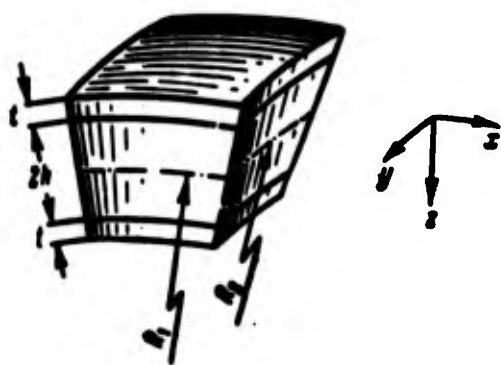
Fig. 16.4. Member of a sandwich shell.
