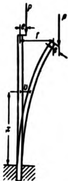
Fig. 1.27. Bar with clamped end under action of eccentric- ally applied load.
