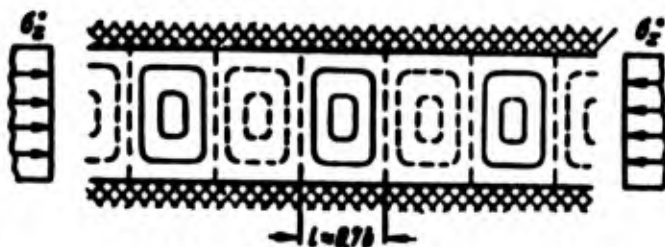
Fig. 7.19. Wave formation of elongated plate, clamped on long edges.
