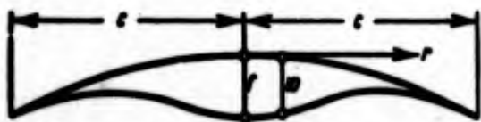
Fig. 14.6. Form of dent during axisymmetric buckling of spherical shell.
