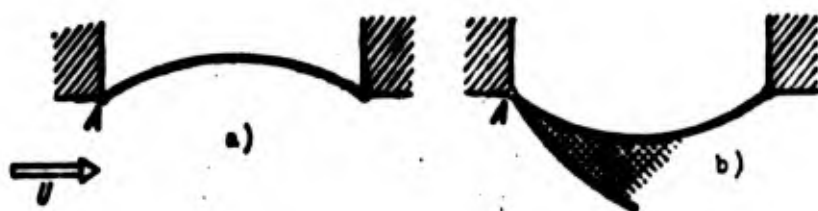
Fig. 19.4. Different cases of distortion of a panel, a) convexity upwards, b) convexity downwards.
