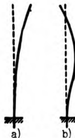
Fig. 1.33. Forms of vibrations during action of follow-up force.
