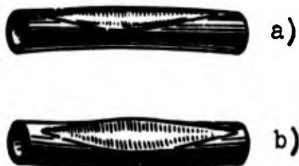
Fig. 11.42. Buckling during bending in "long waves."
