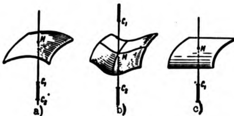
Fig. 10.15. Location of centers of curvature C_1 and C_2 for (a) elliptic, (b) hyperbolic and (c) parabolic points of a surface.
