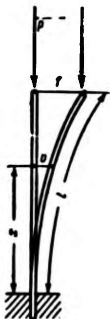
Fig. 1.12. For exact solution of problem of supercritical deformation of a bar.
