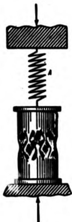
Fig. 11.9. Shell in testing machine.
