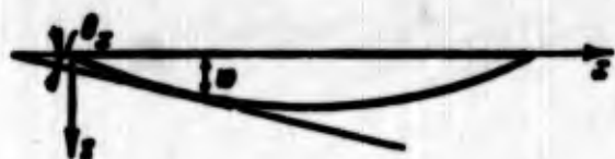
Fig. 7.3. Cross-section of deflection surface of plate.
