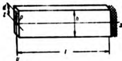
Fig. 4.22. Case, when force is applied not in center of gravity of section.
