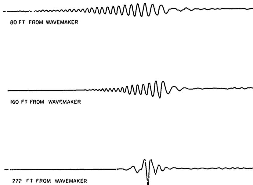
Figure 28 - Transient Wave Form Measured at Various
