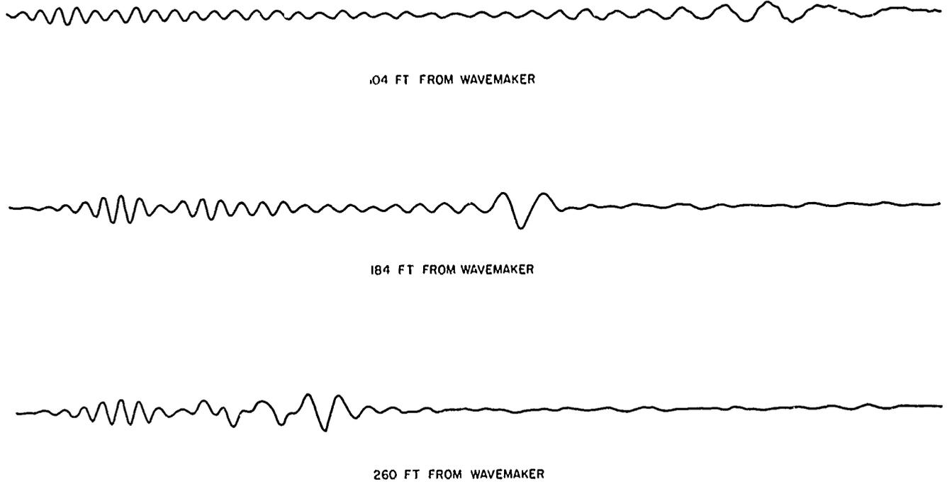
Figure 27 - Transient Wave Form Measured at Various Locations in Basin,
