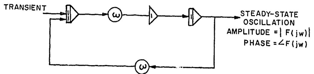
Figure 5 - Transient Analyzer Configuration on Analog Computer
