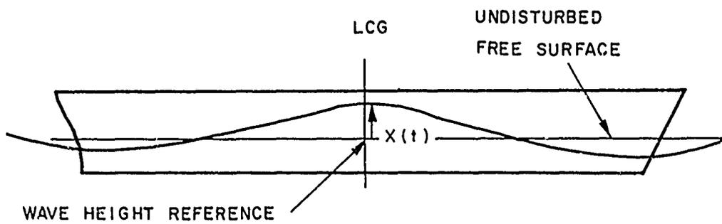
Figure 2 - Wave Height Defined as an Input Signal
