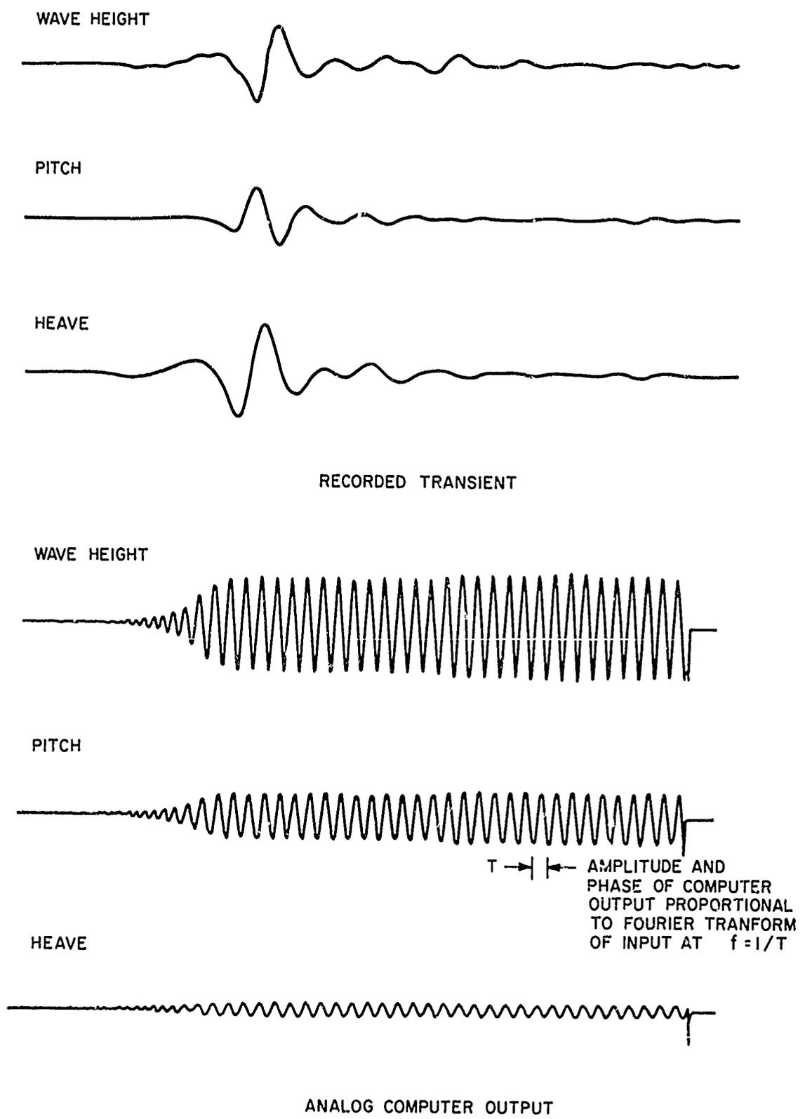
Figure 6 - Measured Transients for Model 4941 and Typical Analog Computer Frequency Response Measurement
