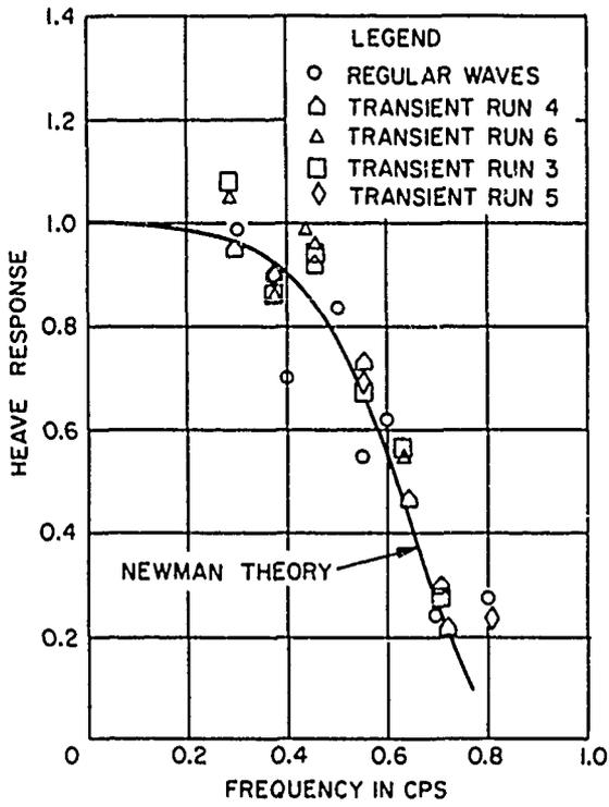
Figure 13 - Heave Response for Model 4606 at Zero Speed in Head Waves
