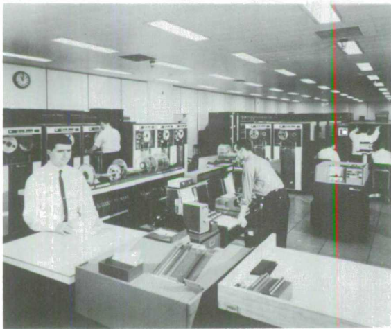
General view of the computer area on the lower level of the Systems Design Laboratory containing most of the components of the IBM 7030 computer.
