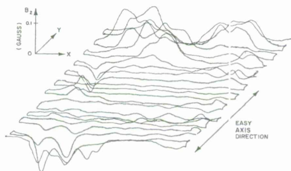
This illustration shows the uniformity of a 3 x 3 inch, thin magnetic film. The mountains and valleys are at the boundaries between differently magnetized areas, which occur when the film is in a partially switched state. The apparent third dimension corresponds to a vertical component of magnetic field.
