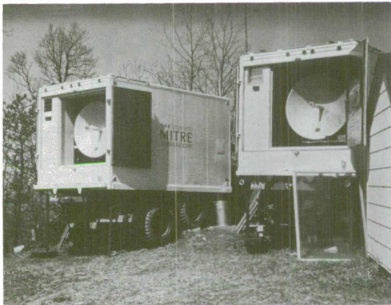
Line integral refractometer receivers aligned for reception of simultaneous, dual-frequency transmission at 15.6 Gc and 31.2 Gc. Each receiver measures the differential phase shift between the signals that are introduced along the path by the water vapor absorption at 22 Gc.
