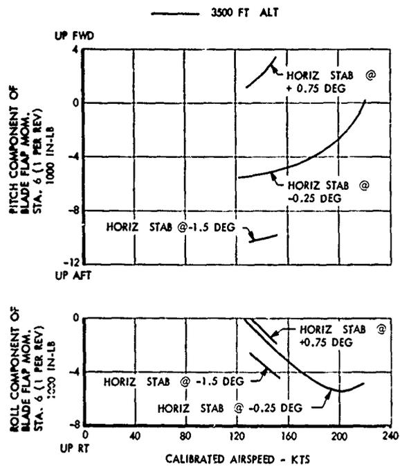
Figure 26. Roll and Pitch Component Versus Calibrated Airspeed
