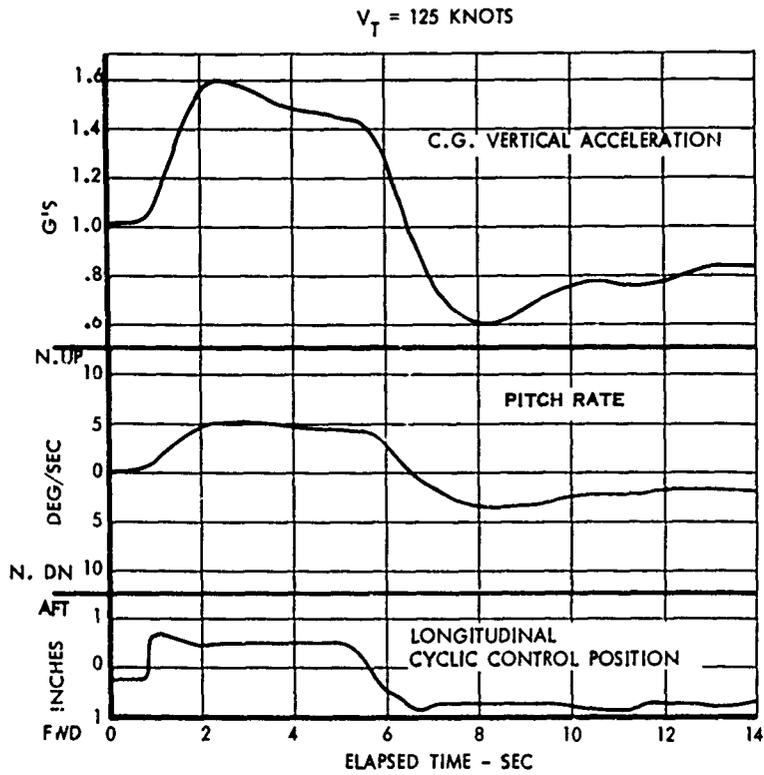
Figure 18. Time History of Longitudinal Control Power - 125 Knots
