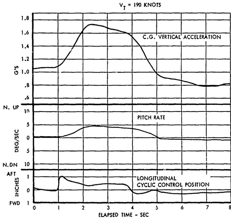
Figure 19. Time History of Longitudinal Control Power - 190 Knots
