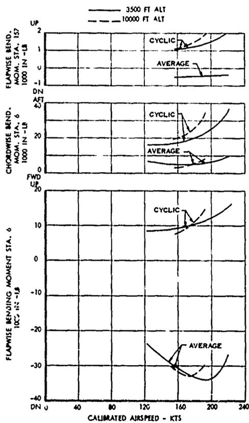
Figure 27. Main Rotor Blade Loads Versus Calibrated Airspeed
