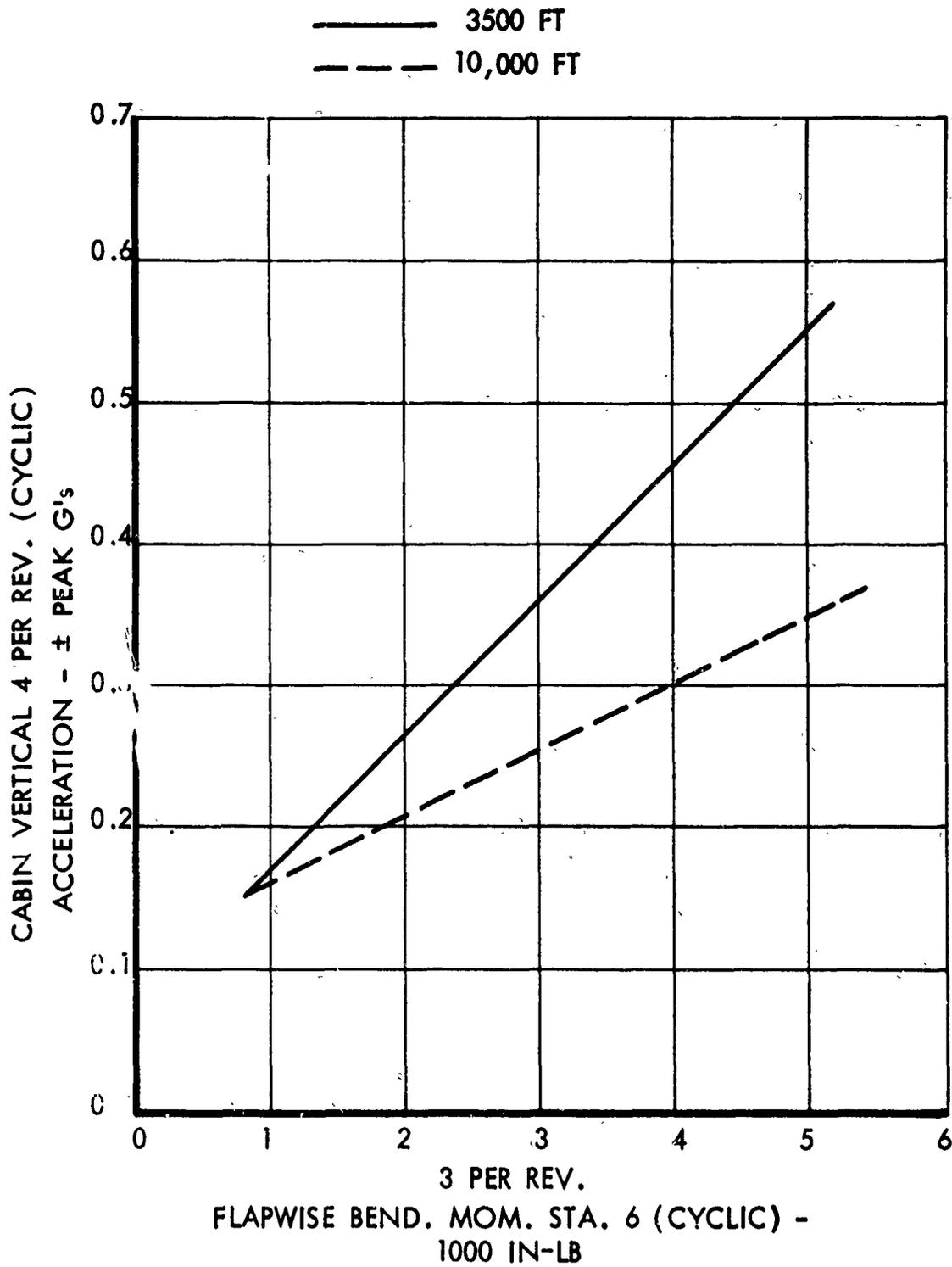
Figure 42. Cabin Vertical Vibration Versus Flapwise Bending Moment
