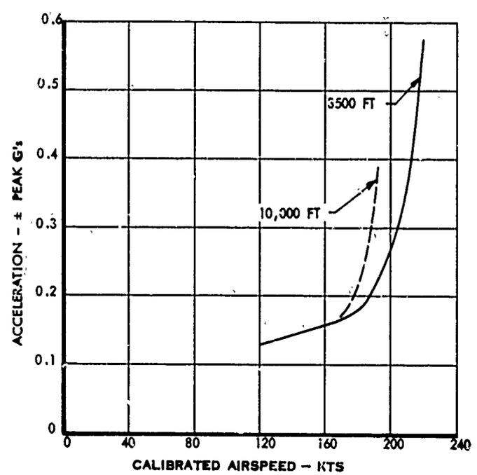
Figure 41. Cabin Vertical Vibration Versus Calibrated Airspeed
