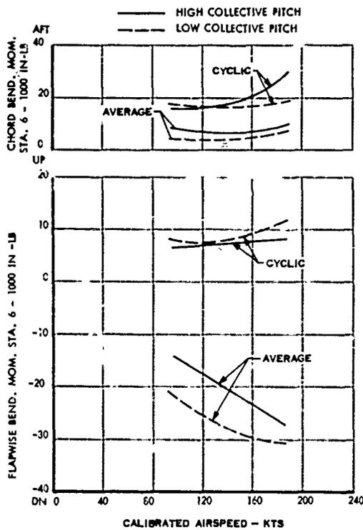
Figure 34. Main Rotor Loads Versus Calibrated Airspeed
