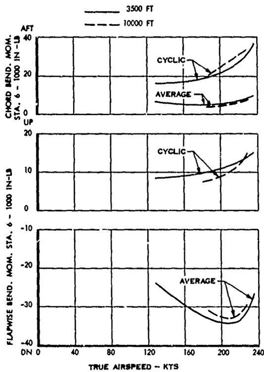
Figure 29. Rotor Characteristics Versus Calibrated Airspeed
