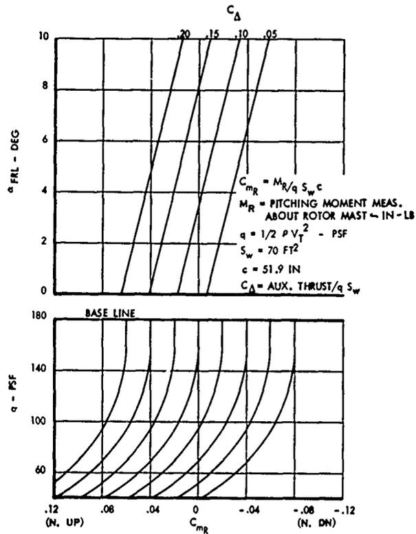
Figure 12. Static Longitudinal Stability and Trim Requirements
