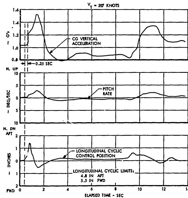
Figure 23. Longitudinal Damping and Control Response Lag - 207 Knots
