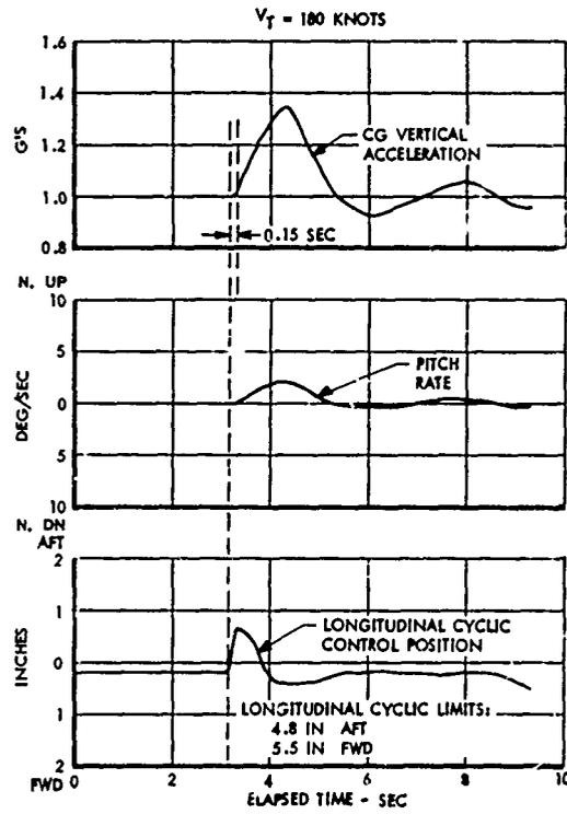
Figure 22. Longitudinal Damping and Control Response Lag - 180 Knots
