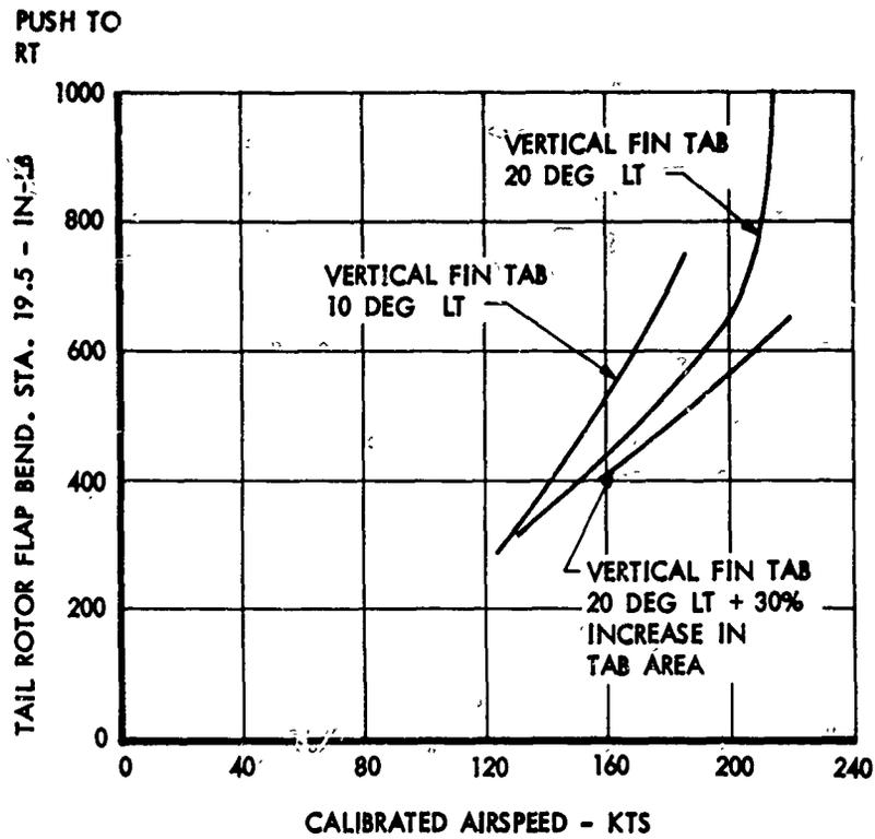
Figure 36. Tail Rotor Flapwise Bending Versus Calibrated Airspeed
