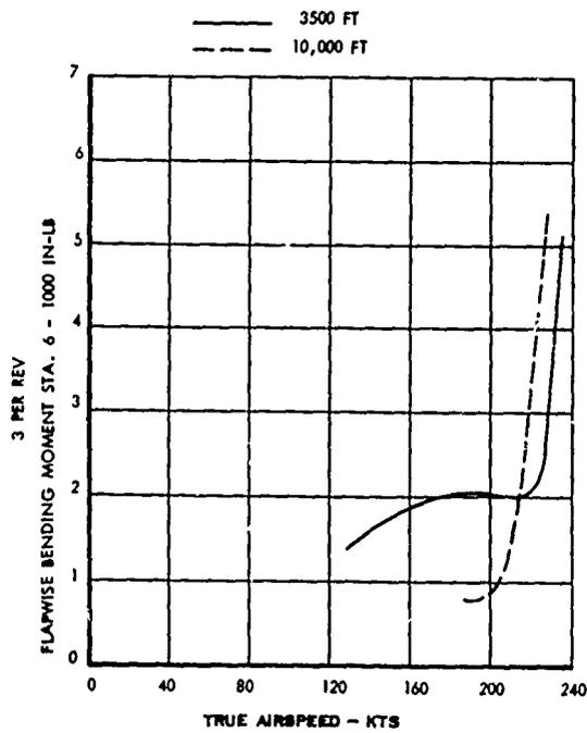
Figure 31. Flapwise Bending Moment Versus True Airspeed
