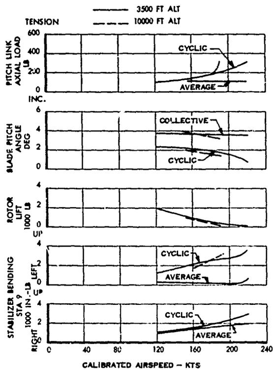
Figure 28. Main Rotor Loads Versus True Airspeed
