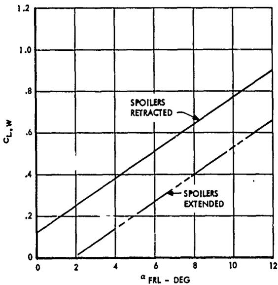
Figure 11. Wing-Body Lift Characteristics
