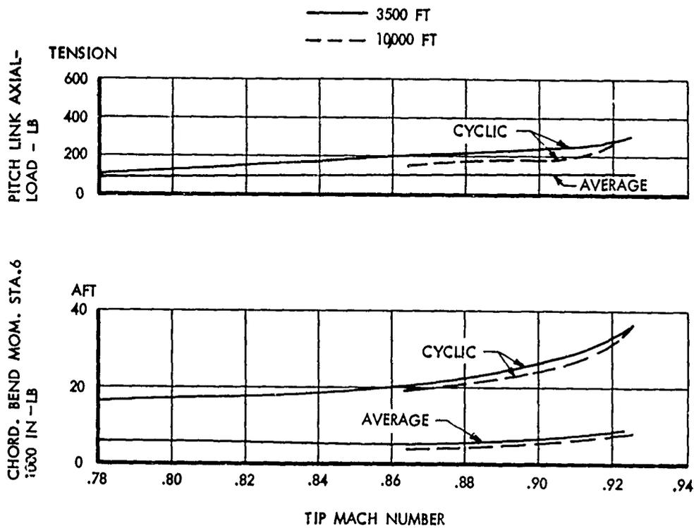
Figure 33. Rotor Loads Versus Tip Mach Number
