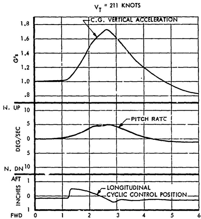
Figure 20. Time History of Longitudinal Control Power - 211 Knots
