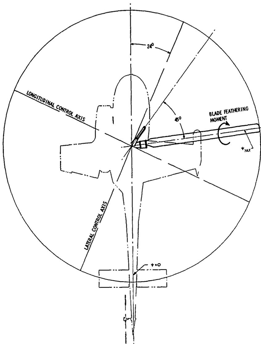
Figure 15. Phase Relationship Between Blade Feathering Moments and Control System
