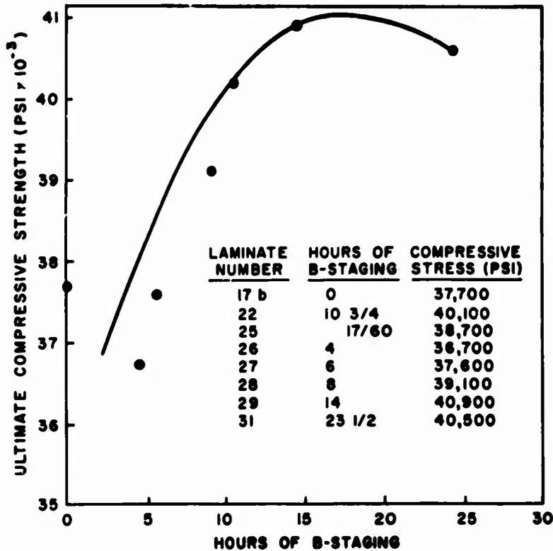
from pre-preg 2 was plotted for an estimate of the zero B-stage strength. The figure indicates that a trend does exist and that the previously used 10-hour B-staging is a good working value, in view of the data scatter and possible interactions with other fabrication variables. It should also be noted that B-staging increases the handling qualities of the pre-preg. Thus, the use of the 10-hour B-staged material was continued for the resin content study. Also, from the figure,
