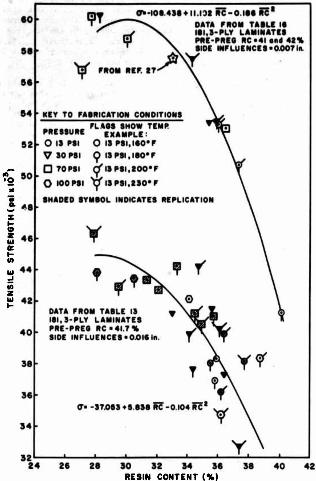
Figure 25. Tensile Strength Versus Resin Content. The lower curve indicates the effect of small stress concentrations.
