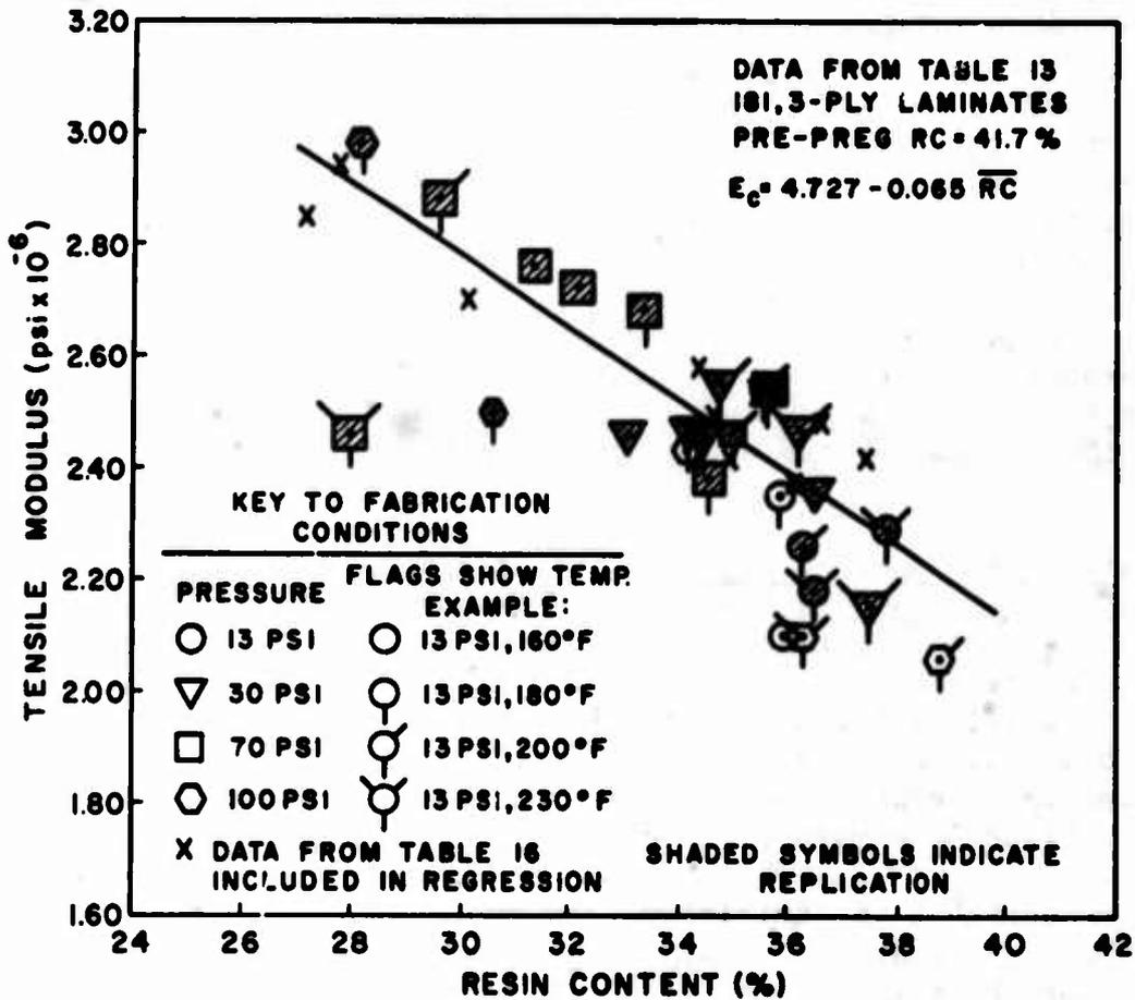
Figure 28. Tensile Modulus Versus Resin Content. The regression analysis is based on the total data shown.
