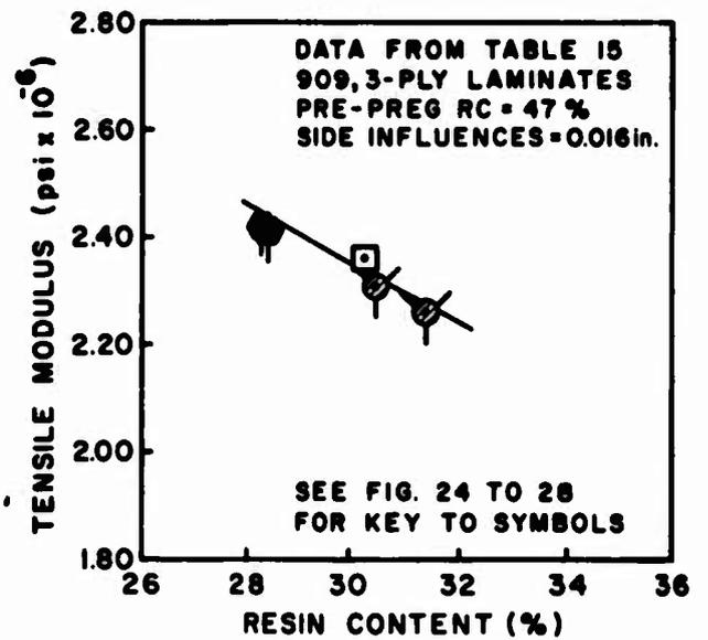
Figure 32. The Effect of Resin Content on Strength Properties of Laminates Reinforced With 909 Fabric, S-920 Finished.
