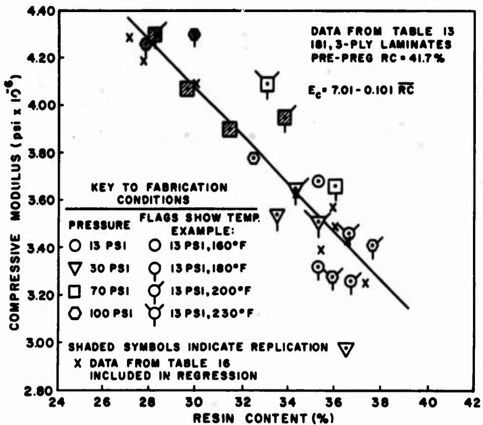
Figure 27. Compressive Modulus Versus Resin Content. The regression analysis is based on the total data shown.
