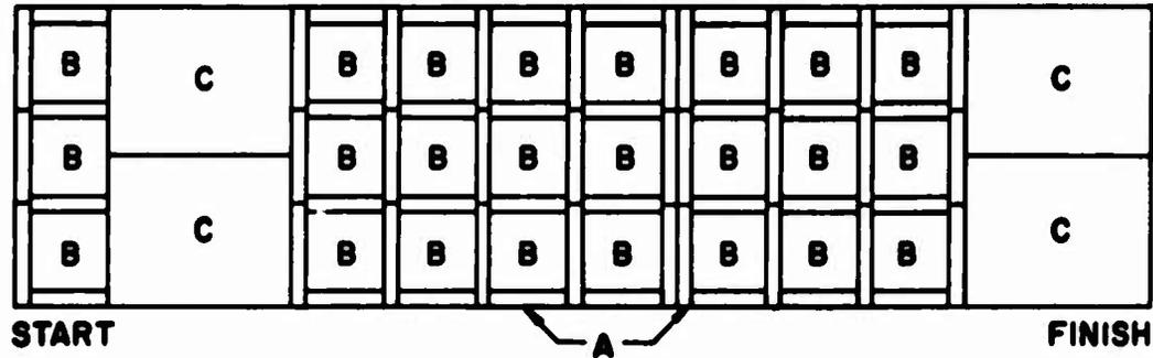
Figure 4. Typical Layout of Pre-Preg for a Resin Content Survey. A, 2-Inch-Wide Strips for Resin Content Sampling; B, 12-Inch-Square Specimens Used for Preliminary Fabrication Investigations; C, 22- by 28-Inch Specimens Used for Sandwich Facings.
