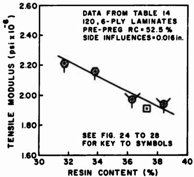
Figure 31. The Effect of Resin Content on Strength Properties of Laminates Reinforced With 120 Fabric, Volan A Finished.
