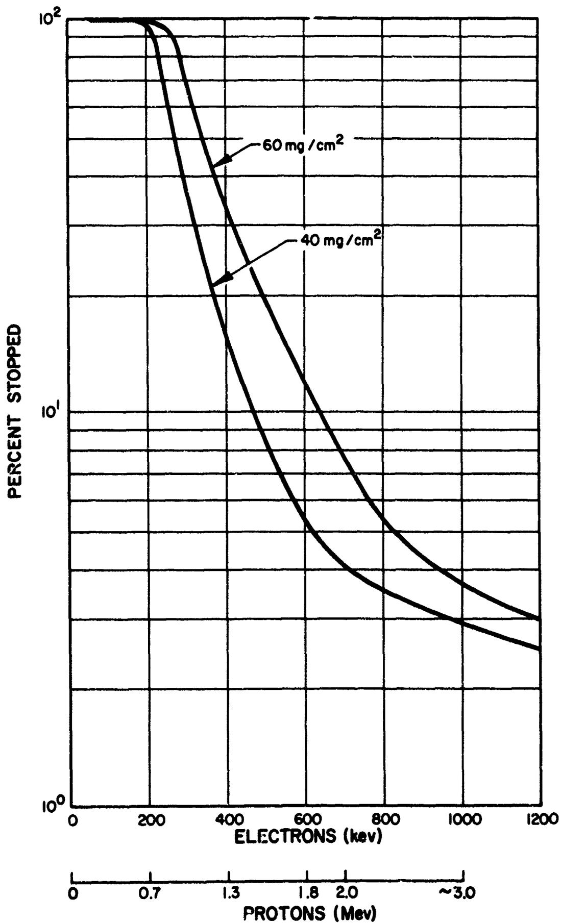
Fig. 15      Electrons Stopped in Aluminum
