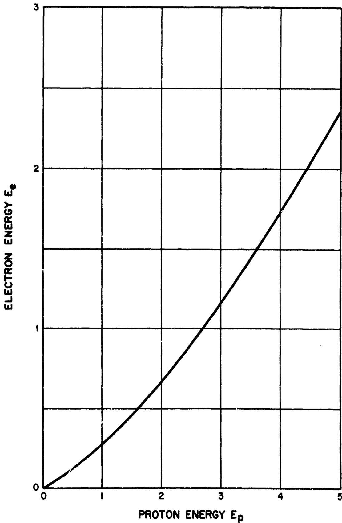
Fig. 16 Electron-Proton Scintillation Light Equivalents in Anthracene
