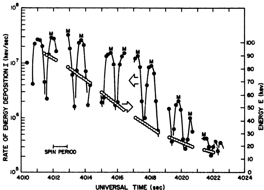
Fig. E1. Typical rate of energy deposition (kev/sec) in the electrostatic analyzer (filled circles) as a function of time. The points marked "M" are used to define a spectrum. Also shown (open circles) is the energy of the detected particles as a function of time.
