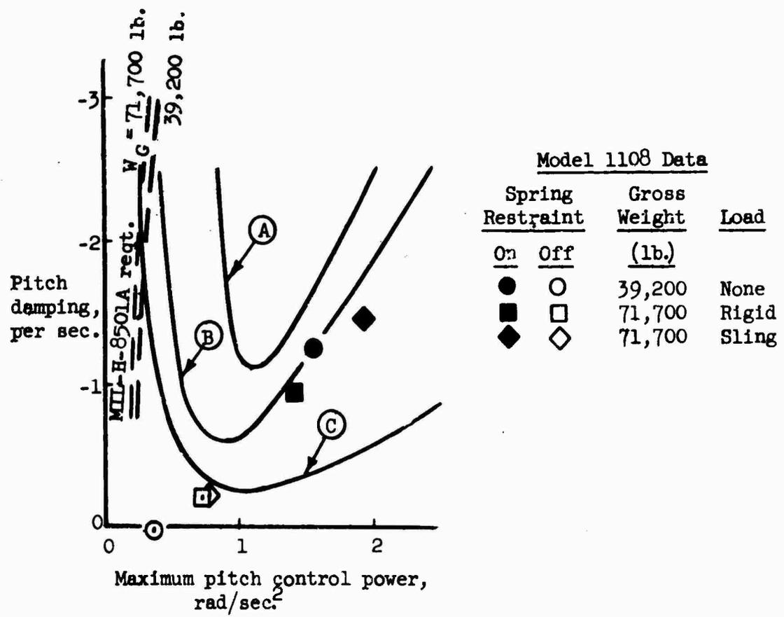
Figure 28. Maximum Control Power, Pitch Axis.
