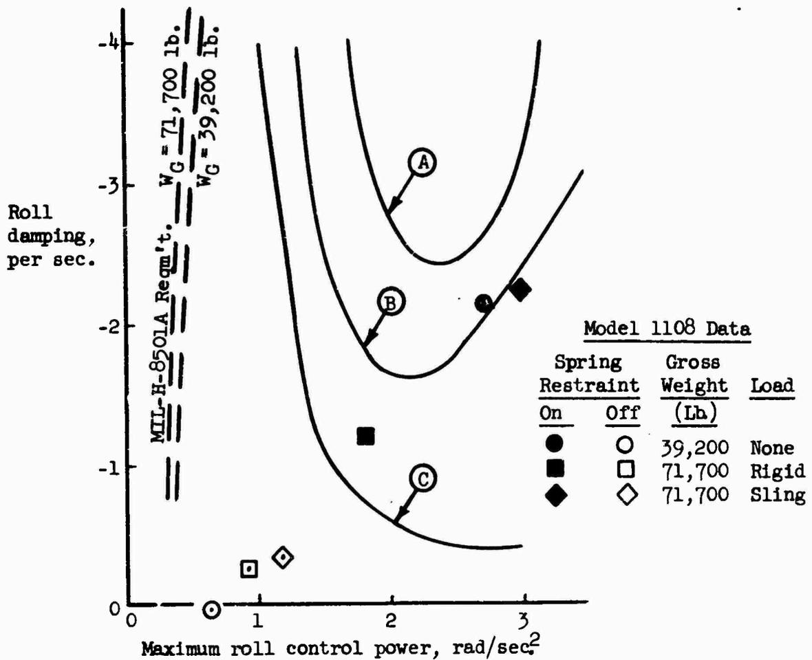
Figure 26. Maximum Control Power, Roll Axis.
