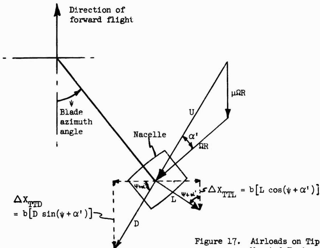
Figure 17. Airloads on Tip-Mounted Engine Nacelles.
