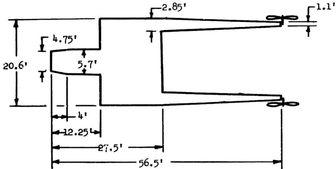
Figure 14. Planform Dimensions - Stability Analysis Model.
