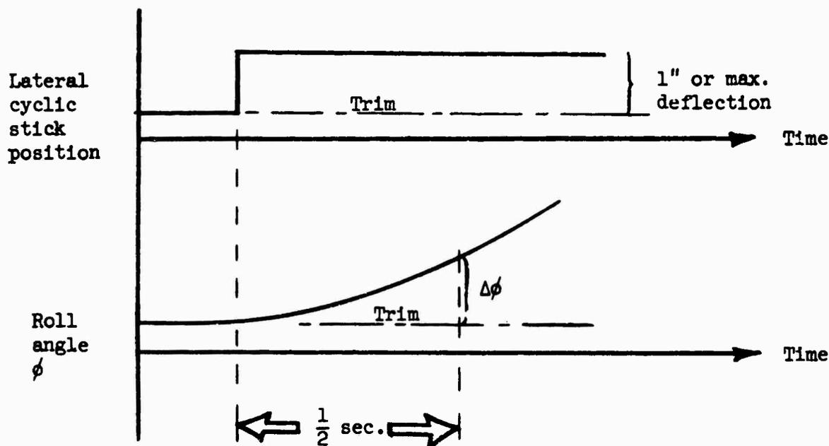
Figure 8. Lateral Control Input.
