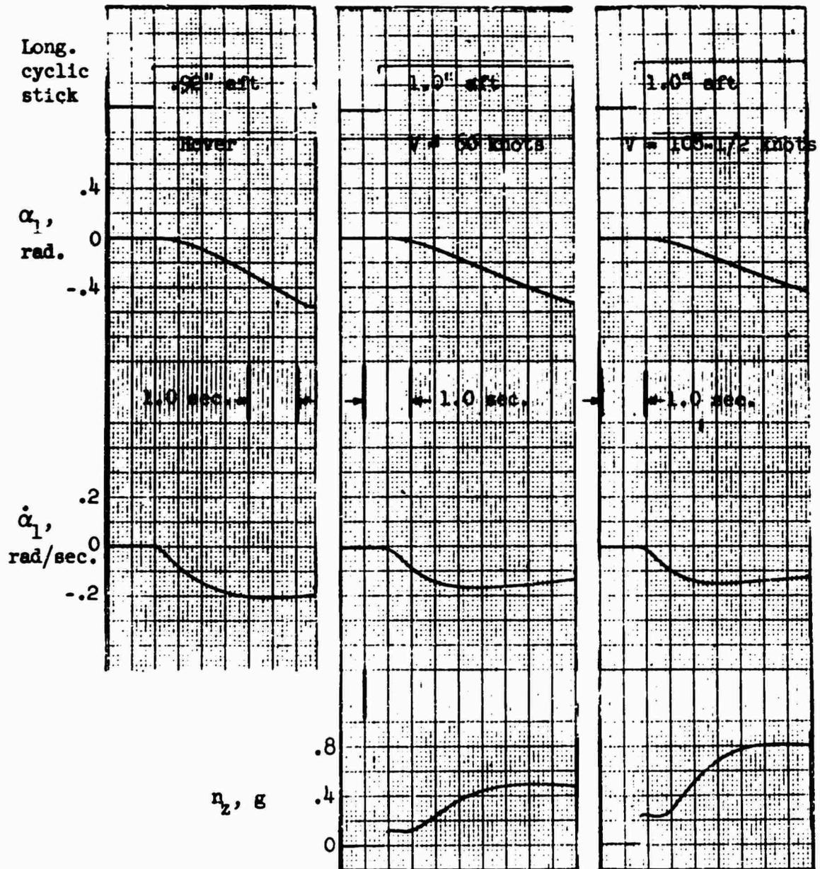
Figure 4. Longitudinal Maneuver Stability.
