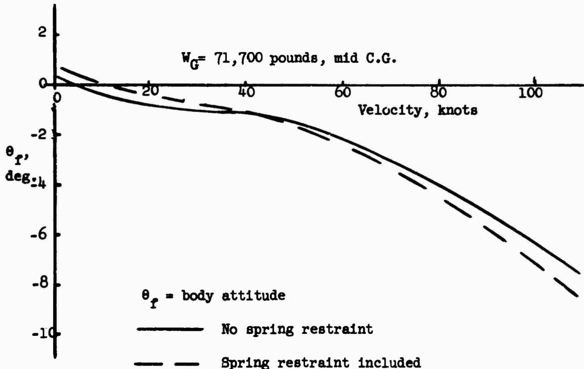
Figure 1. Effect of Spring Restraint on Trim Attitude.
