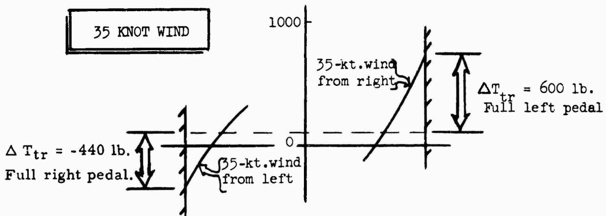
Figure 9. Tail Rotor Thrust for Control.
