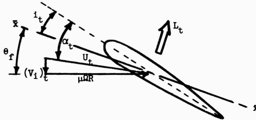
Figure 16. Angles and Forces on Horizontal Stabilizer.
