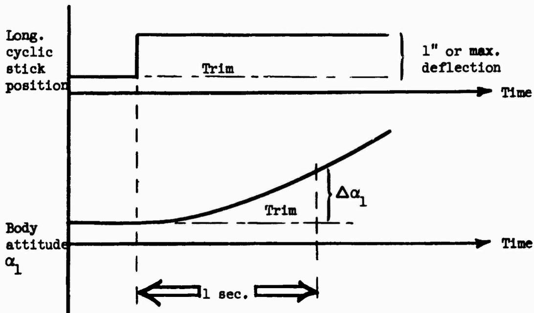
Figure 2. Longitudinal Control Response.
