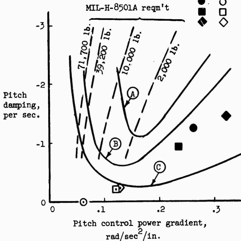
Figure 29. Control Power Gradient, Pitch Axis.
