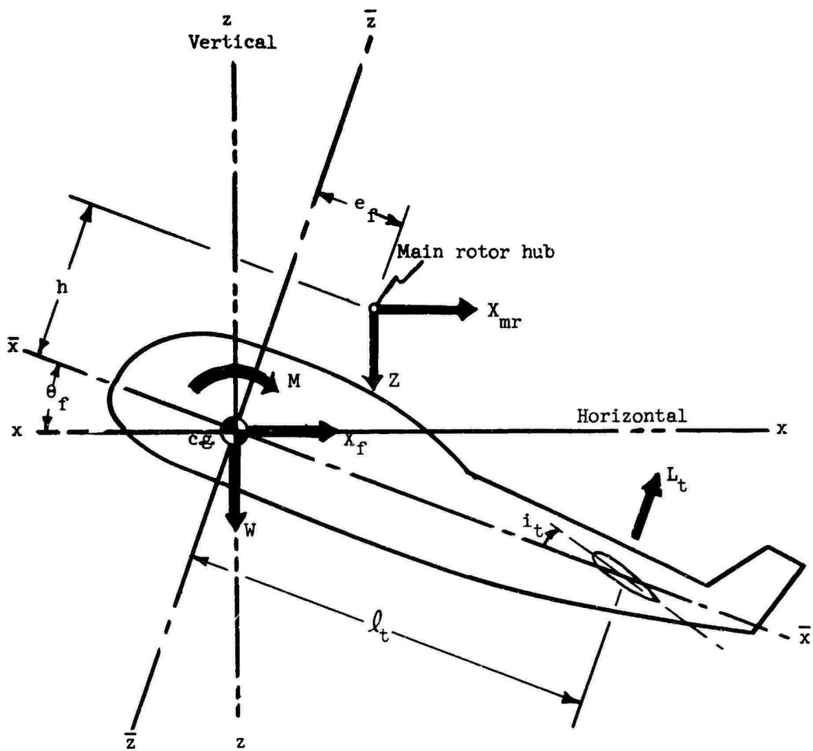
Figure 15. Forces and Moments for Trimmed Flight.
