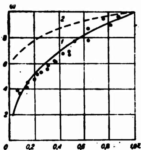
Fig. 26. Comparison of calculated velocity profile at the point of breakaway of the turbulent boundary layer with experimental data: 1) calculation by formula (5.11); 2) calculation according to the  $1/7$  power law;  $\circ$  — experiments of I. Nikuradze;  $\bullet$  — experiments of A. I. Leont'ev, A. N. Oblivin, P. N. Romanenko.
