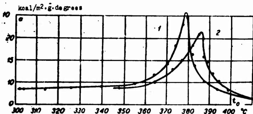
Fig. 50. Change of coefficient of heat transfer during flow of water and steam in the region of critical parameters from the experiments of A. A. Armand et al.: 1 -  $P = 240$  atm; 2 -  $P = 260$  atm;  $q = 1.7 \cdot 10^5$  kcal/m<sup>2</sup> · hr;  $\gamma_w = 650$  kg/m<sup>2</sup> · sec.
