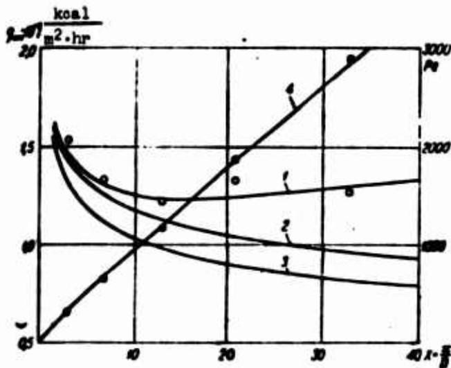
Fig. II.3. Results of calculation of heat transfer in the inlet section of the pipe: 1 -  $q_{wall}$  according to the method of the authors 2 -  $q_{wall}$  according to the method of B. S. Petukhov, 3 -  $q_{wall}$  by the empirical criterial formula for stabilized heat transfer in a pipe, 4 -  $Pe$  according to the method of the authors,  $\circ$  - experimental data of B. S. Petukhov for  $q_{wall}$ ;  $\otimes$  - experimental data of B. S. Petukhov for  $Pe^{**}$ .
