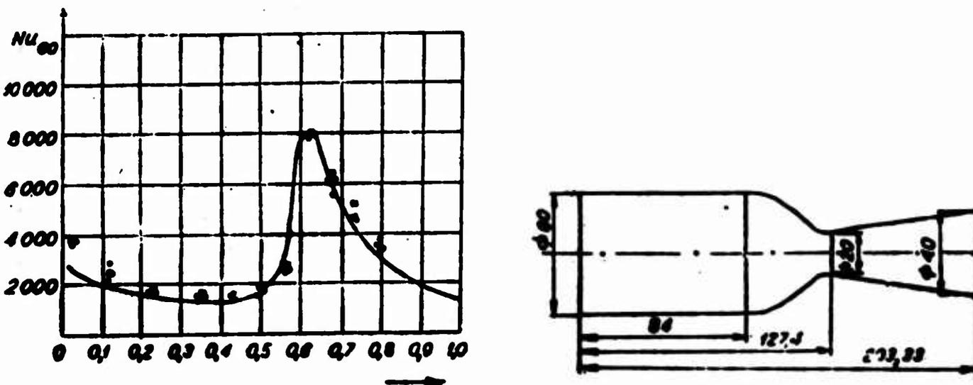
Fig. 41. Comparison of calculations of heat transfer in a supersonic nozzle by formula (5.82) with the experimental data of A. I. Leont'ev.
