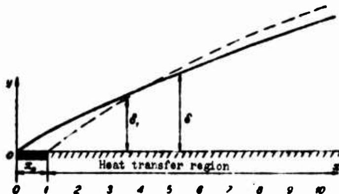
Fig. 9. Plate with initial heat-insulated section ( $Pr = 0.72$ ).
