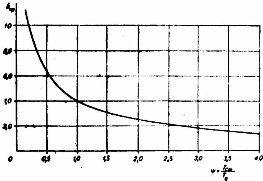
Fig. 17. Influence of heat transfer on the parameter of breakaway  $b_{cr}$  for a uniform boundary layer. — calculation by equation (4.28) for the case  $\psi < 1$  and by equation (4.29) for the case  $\psi > 1$ .
