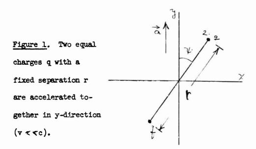
specified acceleration by using the solution to Maxwell's equations which applies throughout the region external to a source charge q whose state of motion is given. For the case where v << c, a source charge, q, produces an electric field,  $\vec{E}$ , at the field point, P, located a distance,  $\vec{F}$ , from the charge,
