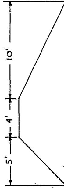
Fig. 4. Operation SNOWBALL: Dimensions of the earthen berm.
