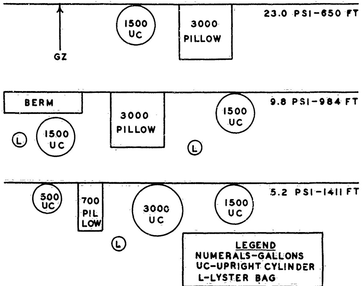
Fig. 3. Tank layout at three overpressure sites.
