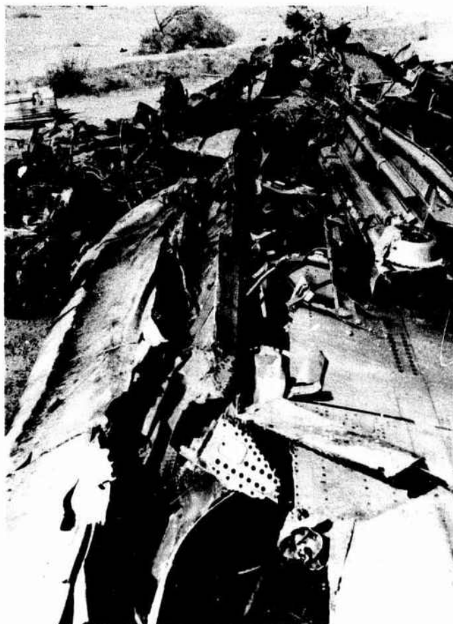
FIG. 34 CLOSEUP VIEW OF FRONT OF LEFT MID-WING AREA (ALTERNATE TANK NO. 1) WHERE GELLED FUEL WAS CARRIED
