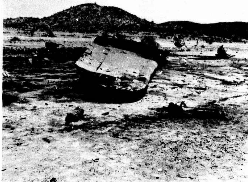
FIG. 32 POSTCRASH VIEW OF LEFT WING WHERE IT CAME TO REST LYING 50 FEET AHEAD OF MAJOR AIRCRAFT WRECKAGE
