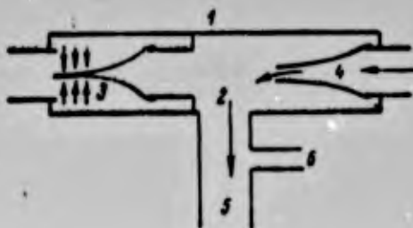
Fig. 2. Diagram of inhalation-exhalation leaf valves. 1) Valve housing; 2) intervalve space; 3) rubber leaves of exhalation valve; 4) rubber leaves of inhalation valve; 5) tube communicating with respiratory passages; 6) tube communicating with manometer which records the pressure in the intervalve space.
