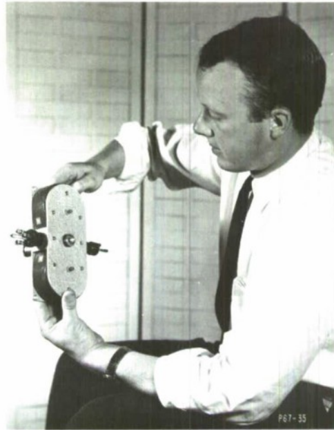
Fig. 17. Floating-drift-tube klystron oscillator used as the power tube for the 8-mm radar. V.L. Lynn, Project Engineer, is shown holding the millimeter wave power tube.
