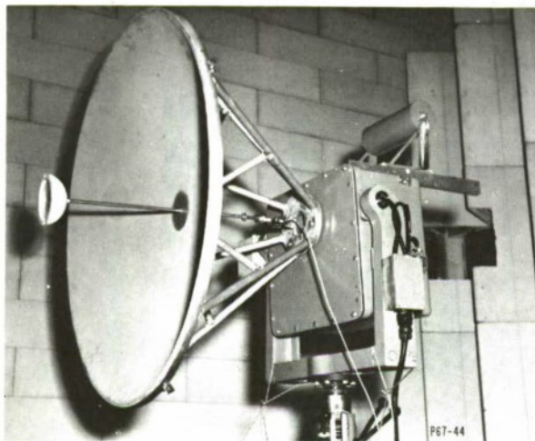
Fig. 15. The Keeping feed installed in a four-foot spun-cast parabola. The unit served as a transmitter for the pattern range employed in the evaluation of the 28-foot parabola.
