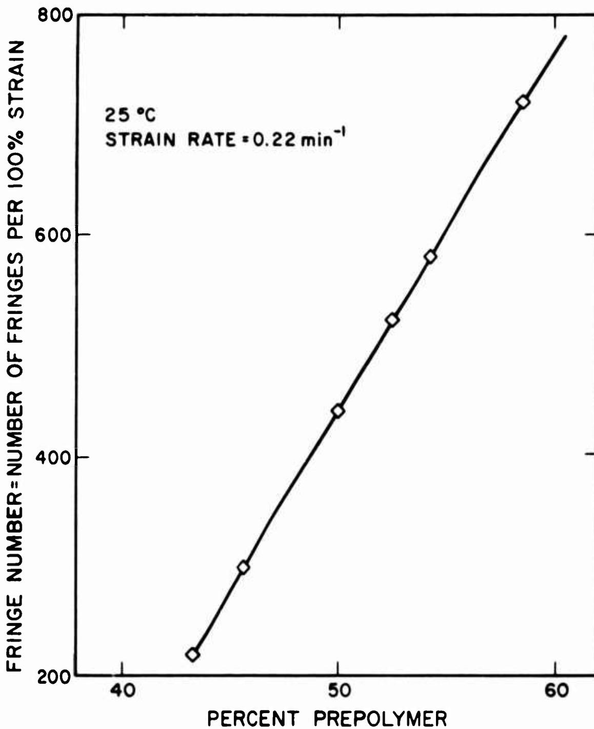
Figure 9. Strain-Optic Coefficient as a Function of Prepolymer-Catalyst Composition at 20°C.
