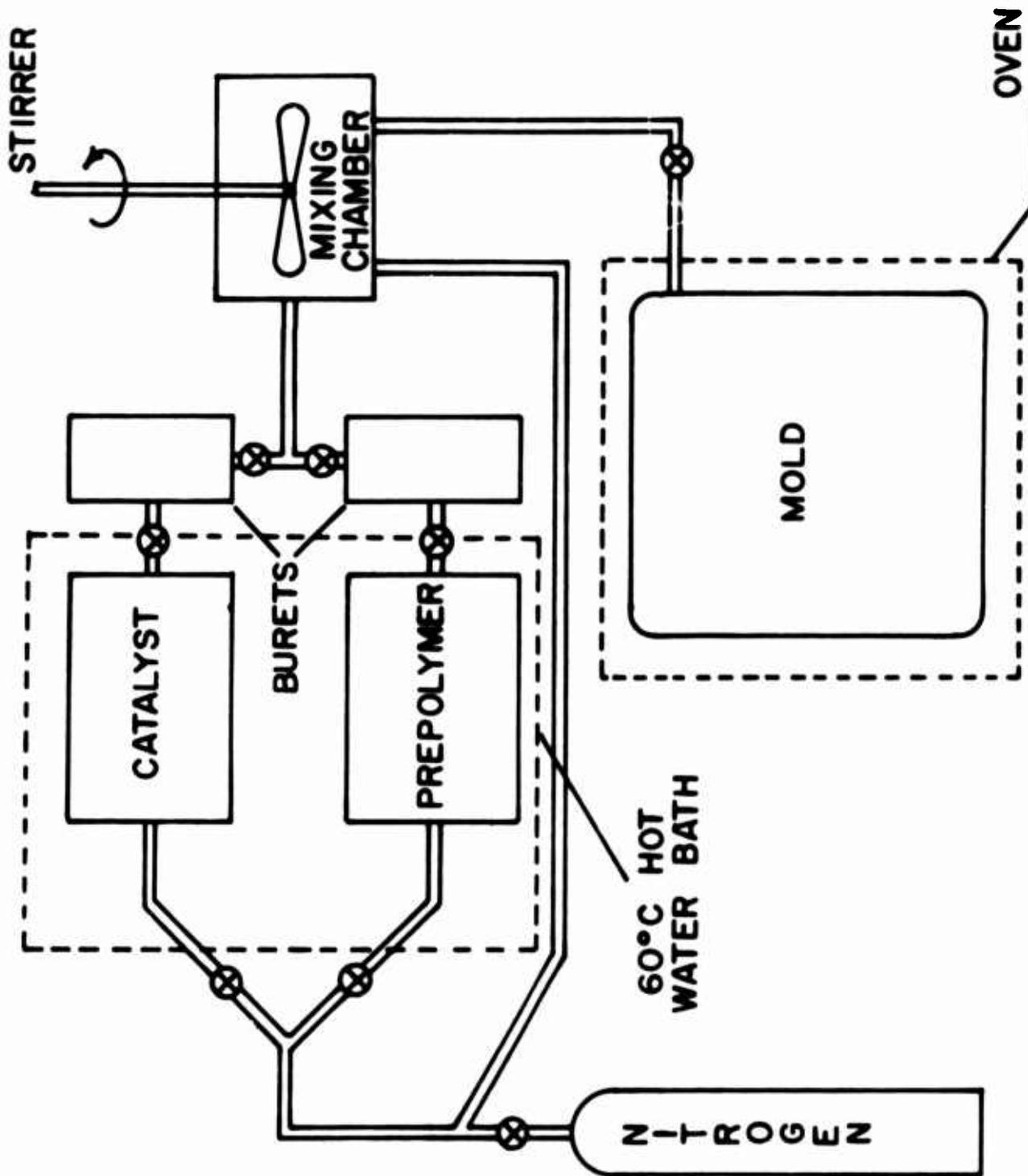
Figure 3. Schematic of Solithane 113 Production Facility.
