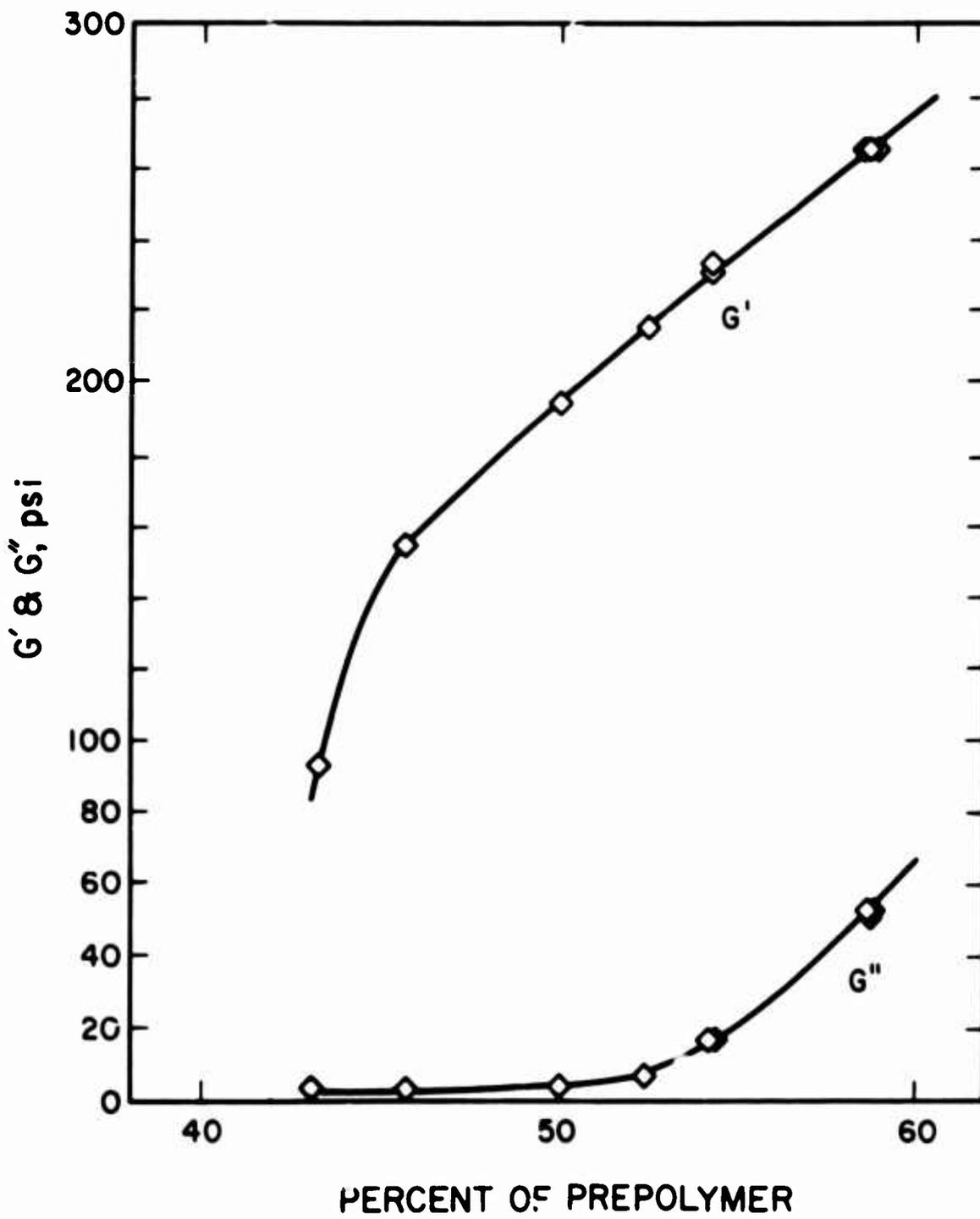
Figure 5. Complex Modulus at 20°C as a Function of Prepolymer-Catalyst Composition.
