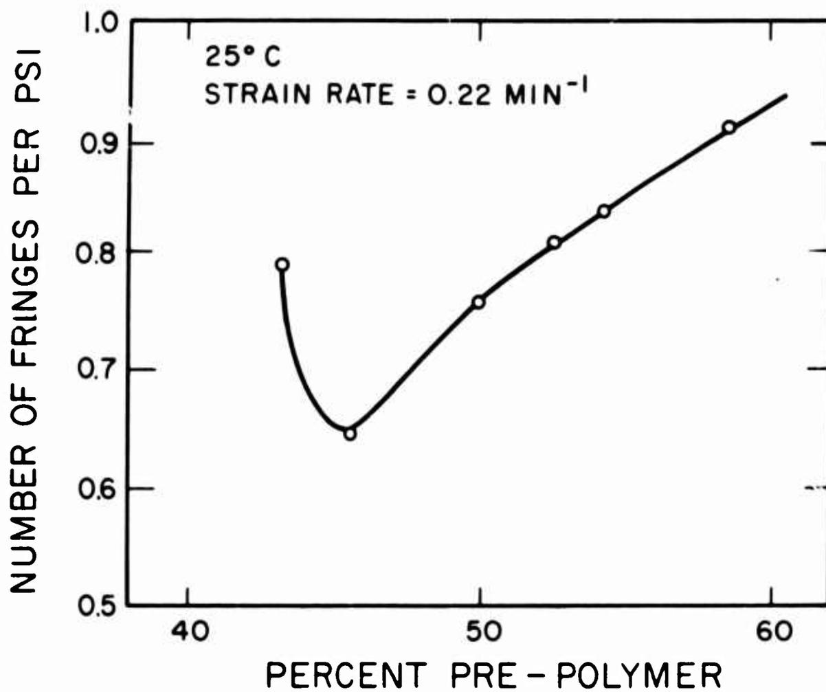
Figure 10. Stress-Optic Coefficient as a Function of Prepolymer-Catalyst Composition at 20°C.
