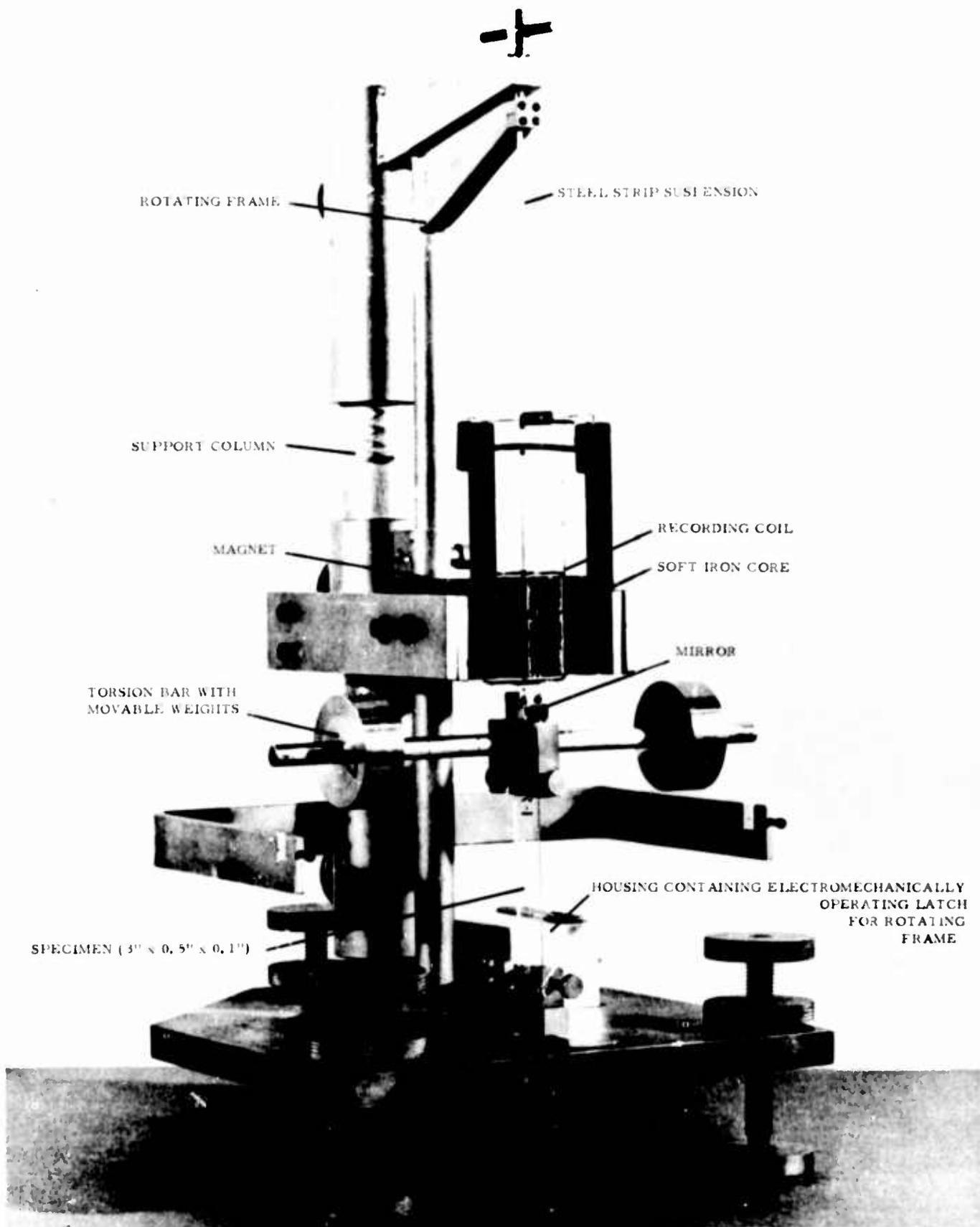
Figure 17. Free Oscillation Torsion Pendulum.
