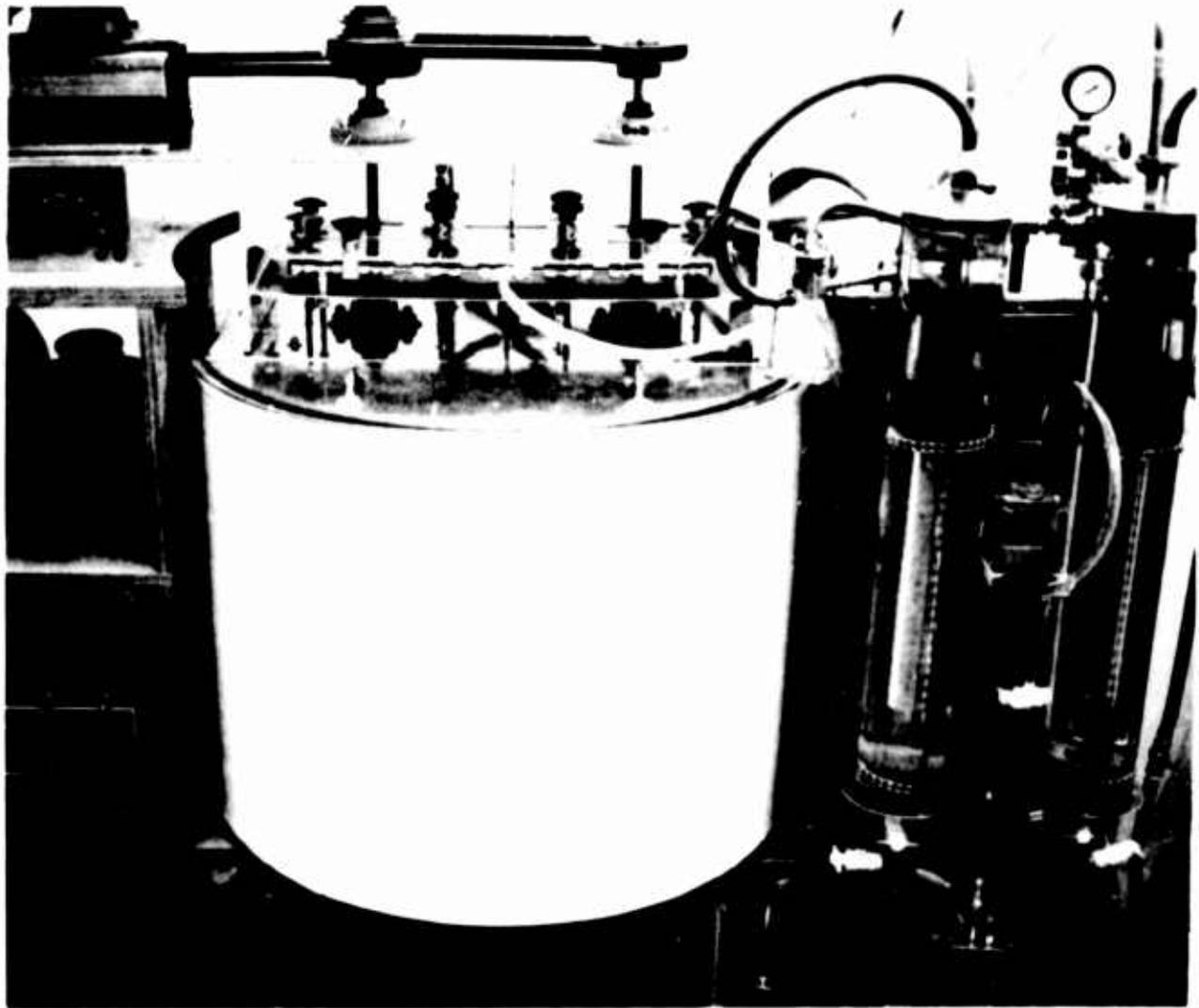
Figure 2. Solithane 113 Casting Facility
