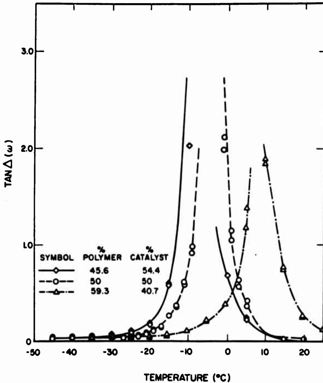
Figure 8. Loss-Tangent as a Function of Prepolymer-Catalyst Composition and Temperature.
