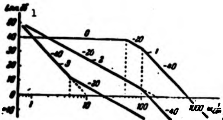
Fig. 17. Logarithmic amplitude characteristic for Problem 18. 1) db; 2) sec.
