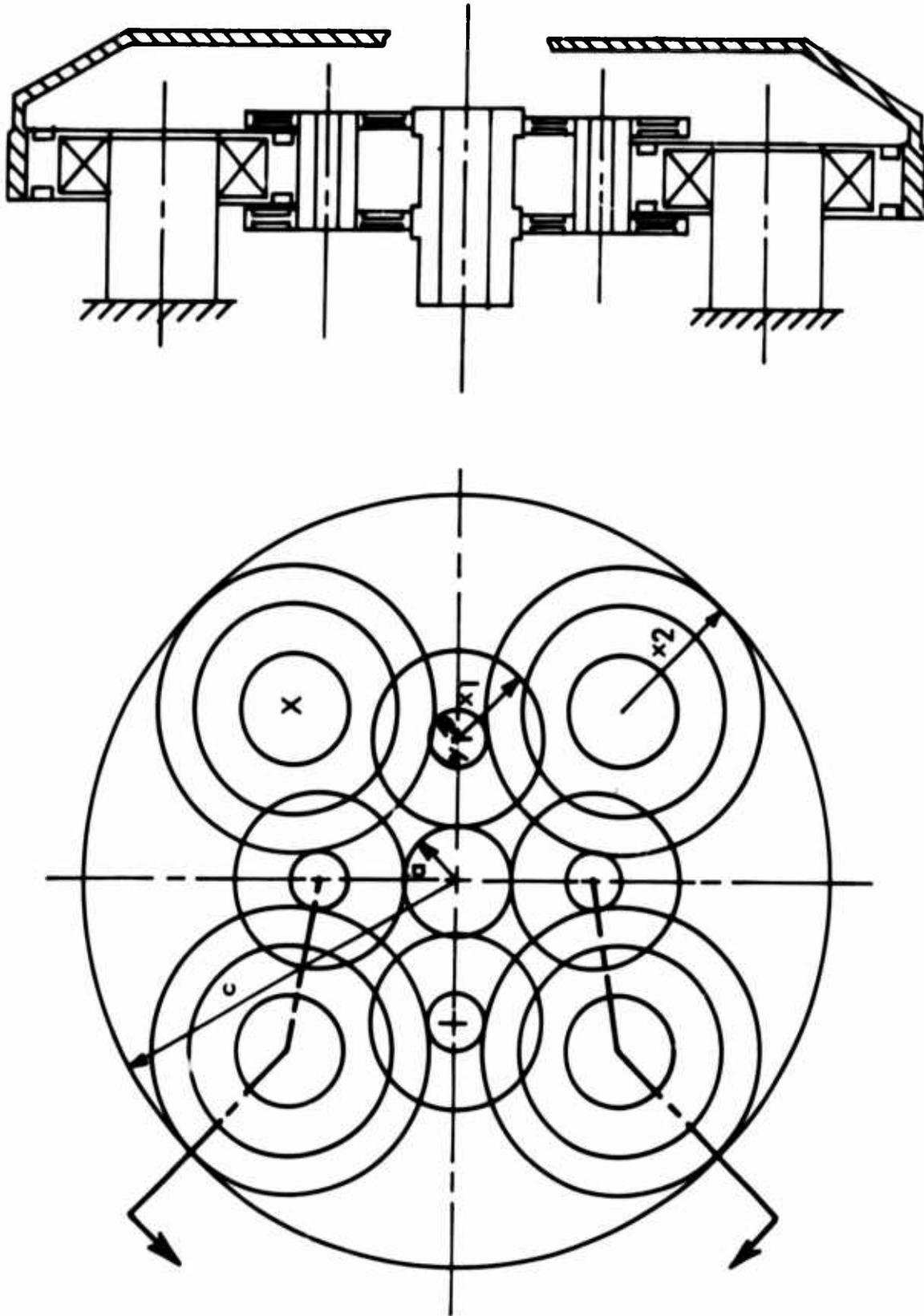
Figure 44. Small Sun Gear Drive; 20:1 Ratio, 21,000-rpm Input Speed, 4-4 Drive.
