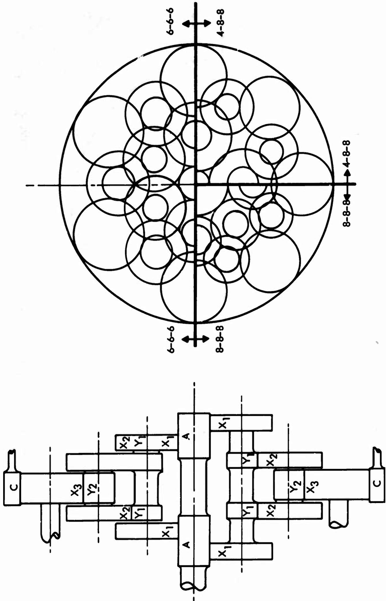
Figure 28. Roller Gear Cluster, Three Row Configuration, Double Staggering ( $X_1 - X_1$  and  $X_3$ ).
