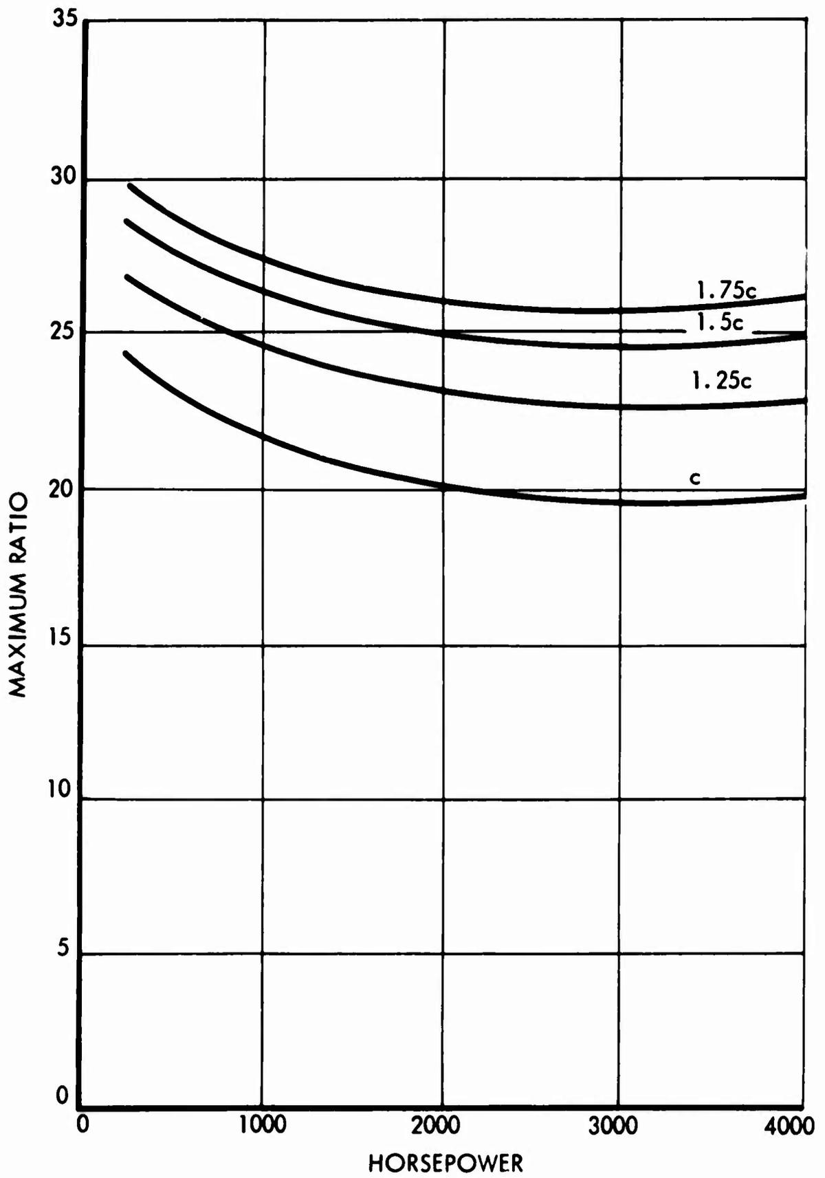
Figure 17. Maximum Ratio Versus Horsepower Curves (8-8 Drive), Staggered X<sub>1</sub>.
