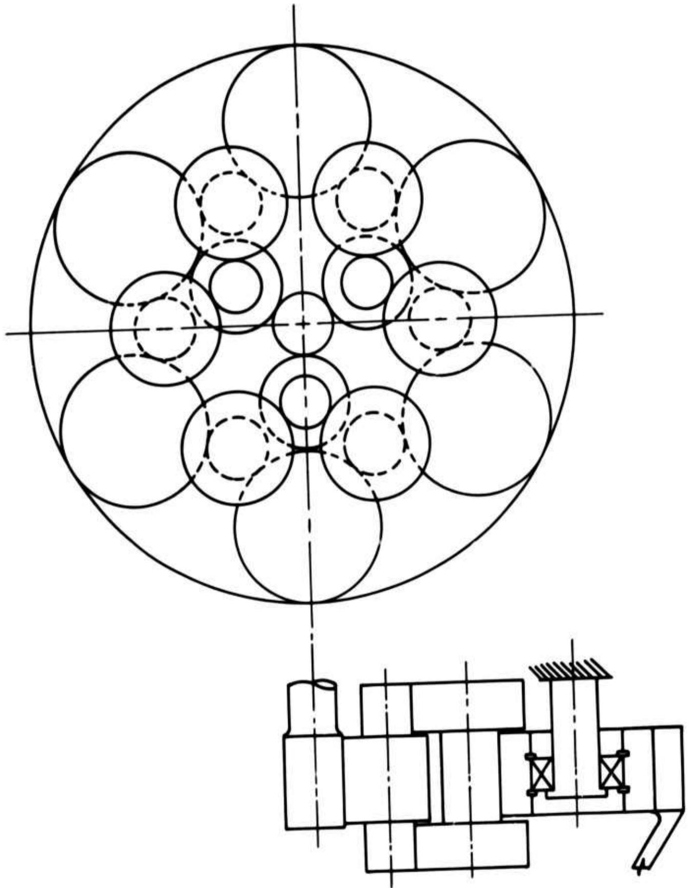
Figure 6. NUOS Roller Friction Drive Schematic.
