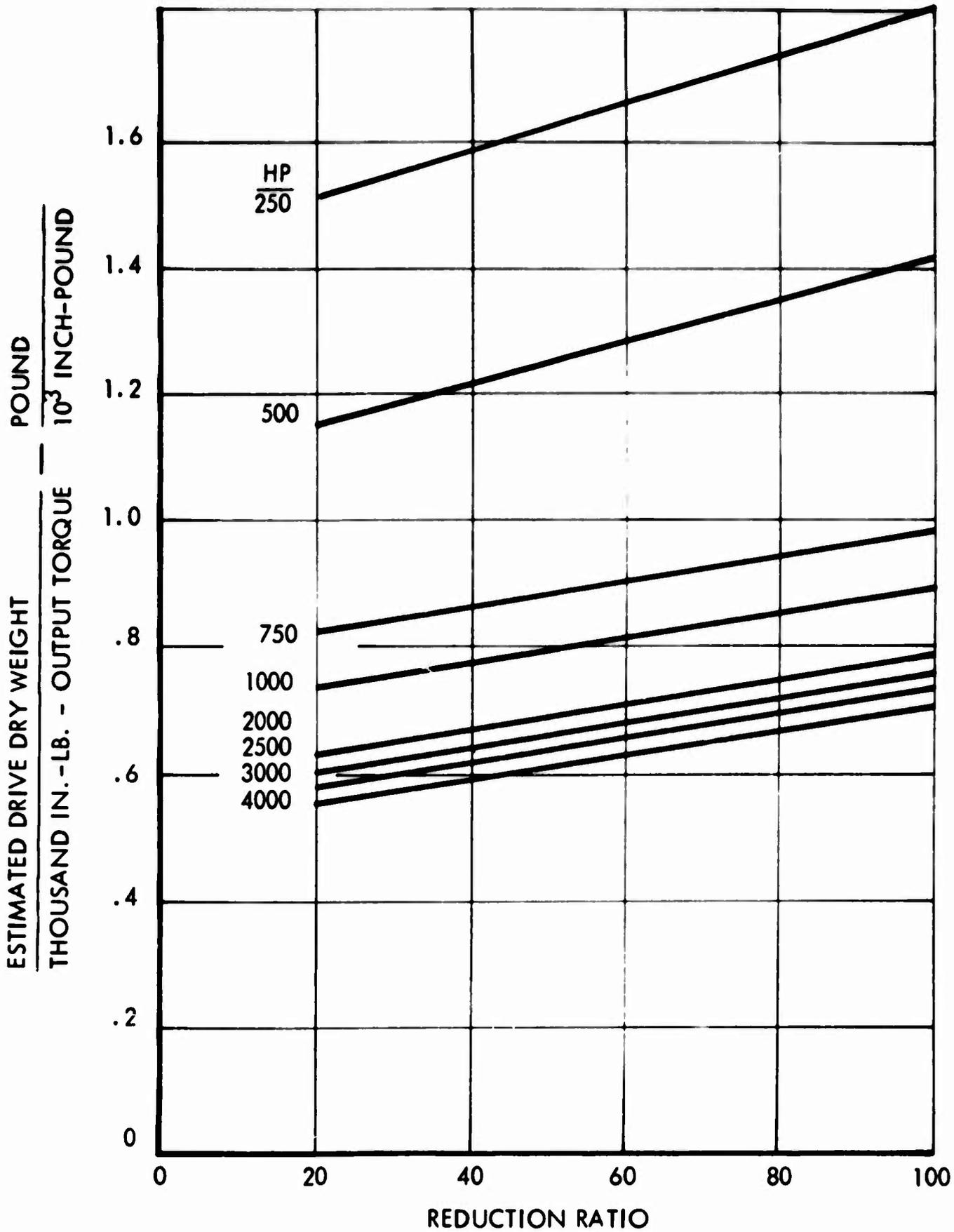
Figure 37. Estimated Drive Weight per Thousand Inch-Pound Output Torque Versus Reduction Ratio-Rotor Output rpm
