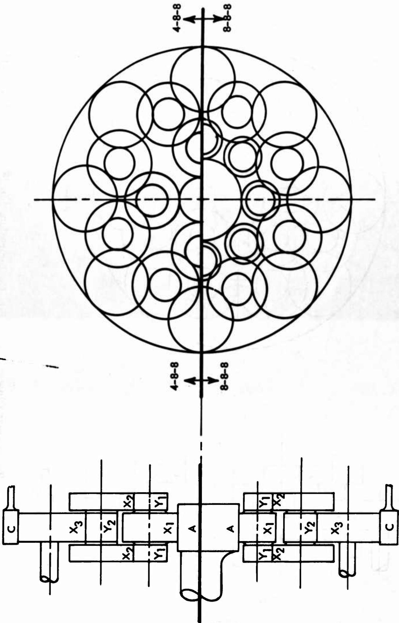
Figure 25. Roller Gear Cluster, Three Row Configuration, Nonstaggering.
