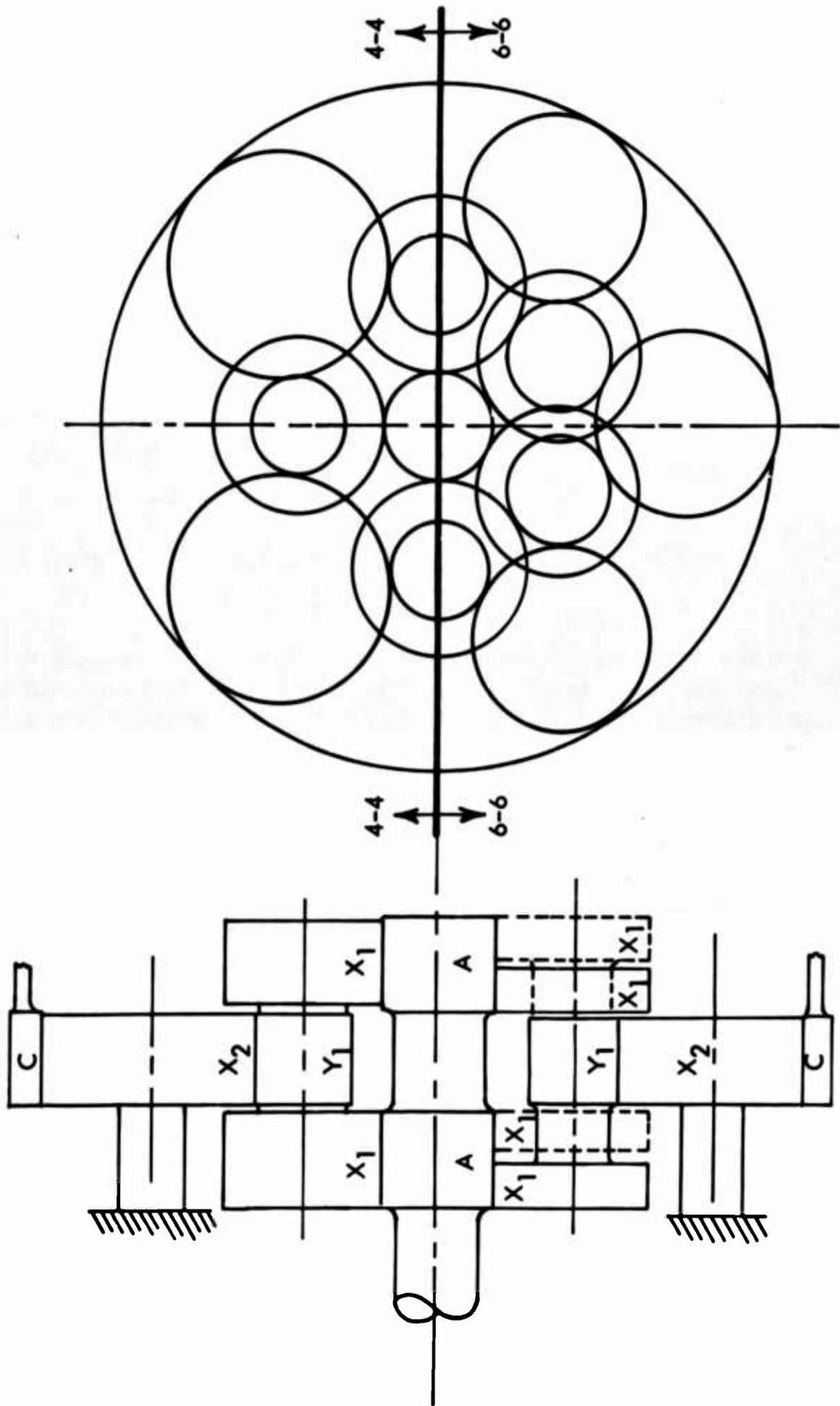
Figure 24. Roller Gear Cluster, Two Row Configuration
