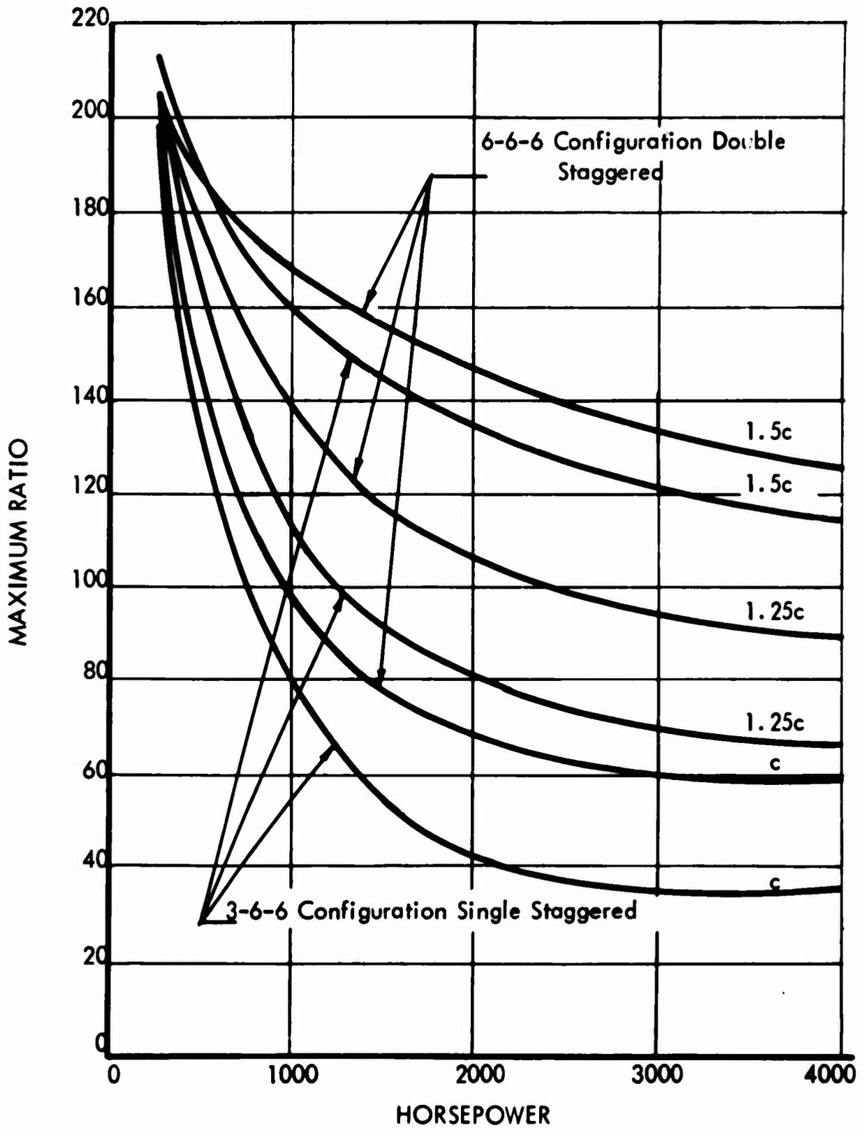
Figure 18. Maximum Ratio Versus Horsepower Curves (3-6-6 and 6-6-6 Drive).
