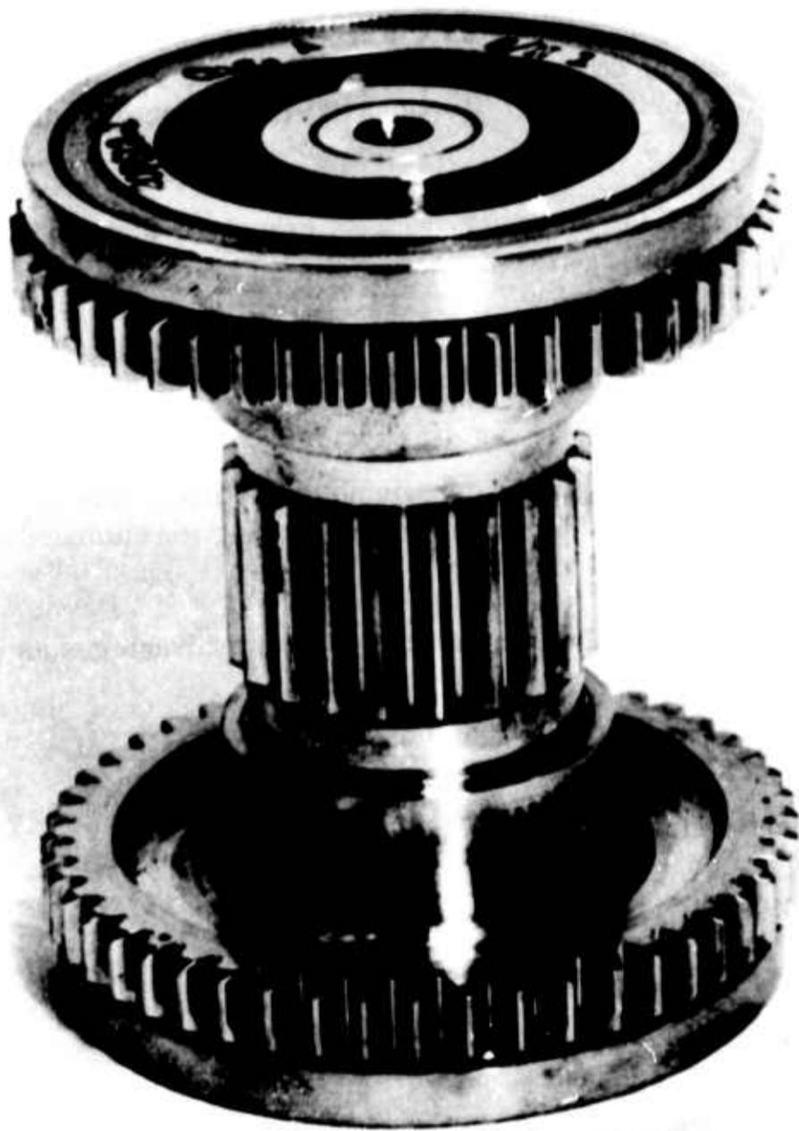
**Figure 7. Roller Gear Stepped Planet.**
