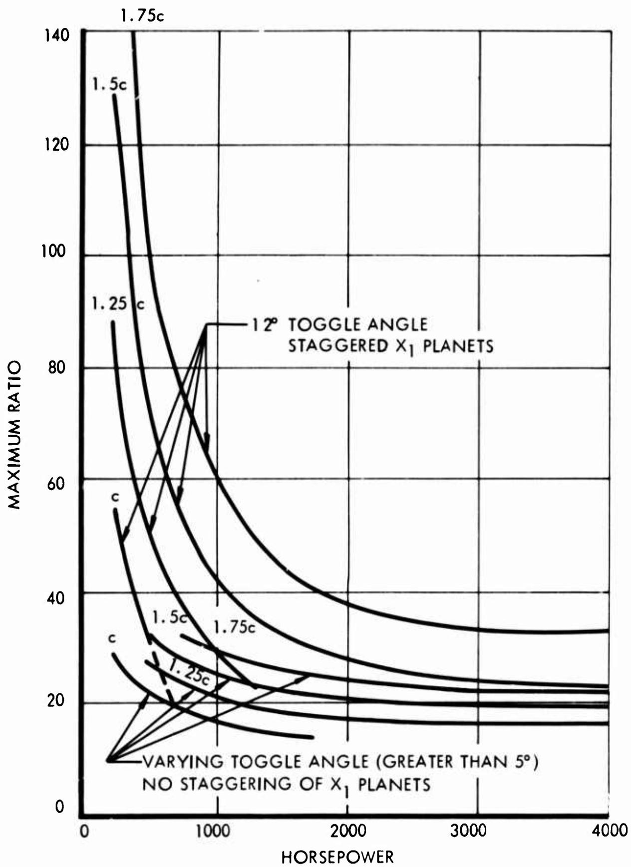
Figure 15. Maximum Ratio Versus Horsepower Curves (4-4 Drive).
