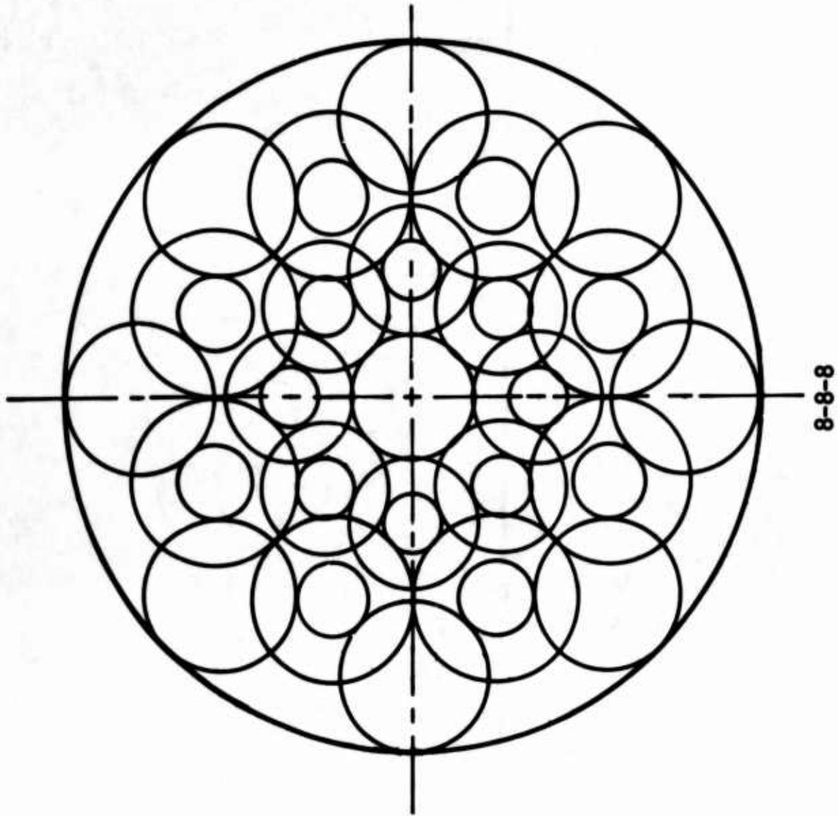
Figure 26. Roller Gear Cluster, Three Row Configuration, Single Staggered ( $X_1 - X_1$ ).
