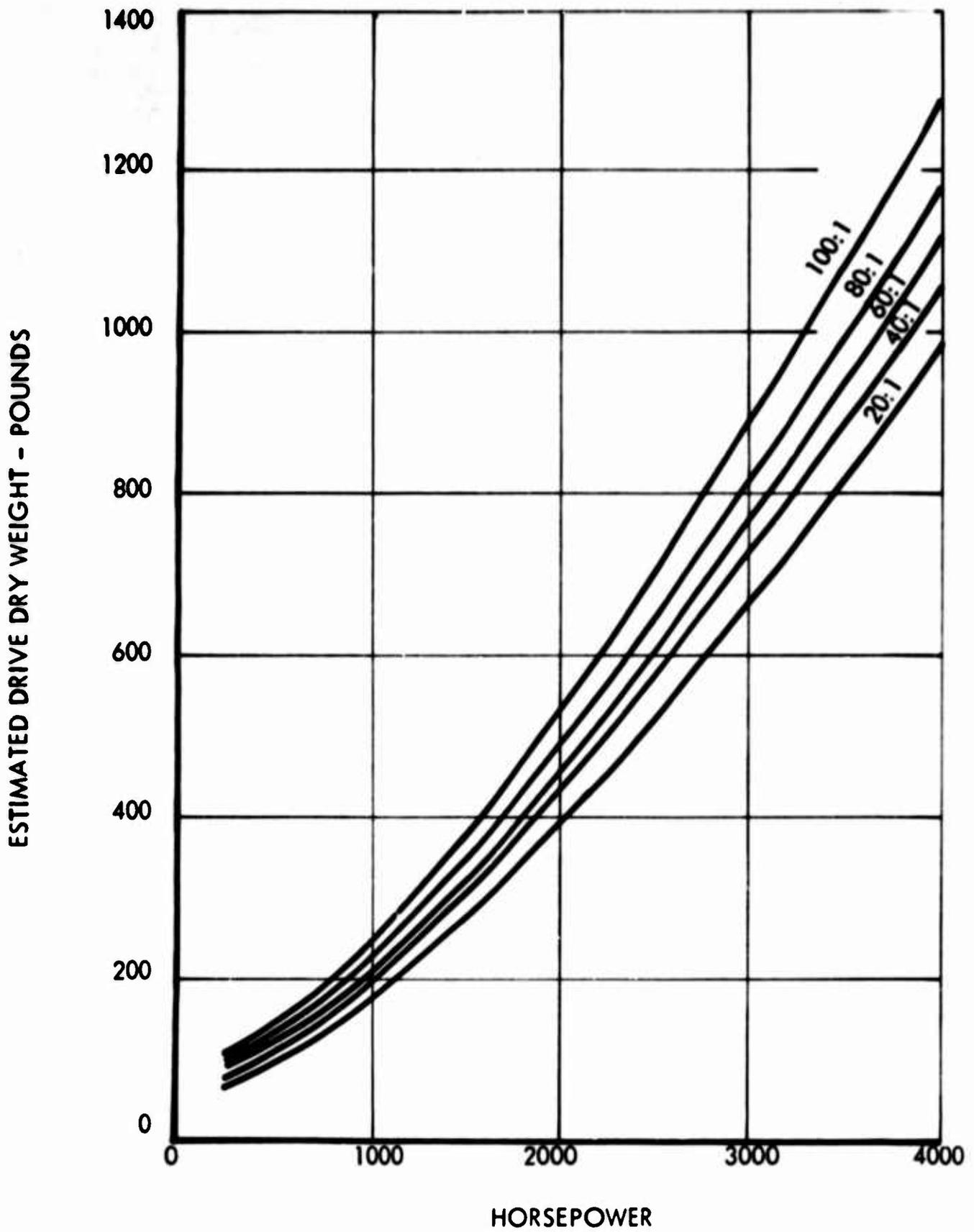
Figure 34. Estimated Drive Dry Weight Versus Horsepower for Constant Ratios - Rotor Output rpm
