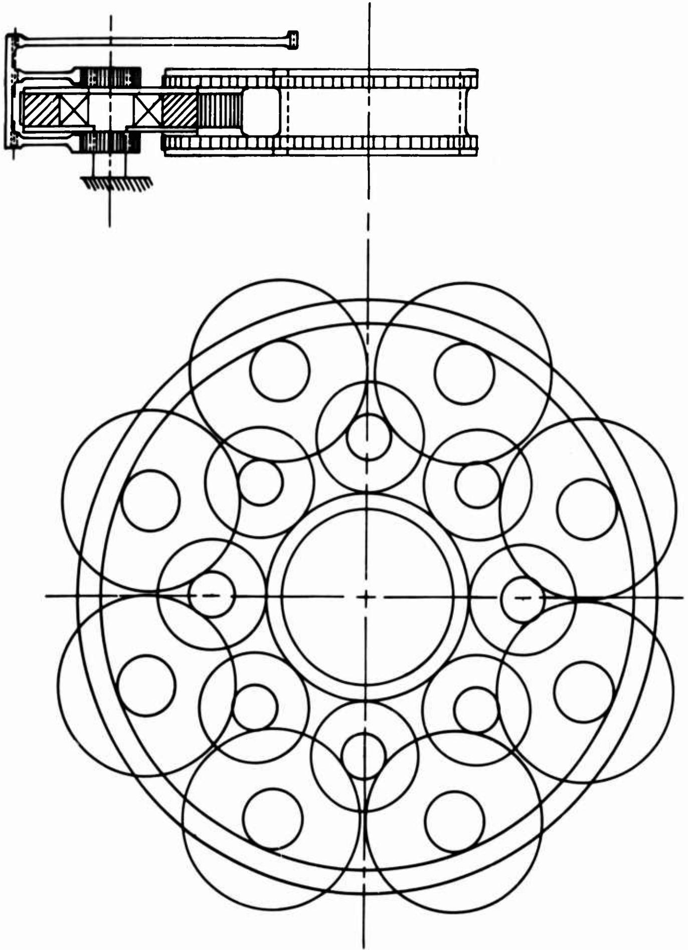
Figure 45. Enlarged Sun Gear Drive; 1000 Horsepower, 20:1 Ratio, 21,000-rpm Input Speed, 8-8 Drive.
