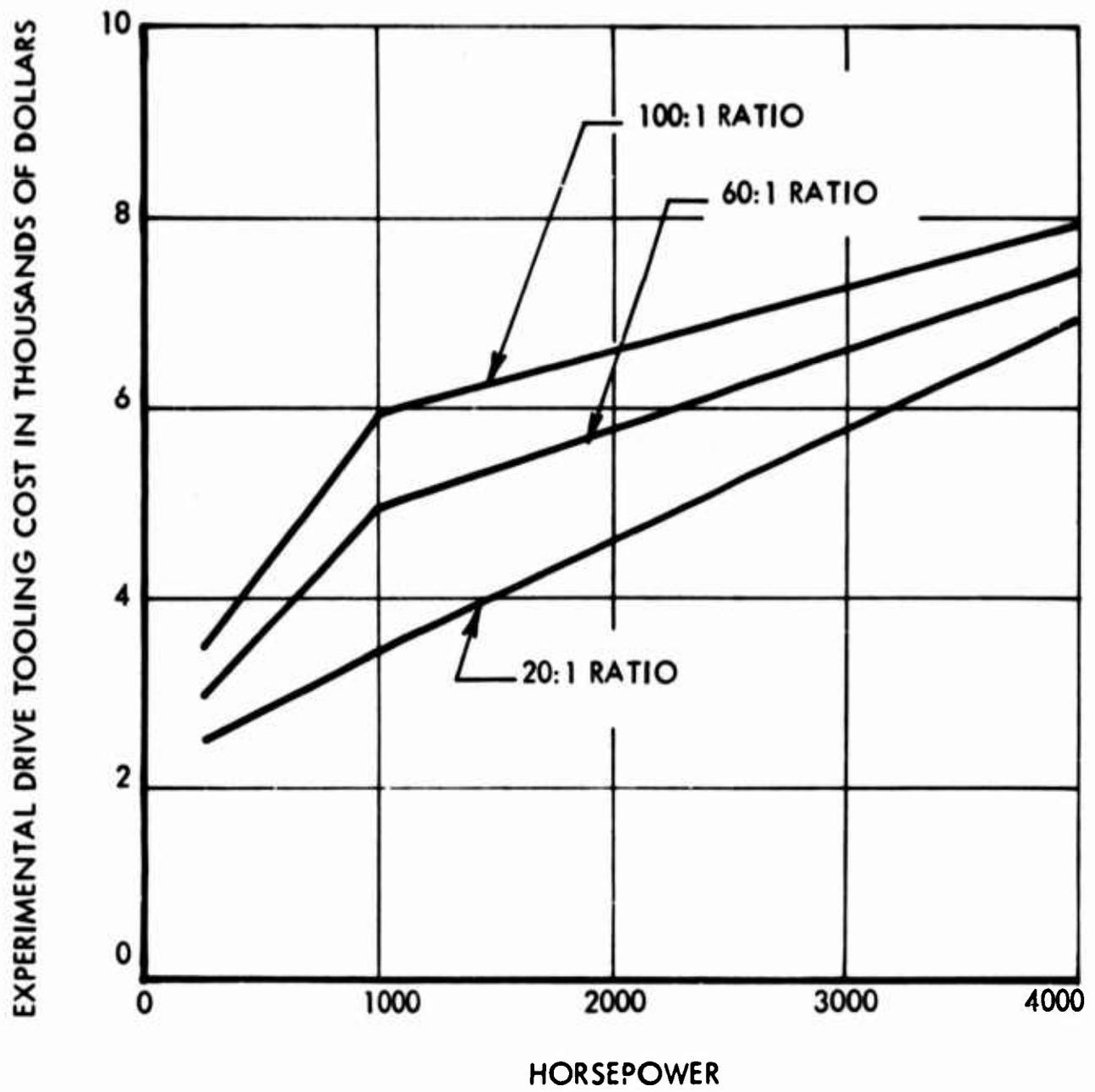
Figure 41. Estimated Experimental Roller Gear Drive Tooling Costs.
