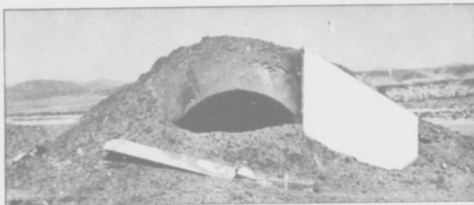
FIG. 25. Acceptor Igloos After Test.
