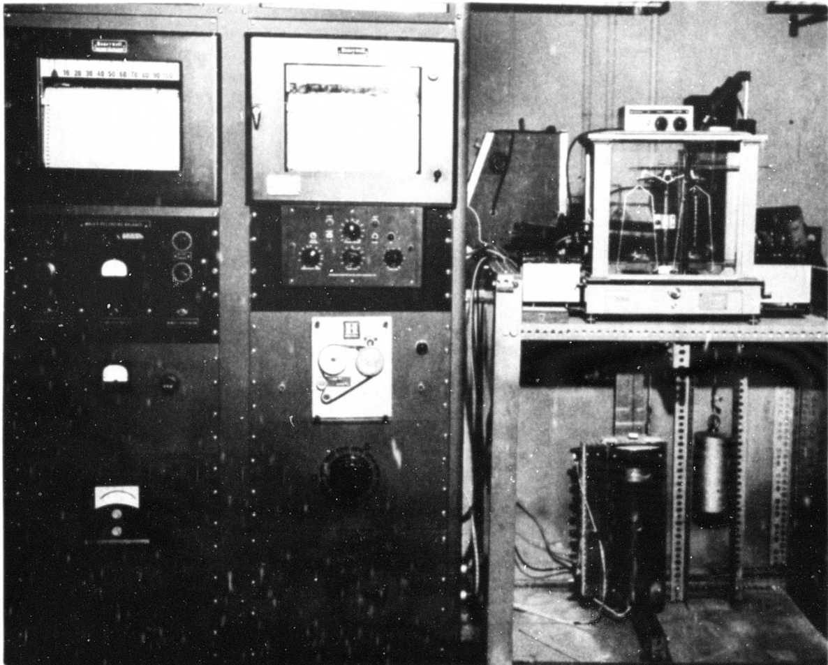
Figure 3. CONTINUOUS WEIGHING AND RECORDING OXIDATION APPARATUS
