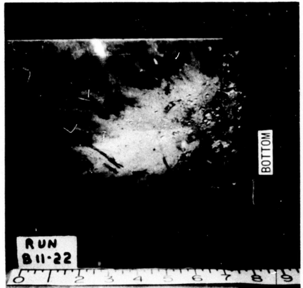
Figure 3 Run 22, 3/16 Inch Diameter Solid Copper Sphere, Oblique Impact at 13,570 Feet/Sec.
