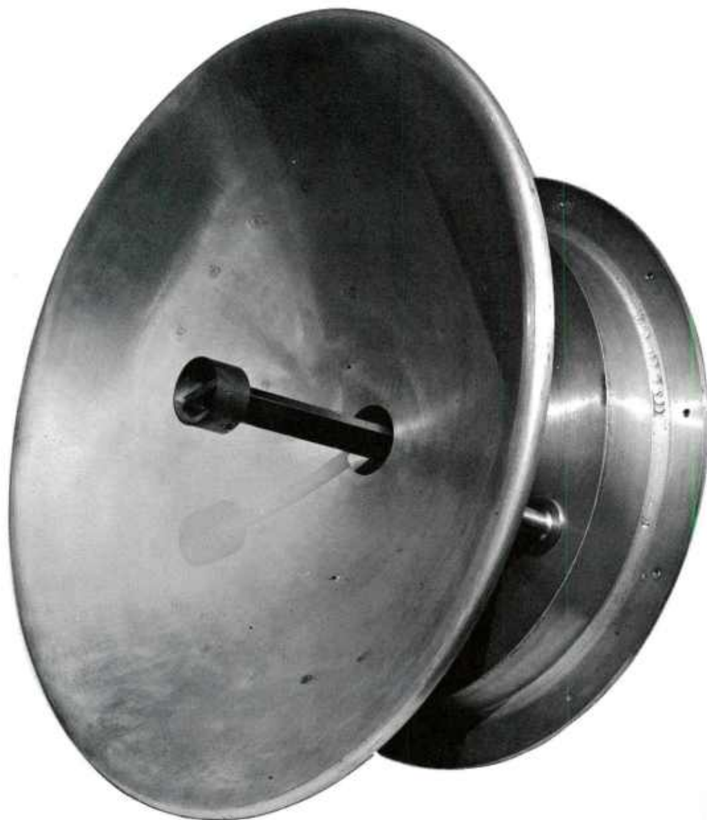
Fig. 18. 5.0 Gcps feed assembled to its mounting structure.
