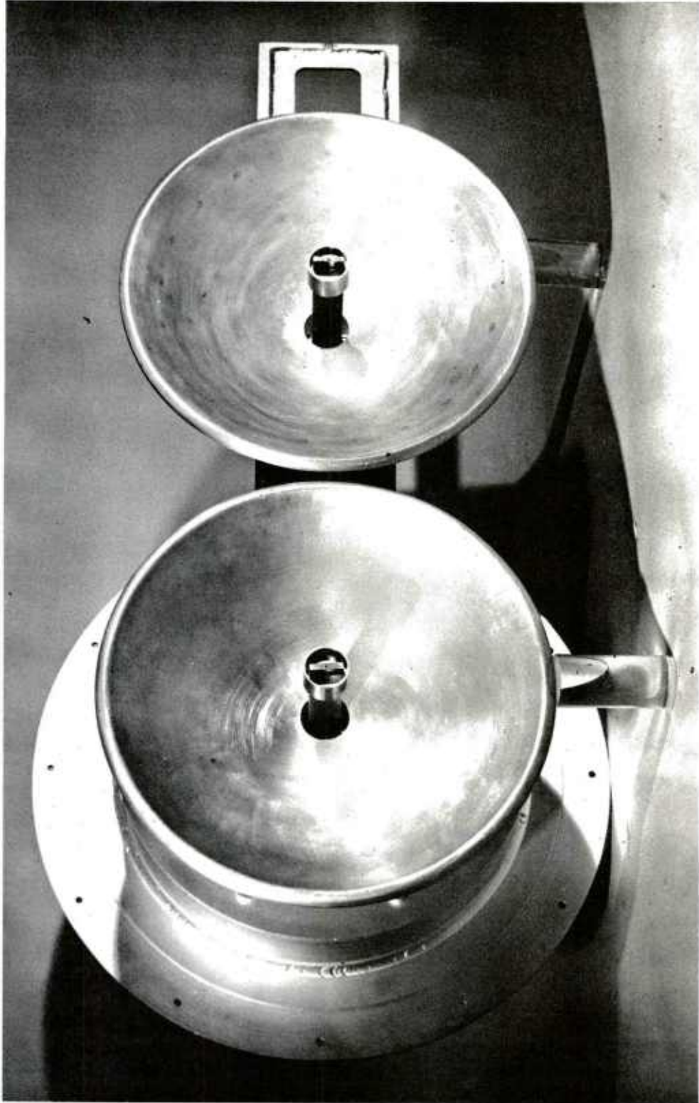
Fig. 15. 8.0 Gcps feed shown with side mounted reference antenna.
