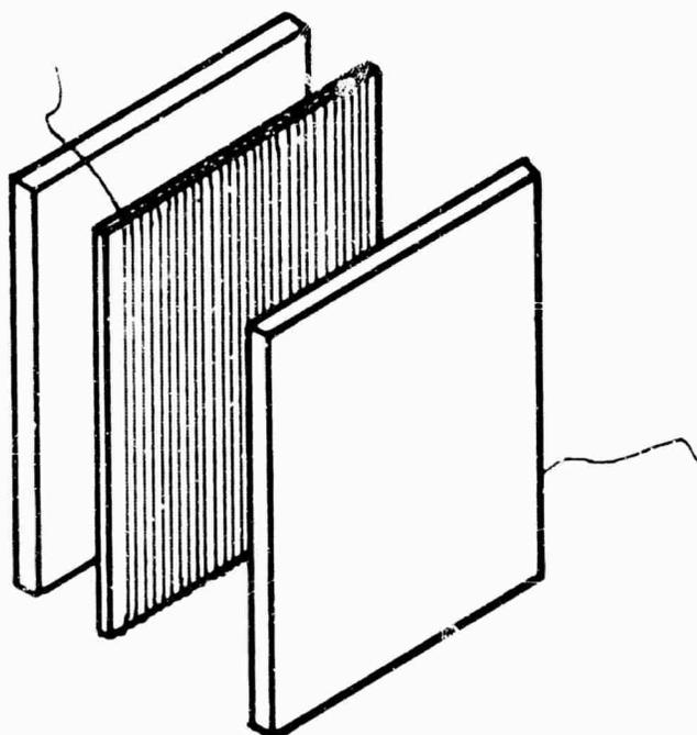
Figure 28. Platinum-Wire Bolometer (exploded view)
