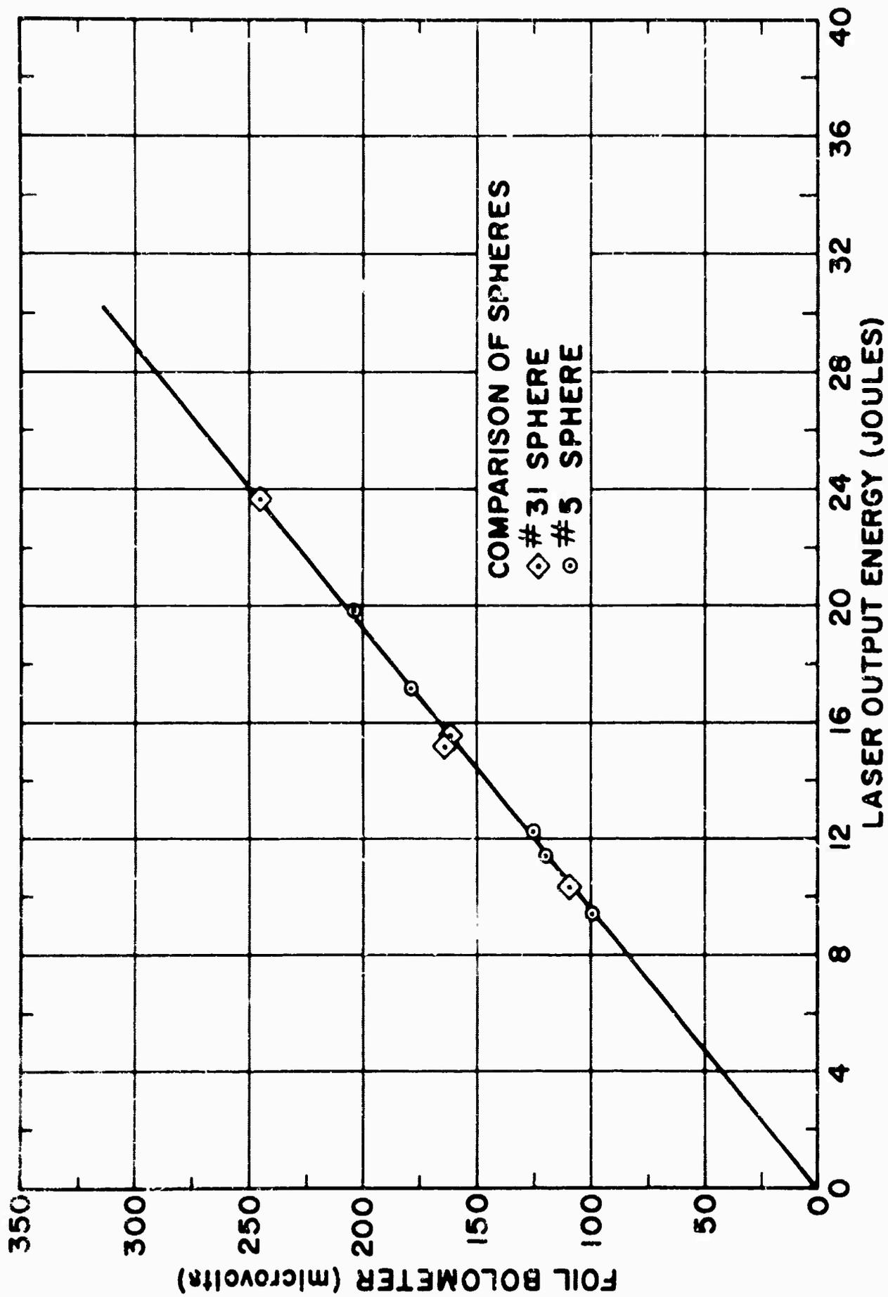
Figure 46. Double Calibration of Foil Bolometers
