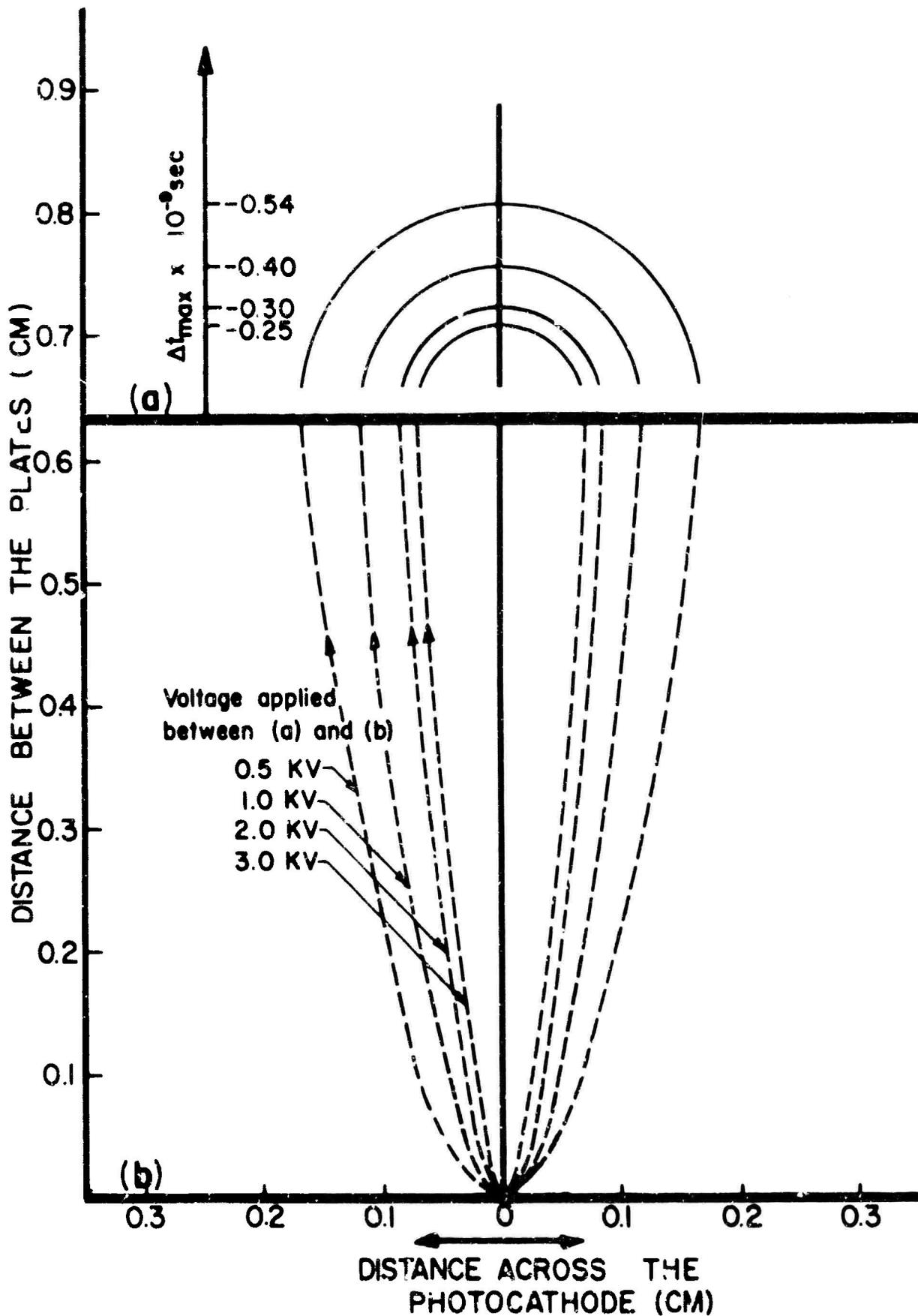
Figure 33. Electron Trajectories in Vacuum Phototube 7,000 Å Light
