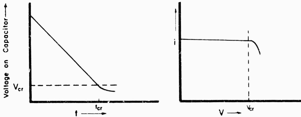
a. Capacitor discharge with time (assume a square-shaped light pulse)
