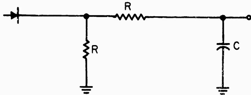
Figure 30. Complete Integrator Circuit
