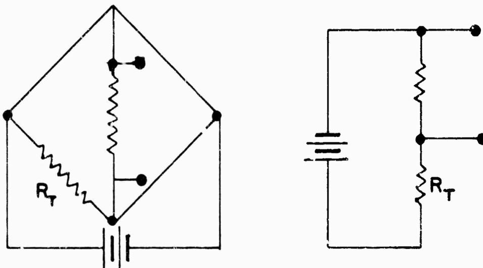
Figure 8. Simplest Thermistor Circuits
