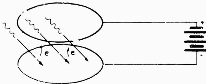
Figure 32. Parallel-Plate Photodetector Circuit
