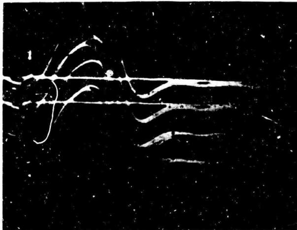
Figure 54. Diode Response to Kerr Cell Shutter
