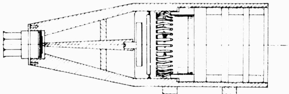
Figure 34. Diode Housing
