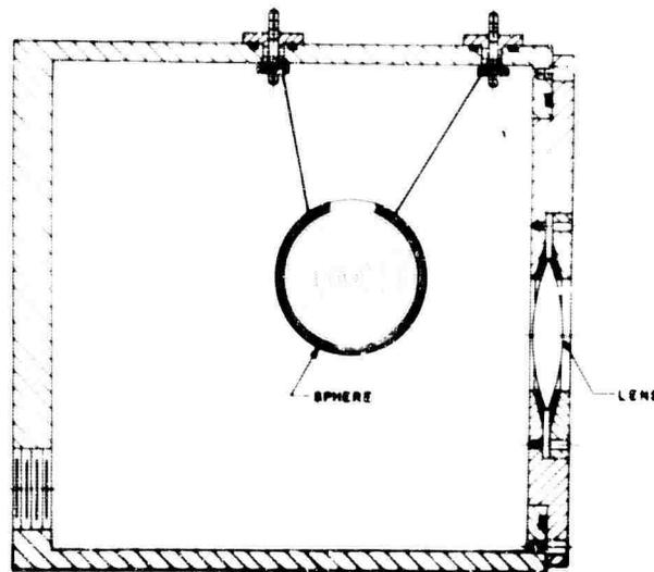
Figure 14. Calorimeter Vacuum Chamber
