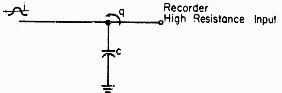
Figure 29. Basic Integrator Circuit
