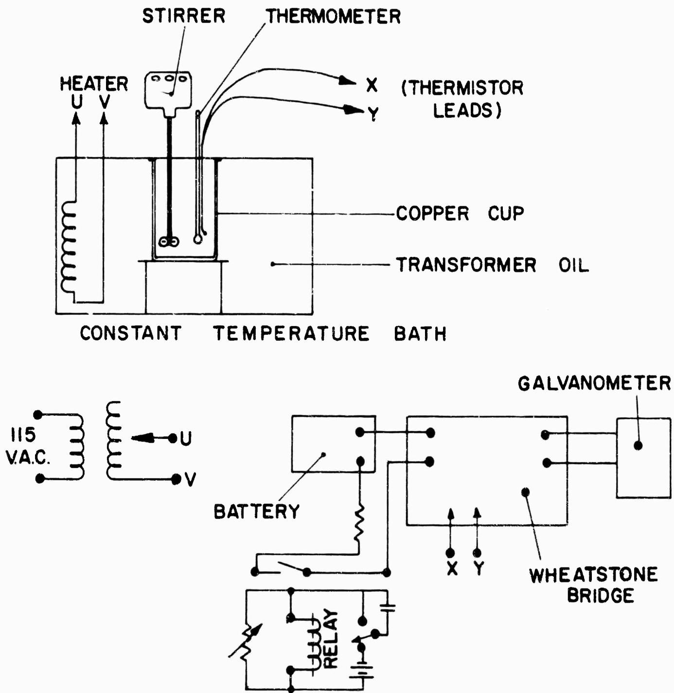
Figure 4. Schematic of Thermistor Calibration
