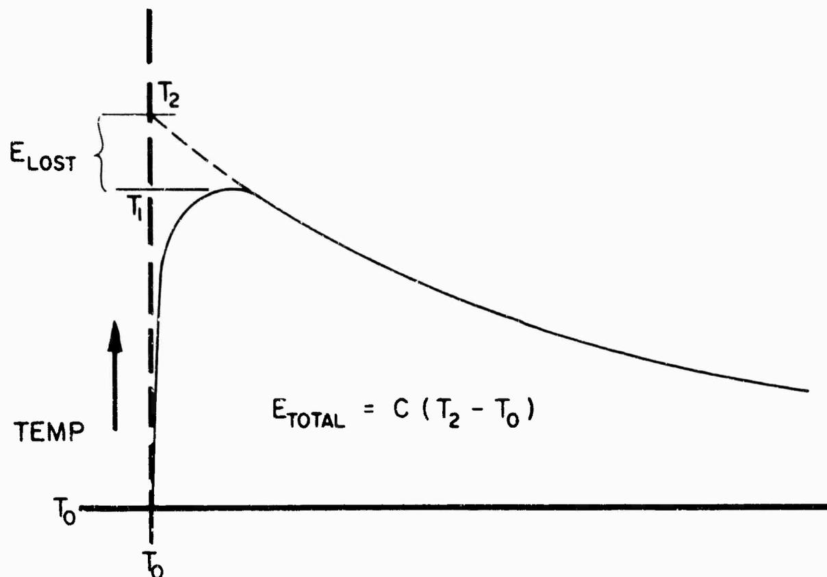
Figure 20. Temperature Decay (an exaggerated case)
