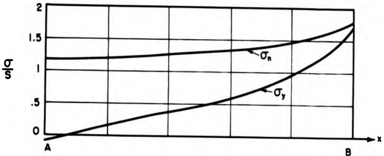
**Stress Distributions Thru the Wall Thickness of Model N-1EA**
