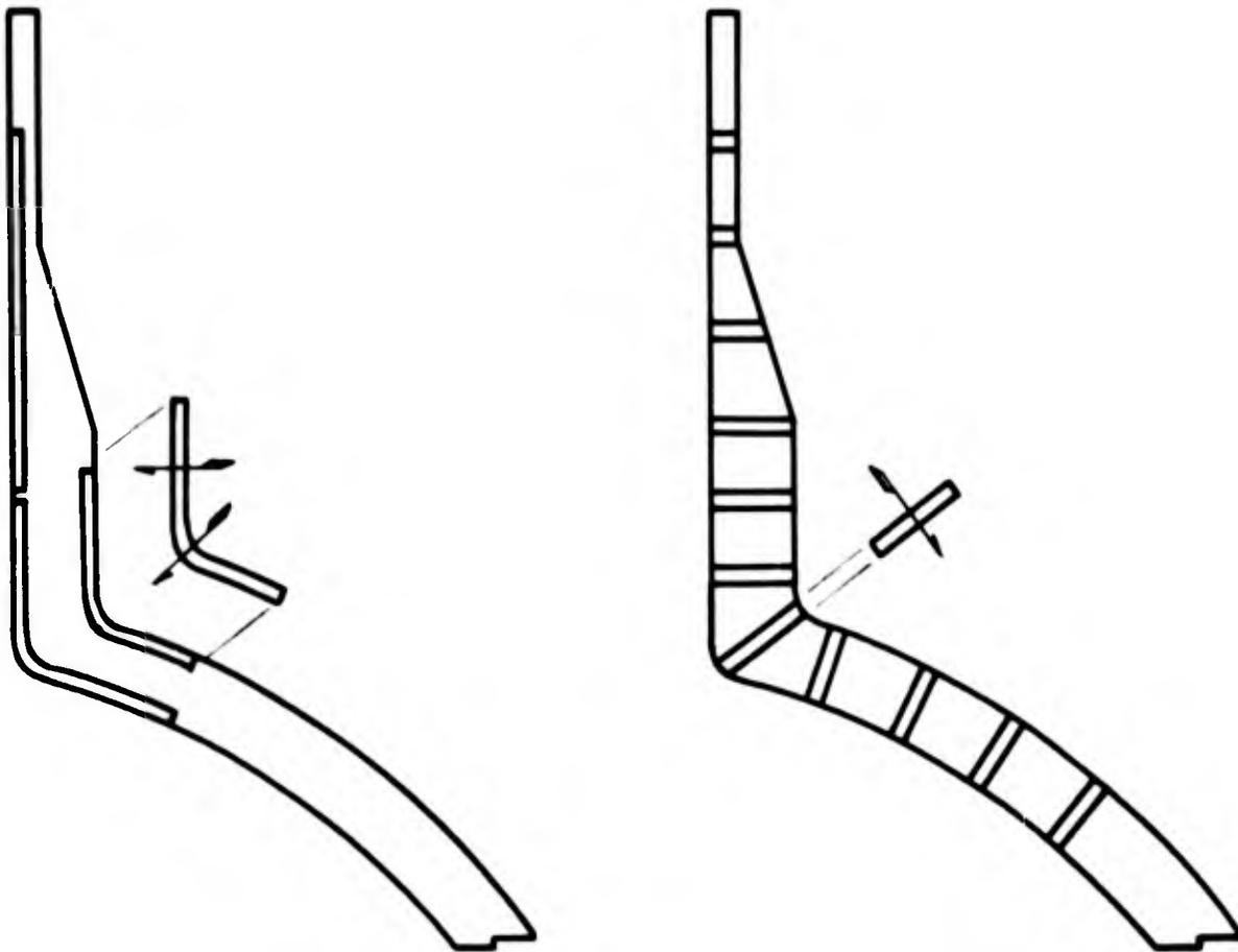
Fig. 3. Methods for Subslicing Model. The figure at the left shows surface subslices and light would pass in the  $r$ -direction through the subslice as indicated by the arrows. For a model subsliced as shown by the figure on the right, the light would travel in the  $t$ -direction.
