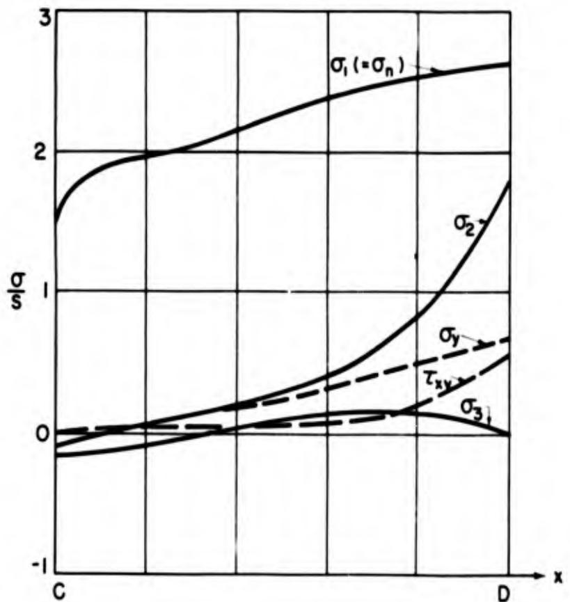
**Stress Distributions Thru the Wall Thickness of Model N-1A**
