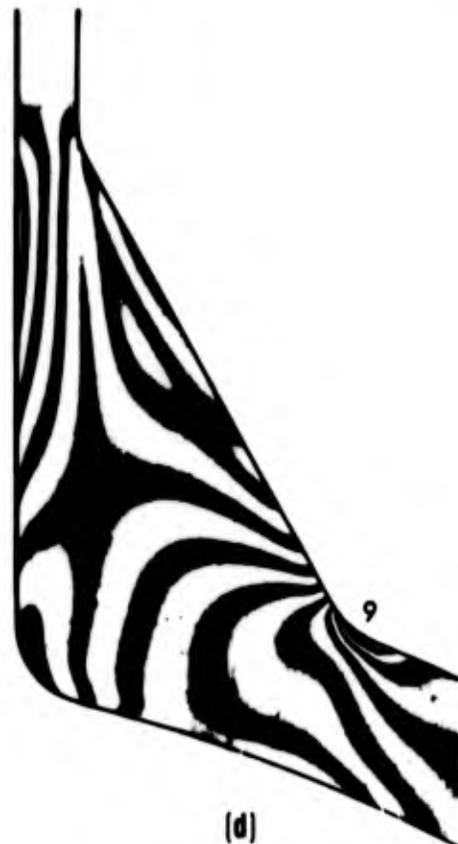
**Fig. 1 Typical Fringe Photographs (a) Cylindrical Model E-4E (b) Spherical Model N-1A (c) Reinforced Spherical Model N-4A and (d) Reinforced Spherical Model N-4D Numerals on Figures Indicate the Fringe Orders**
