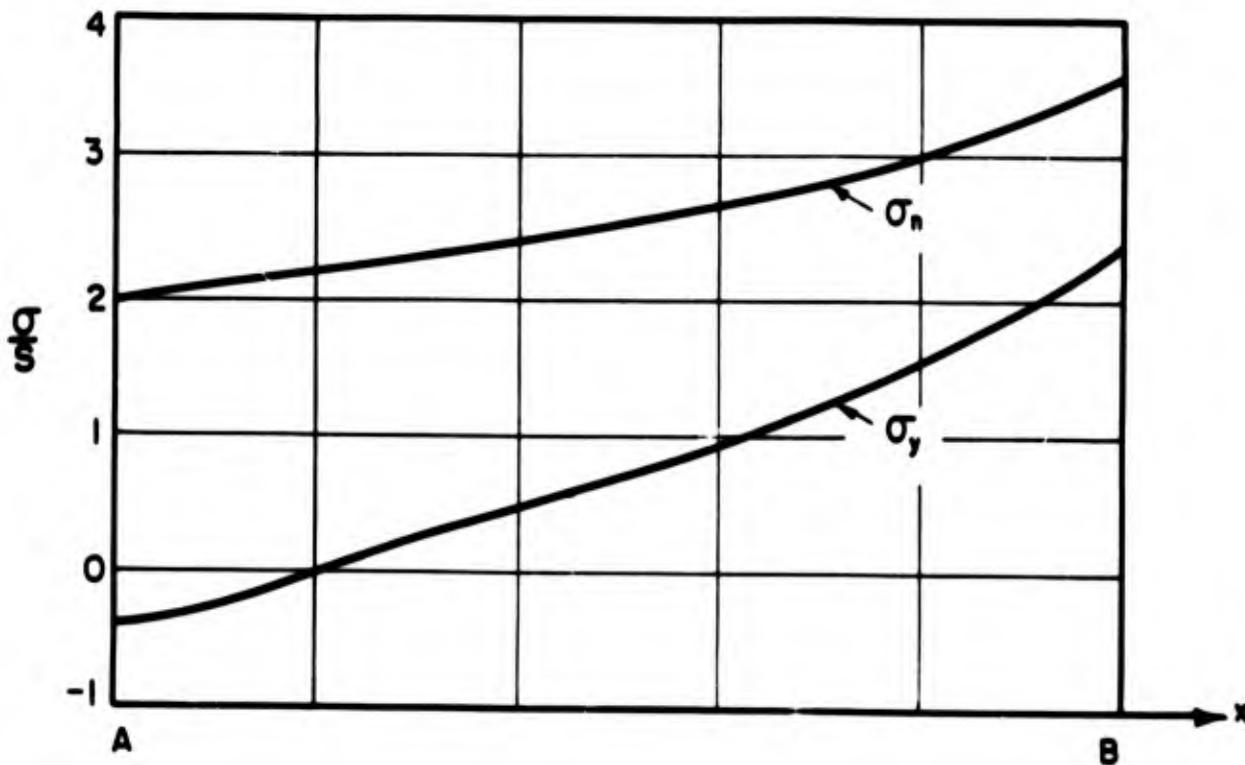
**Stress Distributions Thru the Wall Thickness of Model S-5C**
