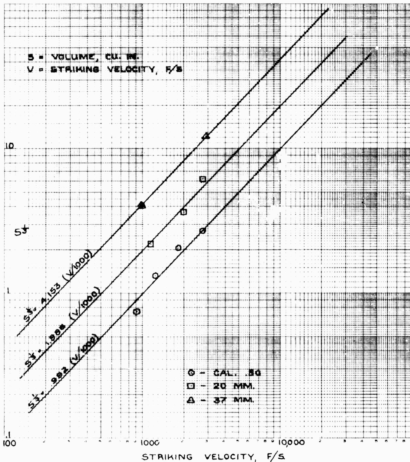
PLOT 14. CUBE ROOTS OF CRATER VOLUMES DUE TO VARIOUS PROJECTILES FIRED INTO DIABASE VS. STRIKING VELOCITY (SINGLE ROUNDS)
