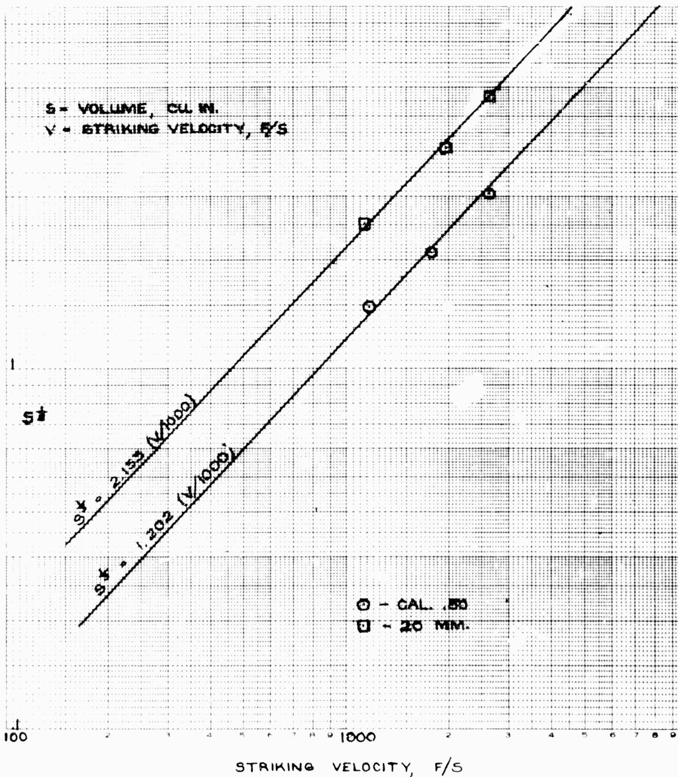
PLOT 16. CUBE ROOTS OF CRATER VOLUMES DUE TO VARIOUS PROJECTILES FIRED INTO INDIANA LIMESTONE vs. STRIKING VELOCITY (SINGLE ROUNDS)
