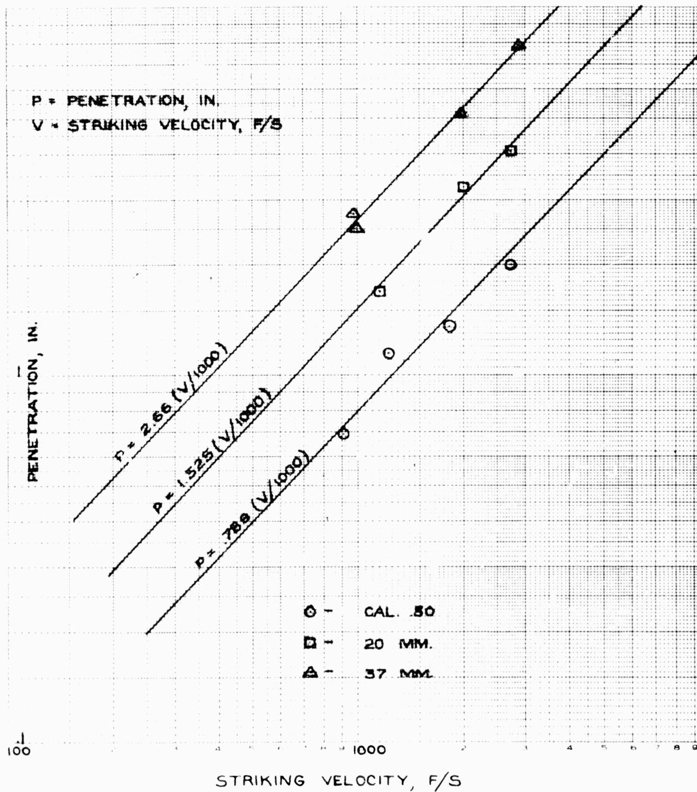
PLOT 2. PENETRATION OF VARIOUS PROJECTILES INTO DIABASE vs. STRIKING VELOCITY (SINGLE ROUNDS.)
