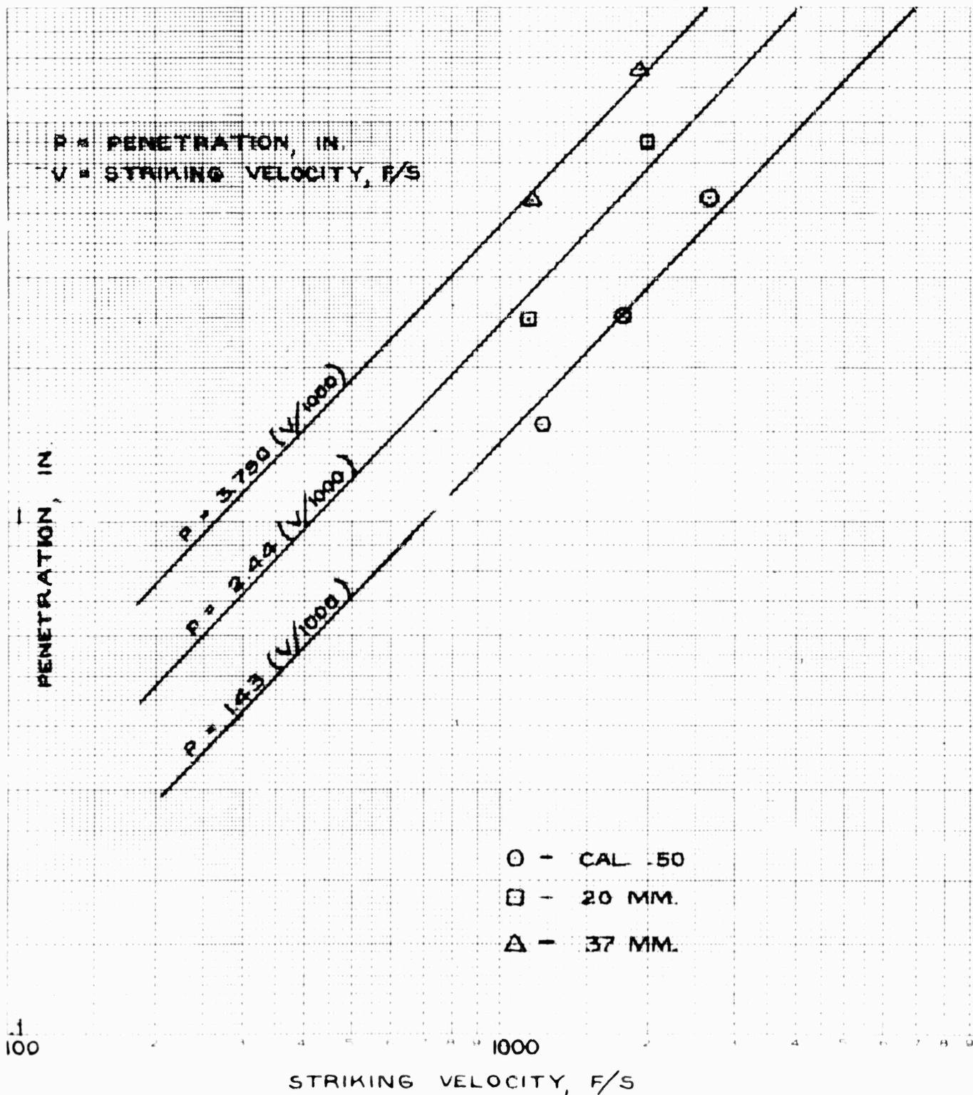
PLOT 5. PENETRATION OF VARIOUS PROJECTILES INTO SANDSTONE vs STRIKING VELOCITY (SINGLE ROUNDS).
