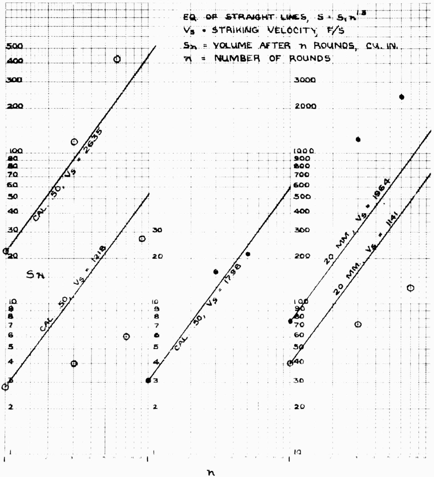
PLOT 27. CRATER VOLUME IN REPEATED ROUNDS, FIRED INTO QUARTZITE.
