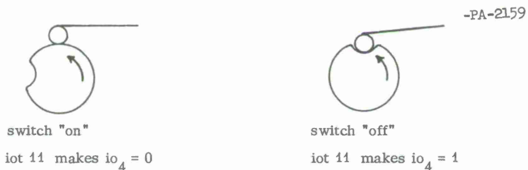
Fig. 7 Cam-microswitch combination
