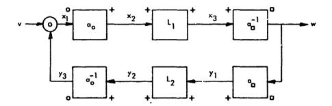
Fig. 11. Equivalent representation of a homomorphic feedback system.
