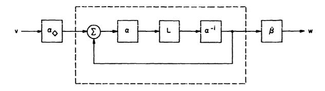
Fig. 16. Equivalent representation of the feedback system of Fig. 13 for the case in which  $\gamma$  is invertible.
