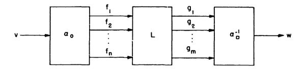
Fig. 8. Canonic representation of a homomorphic system with memoryless input and or out operations.
