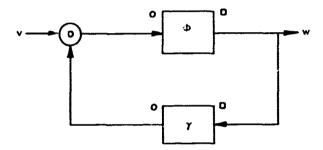
Fig. 10. Homomorphic feedback system with nonadditive feedback.
