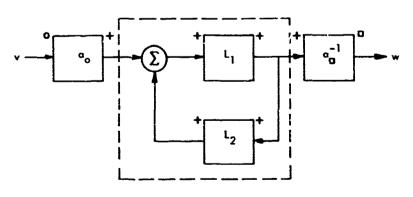
Fig. 12. Canonic representation of a homomorphic feedback system.
