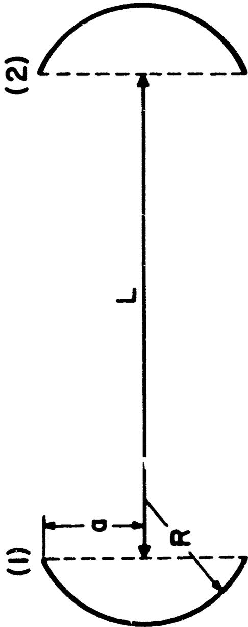
FIGURE 1. ILLUSTRATING RESONATOR CONFIGURATION
