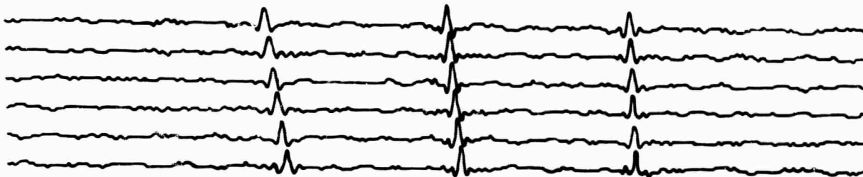
Figure 6.2 - 5: Example of application of band-pass and band-pass, band-reject filters to simulated noise and signal traces.
