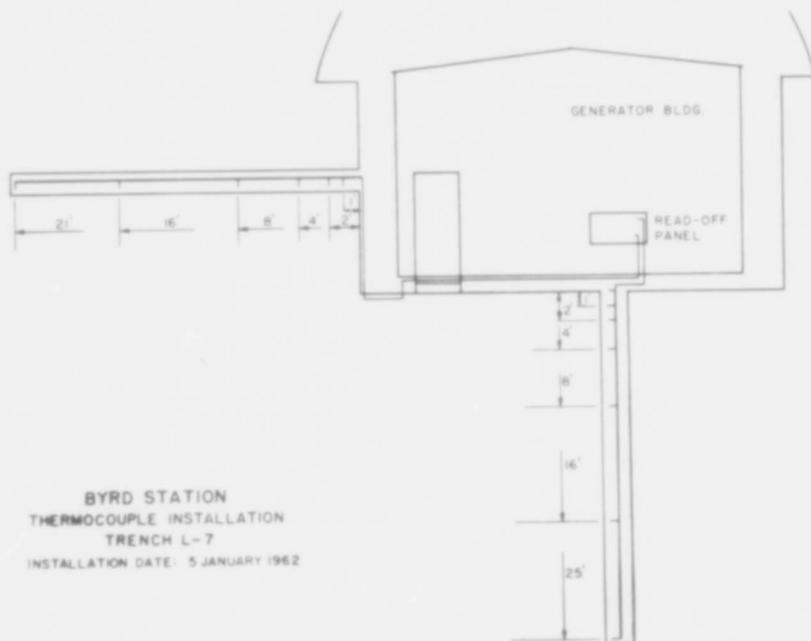
Figure 6. Arrangement of thermocouples in trench L-7.
