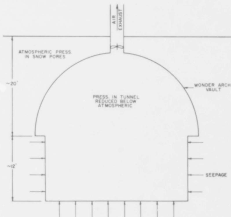
Figure B2. Proposed method for drawing cold air into a closed tunnel from the permeable snow mass.
