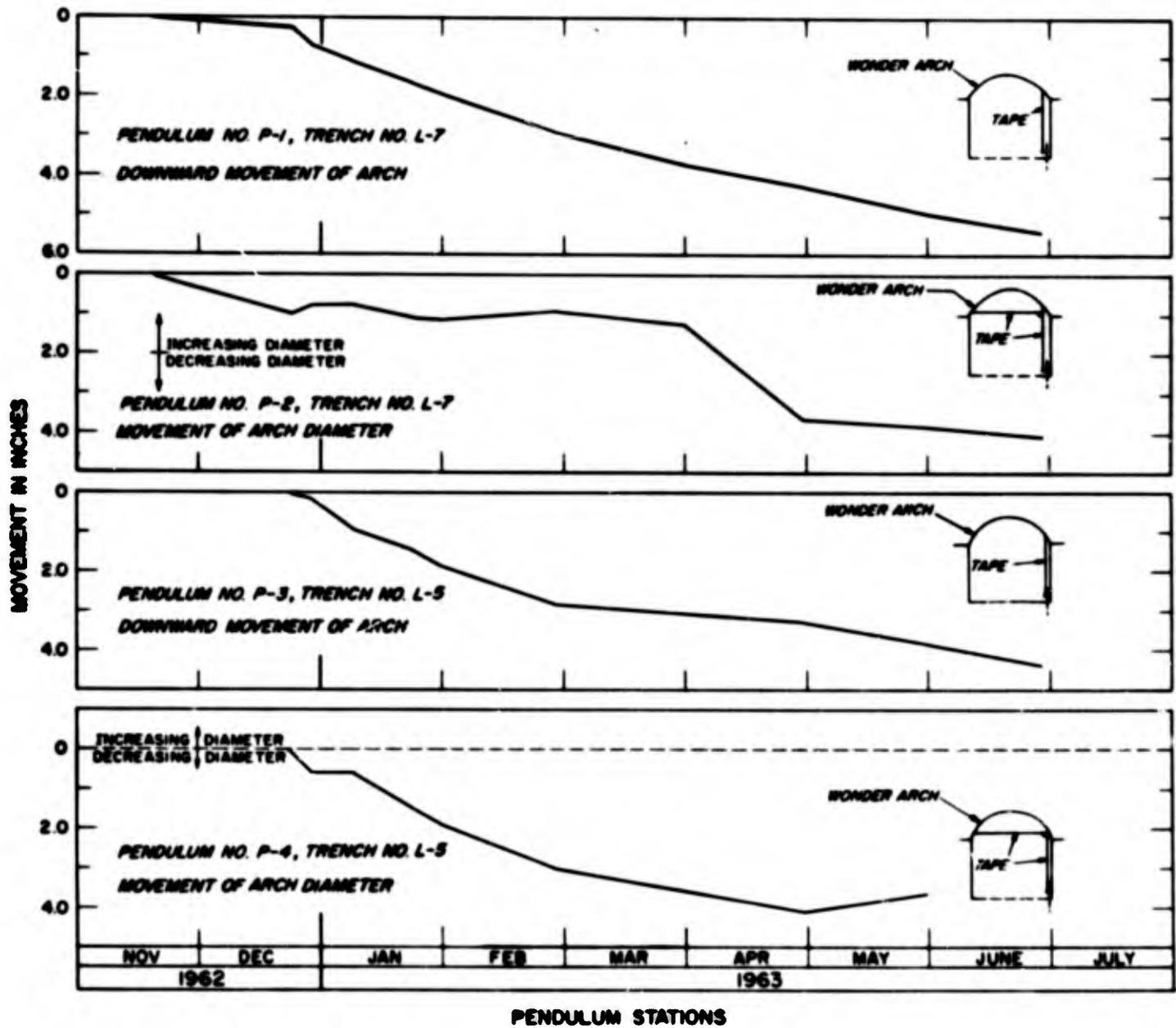
Figure 26. Records for pendulum gages.
