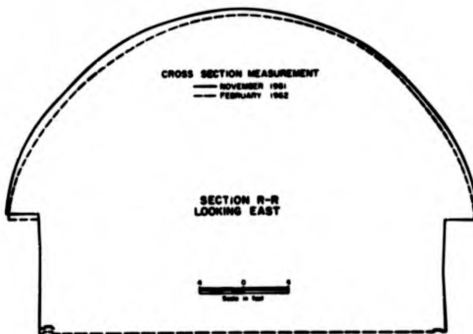
Figure 15. Cross-section profiles at section R - R in trench L - 3.
