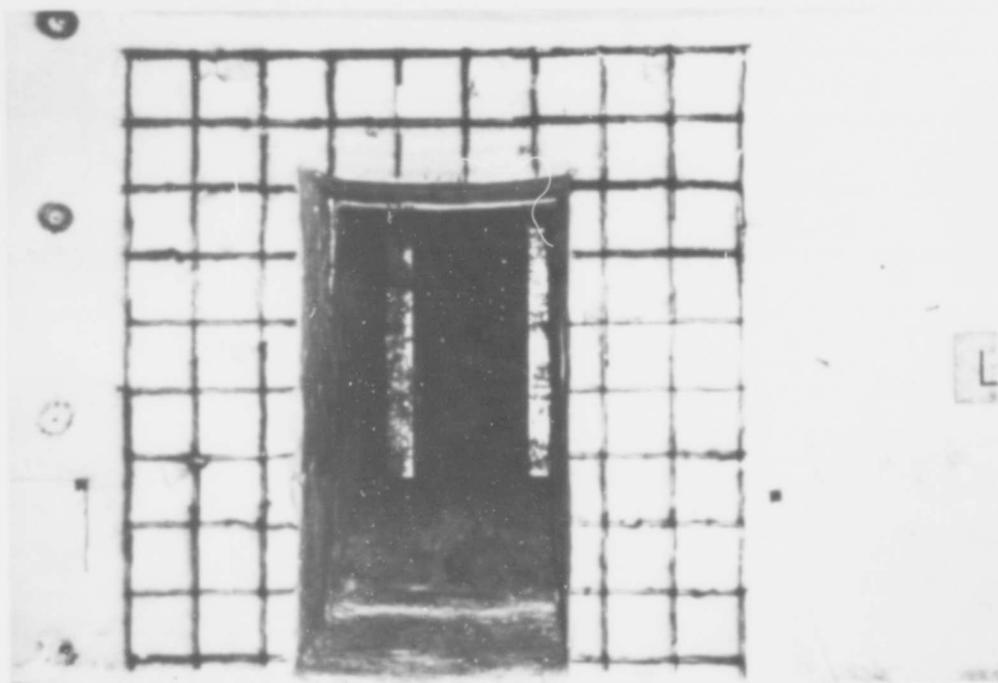
Figure 5. Deformation grid marked on the snow wall at the entrance of the passageway from M-1 into L-2. The sagging roof of the passage, and the faintly visible natural strata, show that some deformation occurred before the grid was marked. (Official U. S. Navy photograph)
