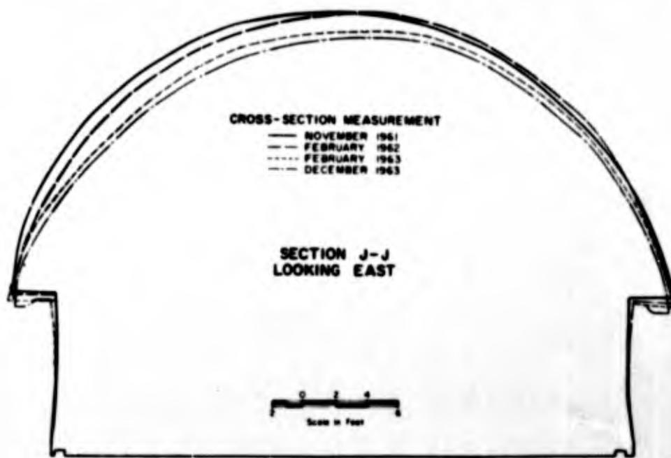
Figure 16. Cross-section profiles at section J - J in trench L - 3.
