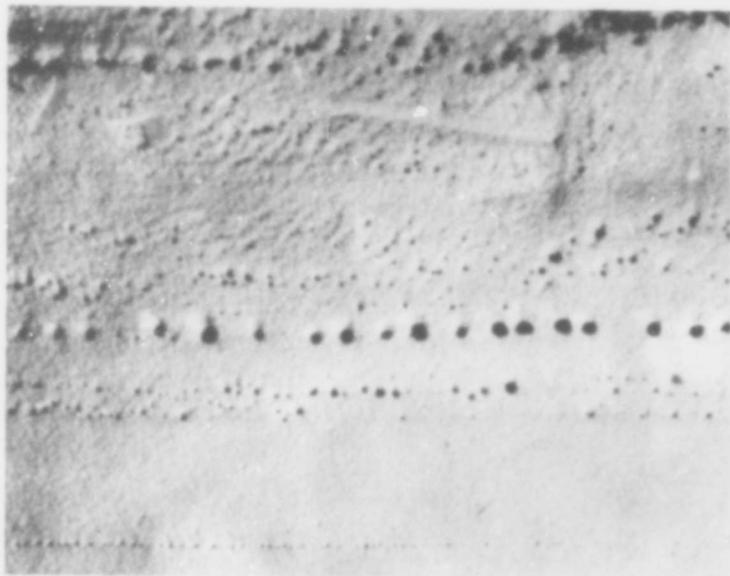
Figure B1. Holes in the surface of a snow wall, produced by evaporation as air flows out into the tunnel from the pores of the snow mass.
