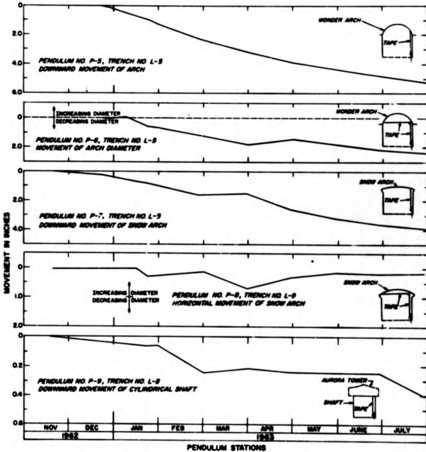
Figure 26 (Cont'd). Records for pendulum gages.
