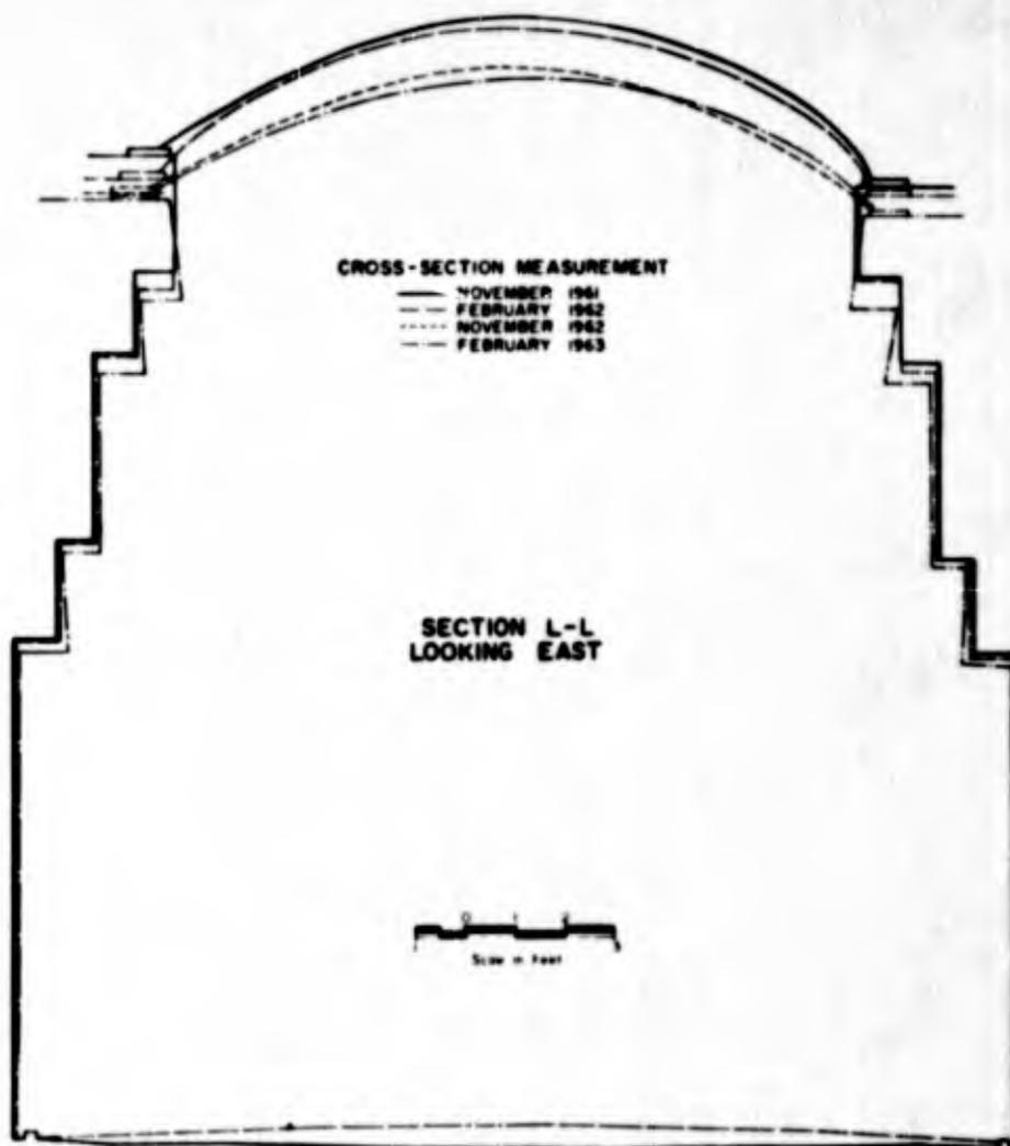
Figure 17. Cross-section profiles at section L - L in trench L - 4.
