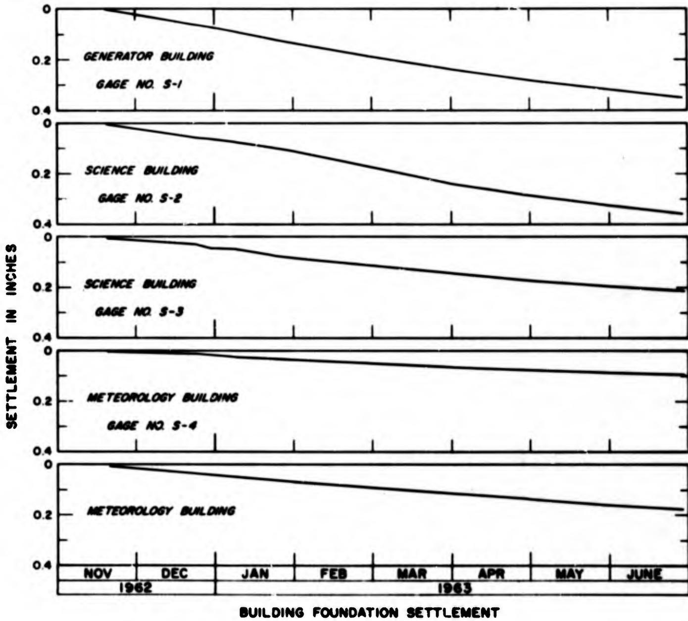
Figure 28. Records for foundation settlement gages.
