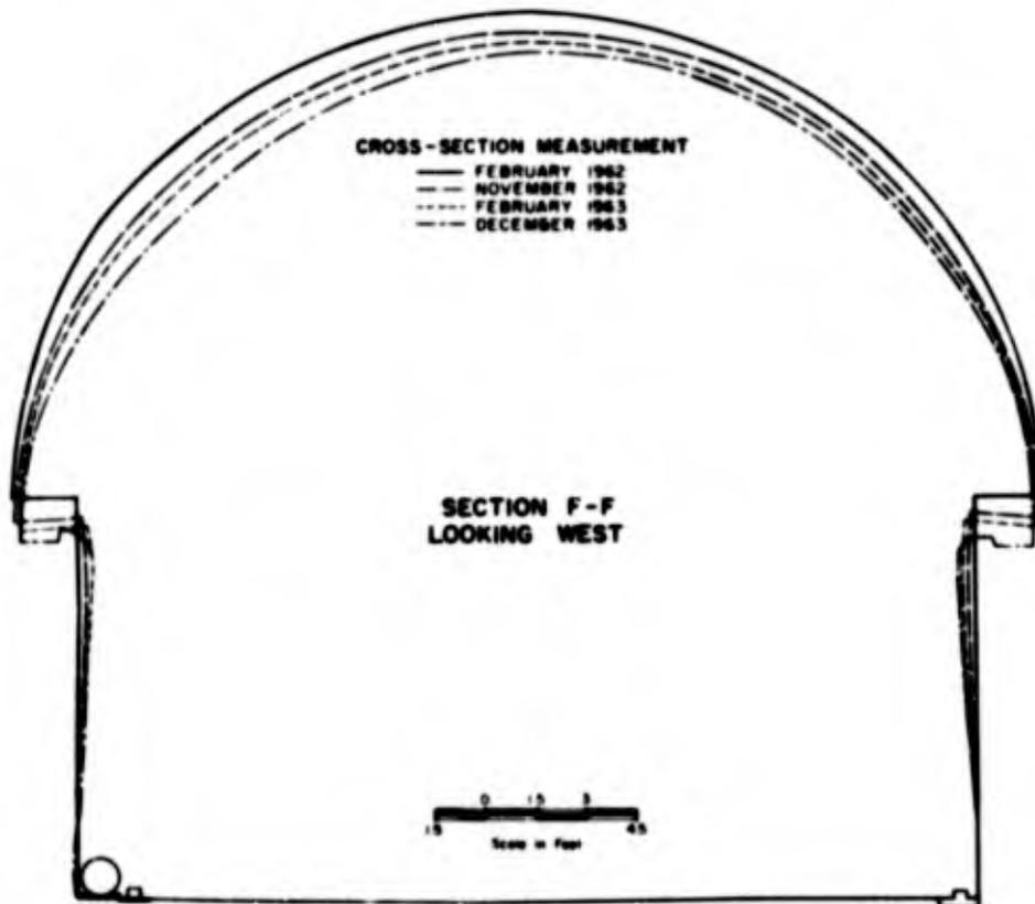
Figure 11. Cross-section profiles at section F - F in trench L - 5.
