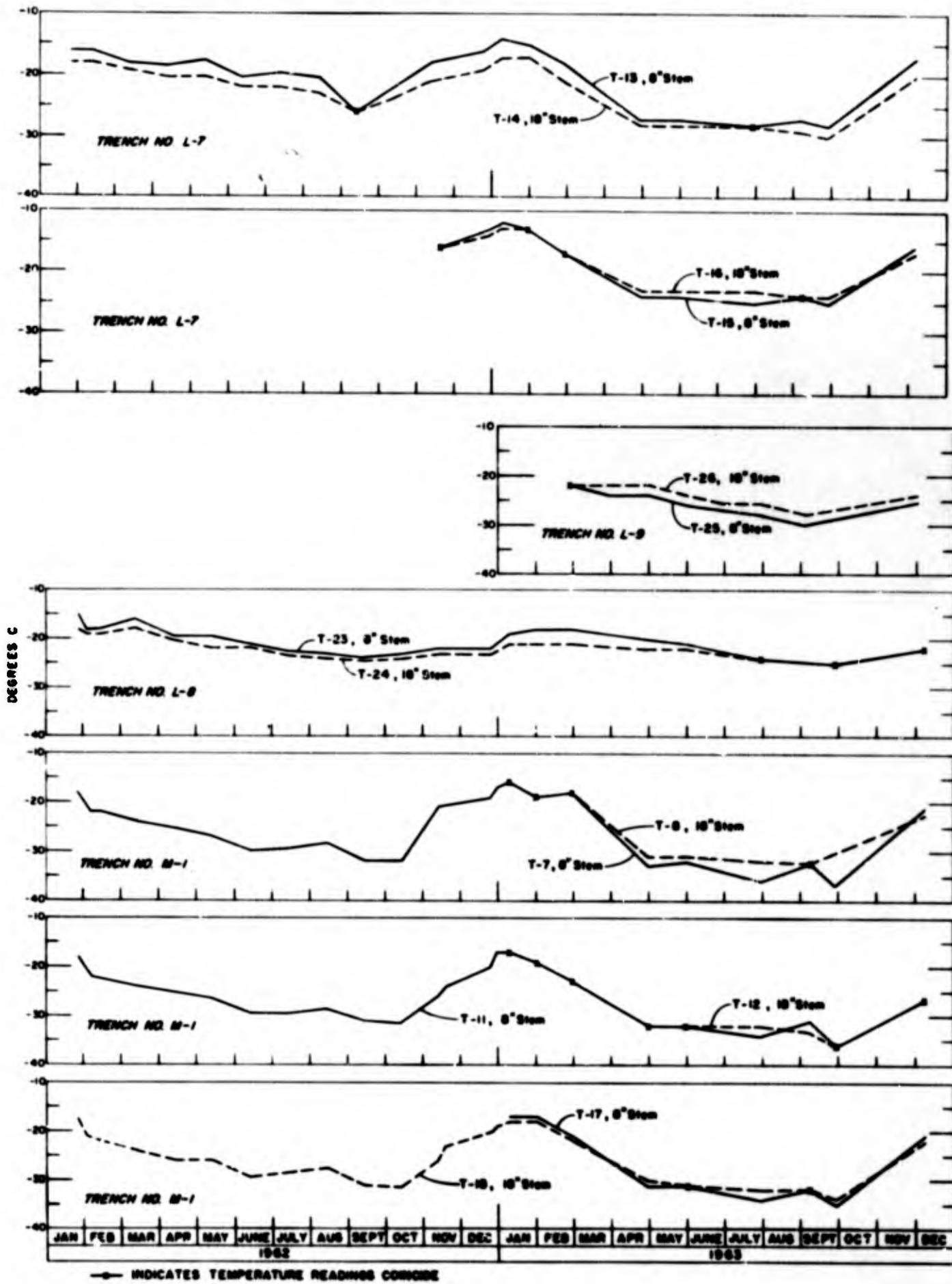
Figure 29 (Cont'd). Records from dial thermometers in trench walls.
