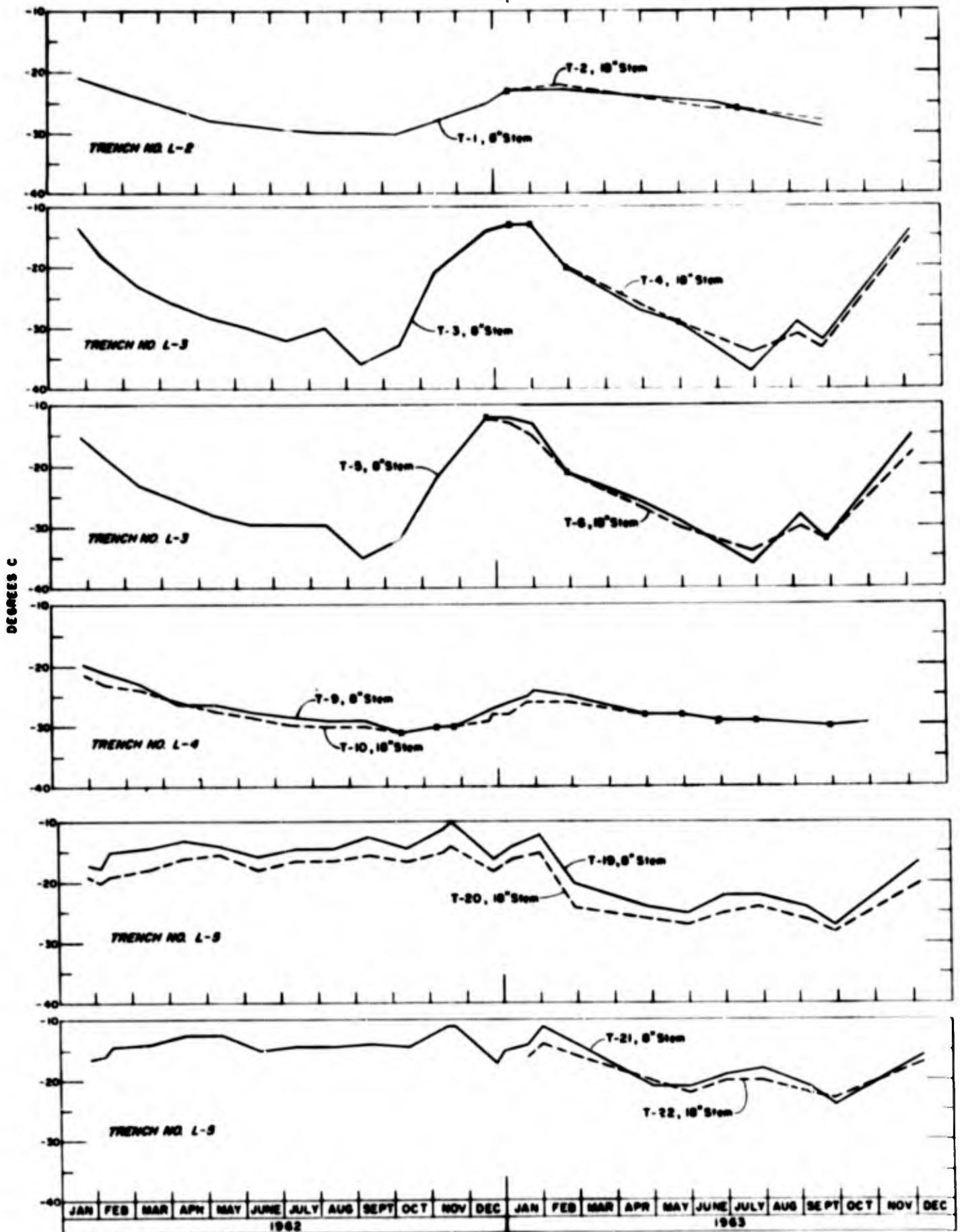
Figure 29. Records from dial thermometers in trench walls.
