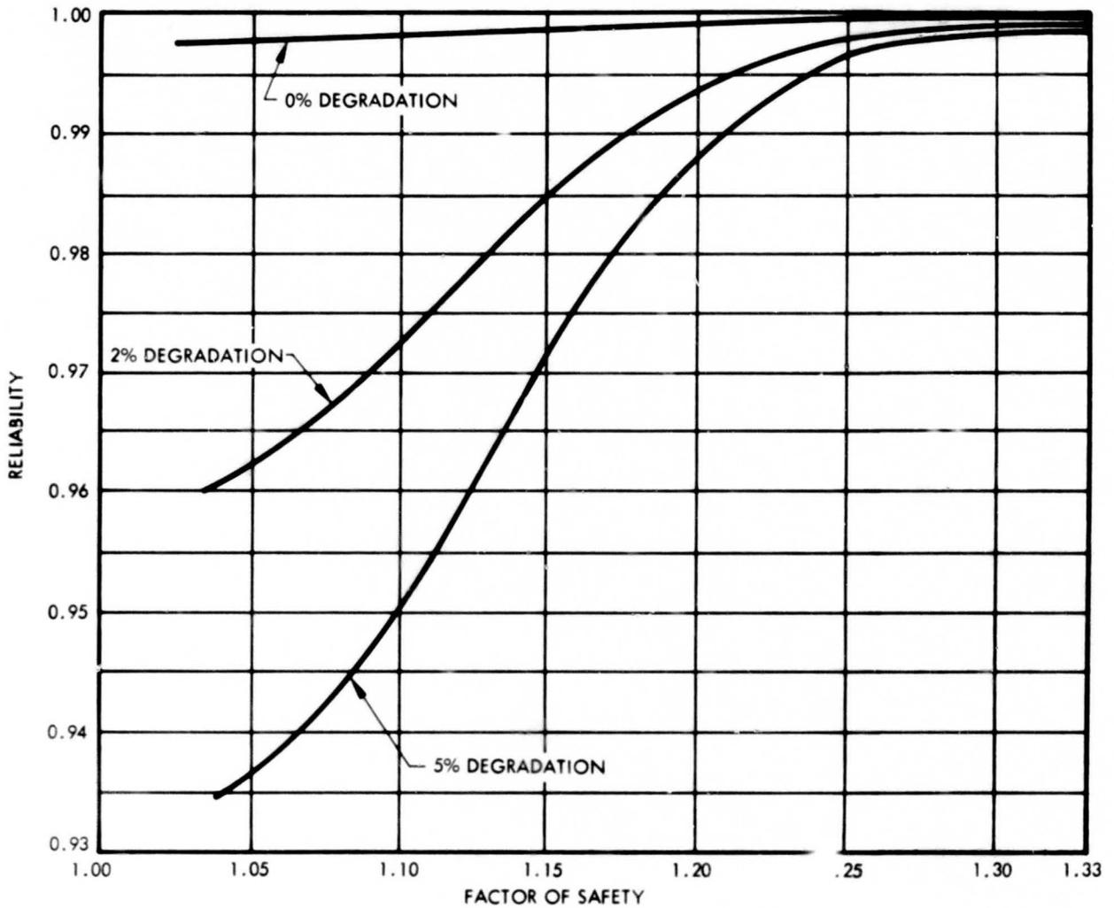
$$\text{FACTOR OF SAFETY} = \frac{\text{ORIGINAL MEAN STRENGTH}}{\text{PROOF PRESSURE LEVEL}} = \frac{\text{ORIGINAL MEAN STRENGTH}}{945 \text{ psig}}$$
