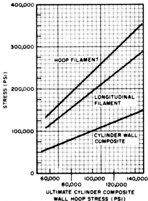
**FIGURE B-1. STRUCTURAL AND DIMENSIONAL REQUIREMENTS FOR LARGE GLASS FILAMENT-WOUND MOTOR CASE OF 260-IN.-DIA AND 113 FT LENGTH**
