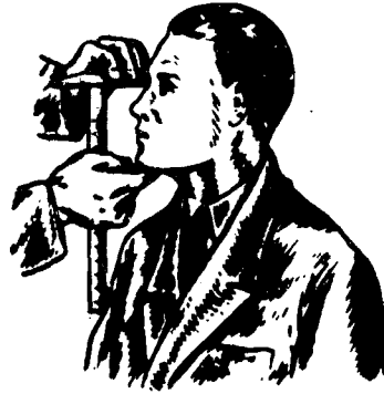
Fig. 5. Measuring the height of the face with sliding calipers.
