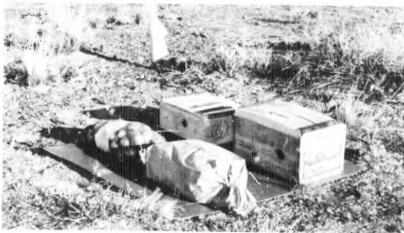
Fig. 3—Semiperishable foods arranged on ground surface at Station C (1 mile), Shot L.
