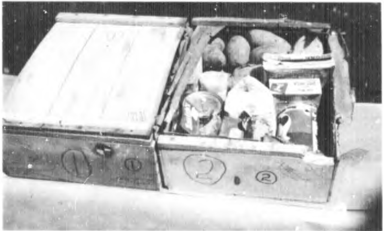
Fig. 16—Box buried flush with ground with no soil cover at Station A (1100 ft) (right). (Note destruction of cover and loss of polyethylene potato bag.) Check box not exposed (left).
