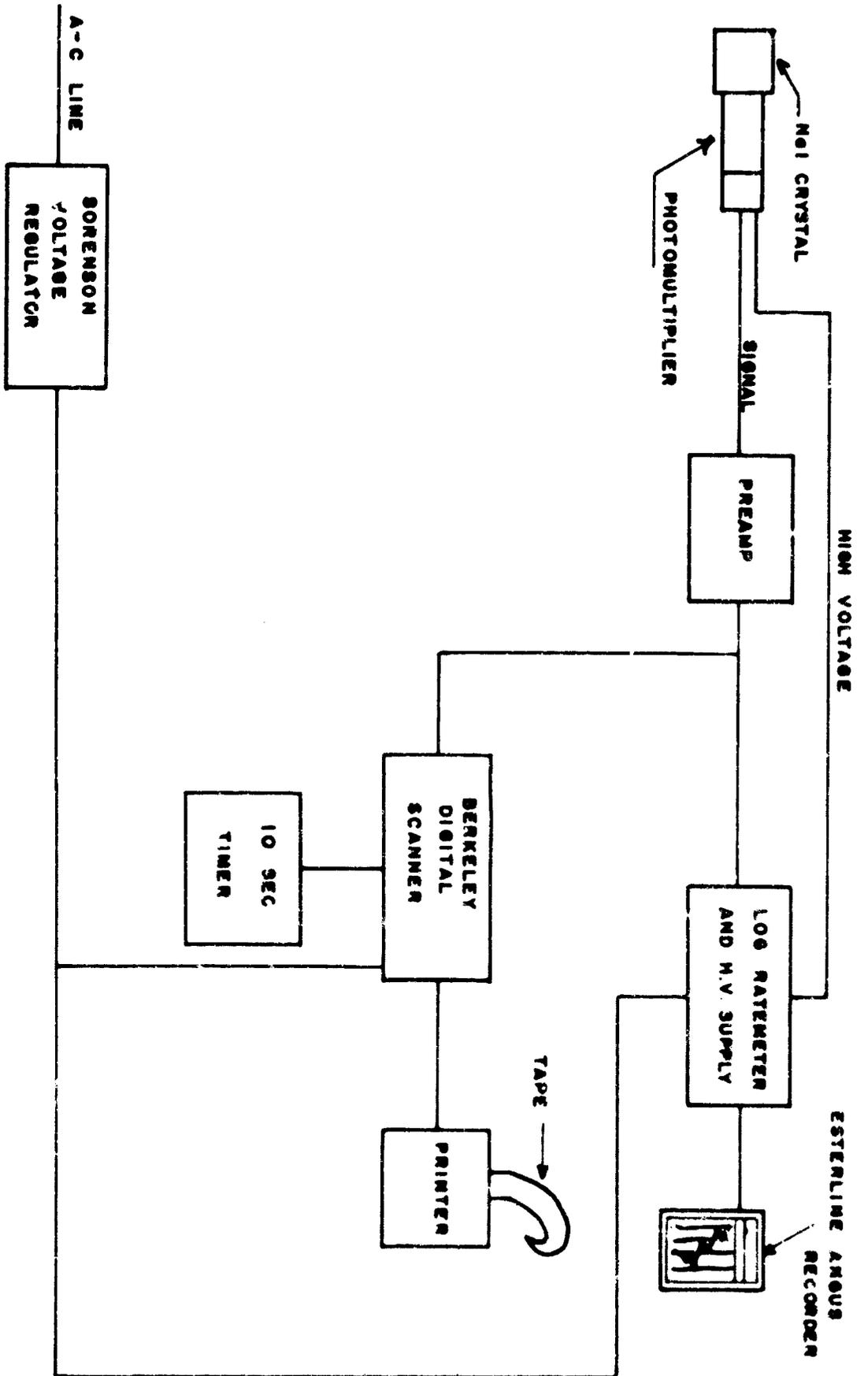
Fig. B.3—Block diagram of directional gamma apparatus.
