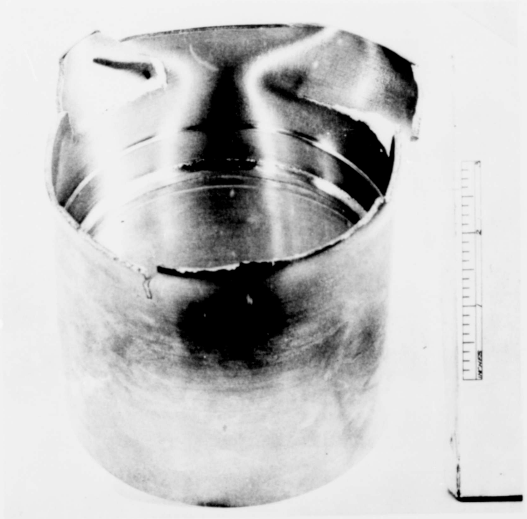
COMPRESSION TEST ON THIN WALLED PRESSURE WELDED CYLINDER - 100% WELD EFFICIENCY LOAD - 212,000 LBS
