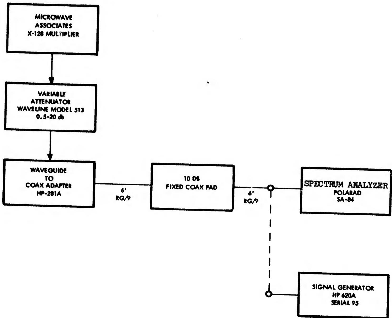
Figure III-1 Equipment Set-Up for Measuring Spectral Composition of Exciter Output
