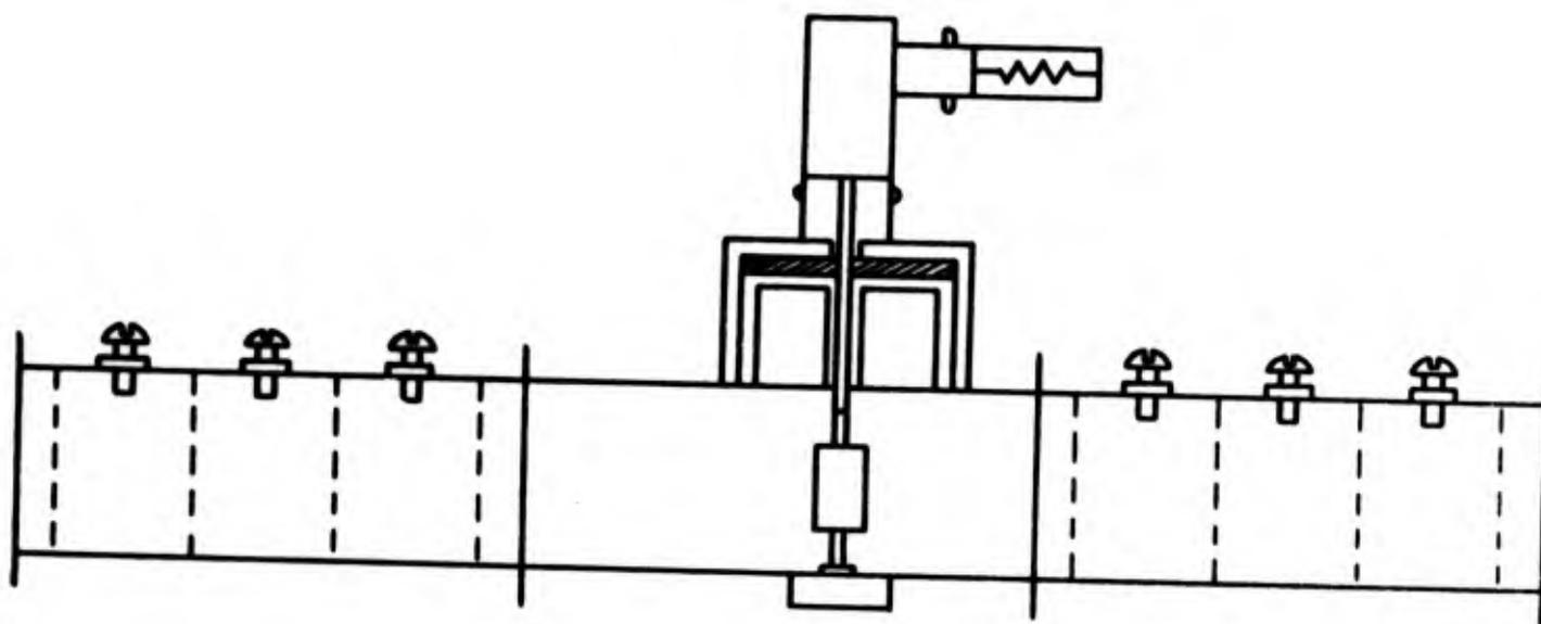
Figure 3-26. Upper Sideband Upconverter (7630/8330 Mc)
