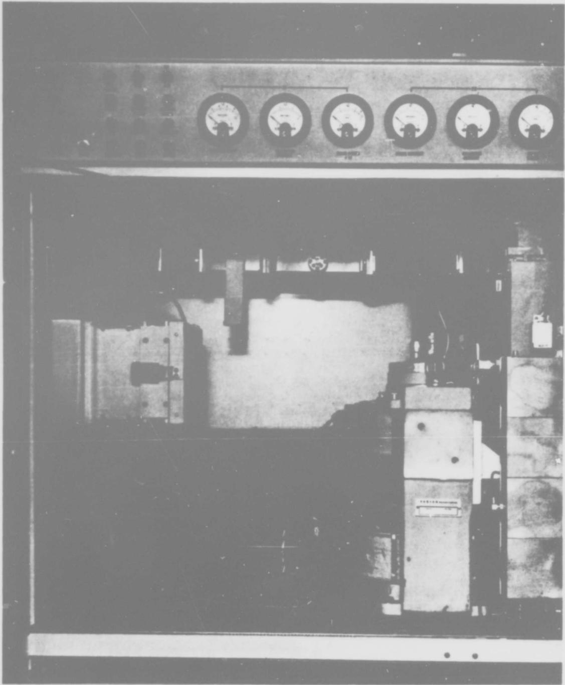
Figure 2-2. Left Hand Transmitter Cabinet Before Modification
