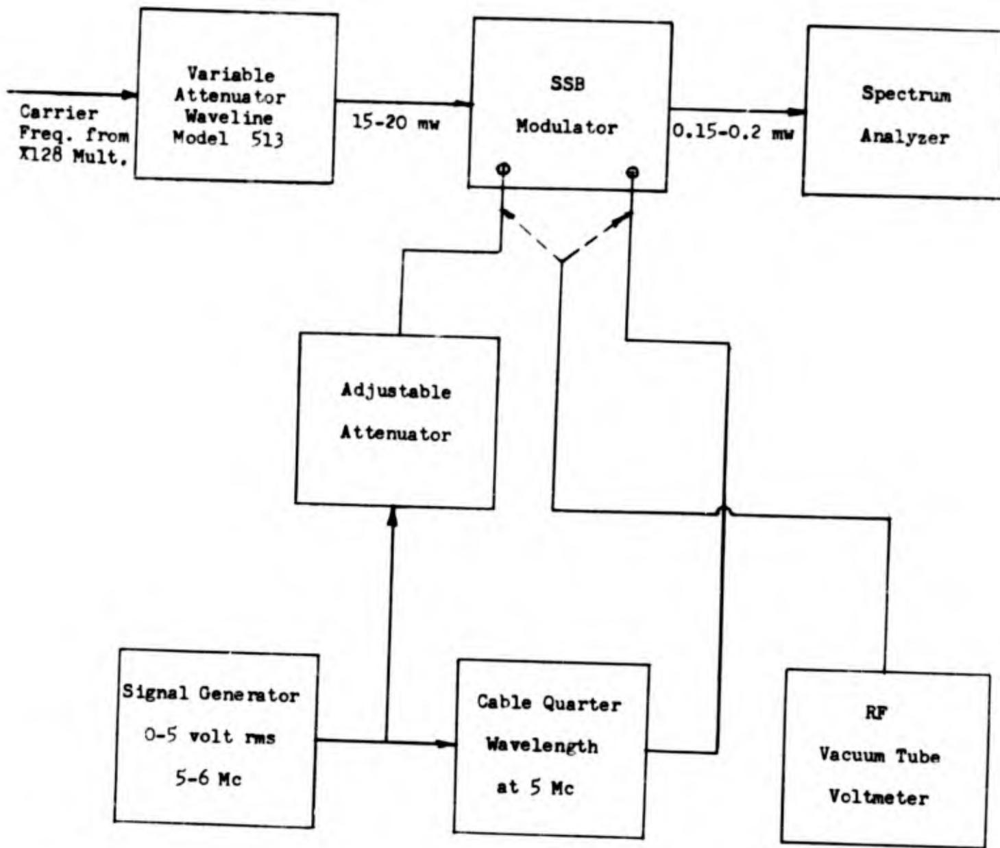
Test-Set-Up For Modulator Adjustment
