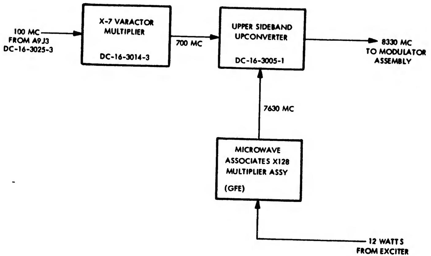
Figure 3-23. 700 Mc Offset Frequency Generator Block Diagram
