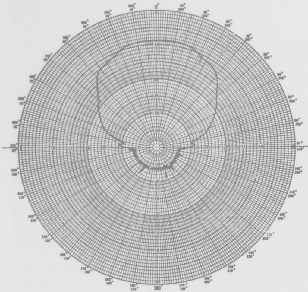
Figure 1-5. Radiation Pattern of Feed Horn Alone
