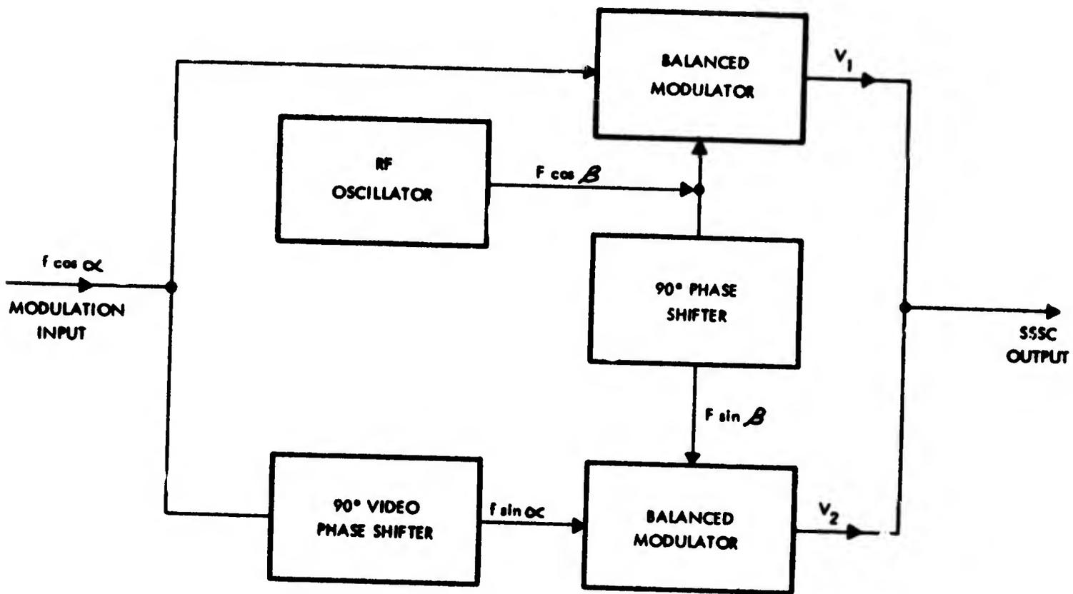
Figure II-1. Phase Discriminator SSB Modulator
