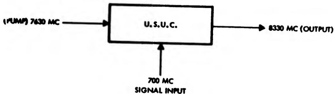
Figure 3-25. Upper Sideband Upconverter (7630/8330 Mc)
