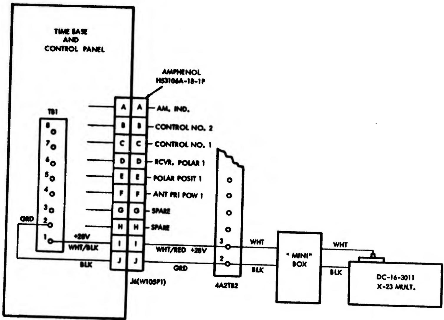
Figure III-3. Modification to Control Chassis Wiring
