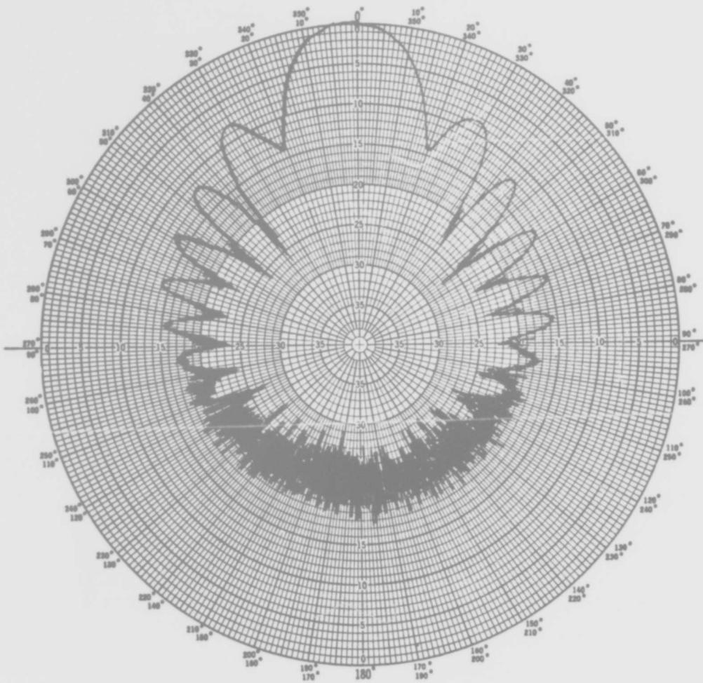
Figure 1-9. Radiation Pattern of Completed 8330 Mc Feed Assembly
