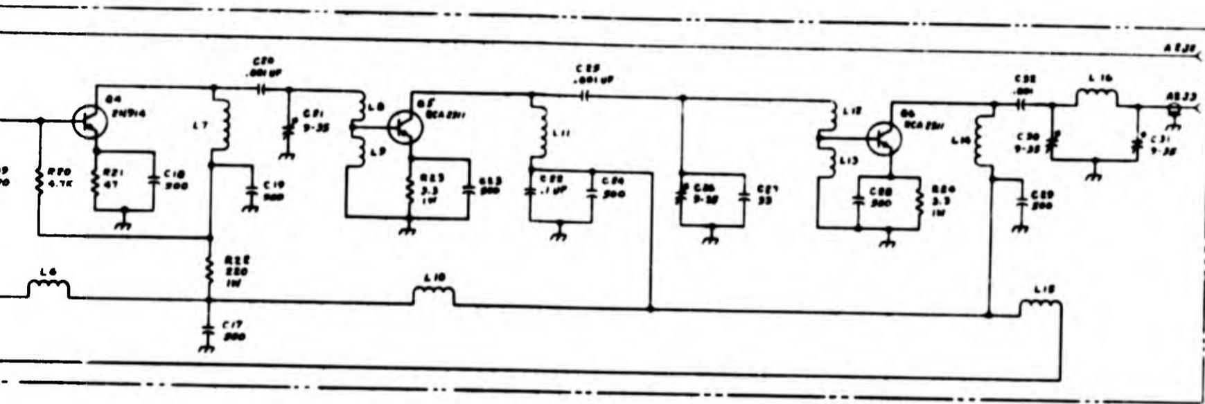
Figure 3-10. 100 Mc Power Amplifier Schematic Diagram
