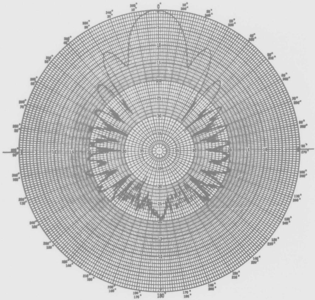
Figure 1-6. Radiation Pattern of Feed Horn with Disc-on-Rod Element
