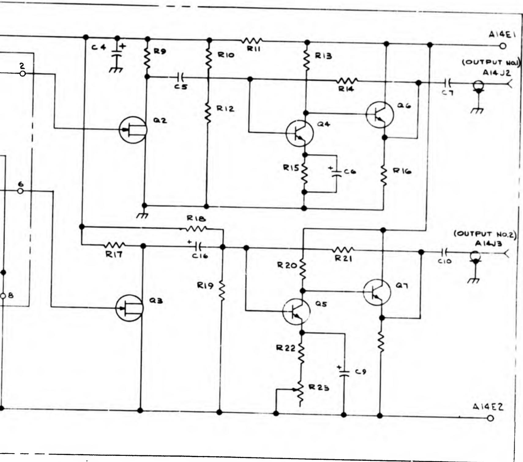
Figure 2-7. Quadrature Amplifier Schematic Diagram
