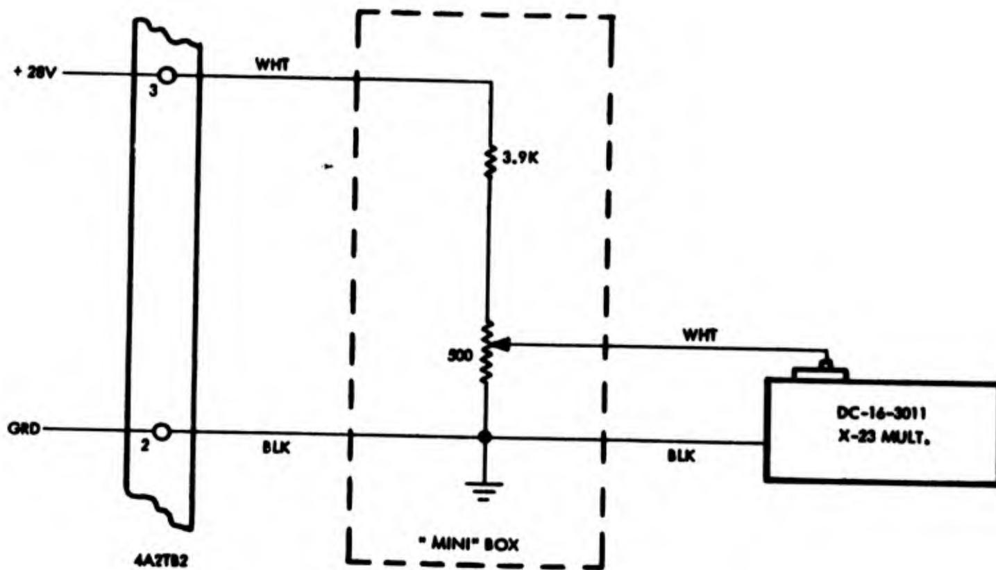
Figure III-2. Bias Circuit for X-23 Multiplier
