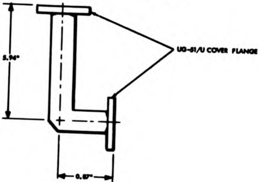
Figure III-5. Modulator Waveguide Change
