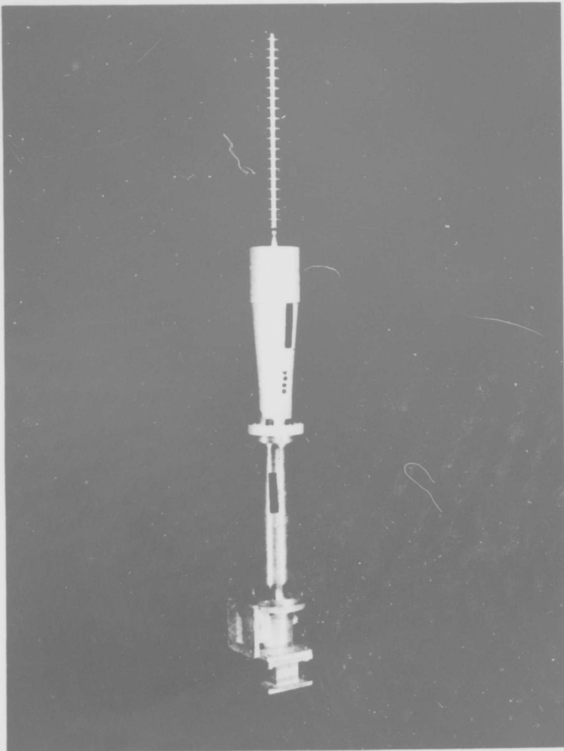
Figure 1-7. Completed Feed Assembly Showing Horn,
