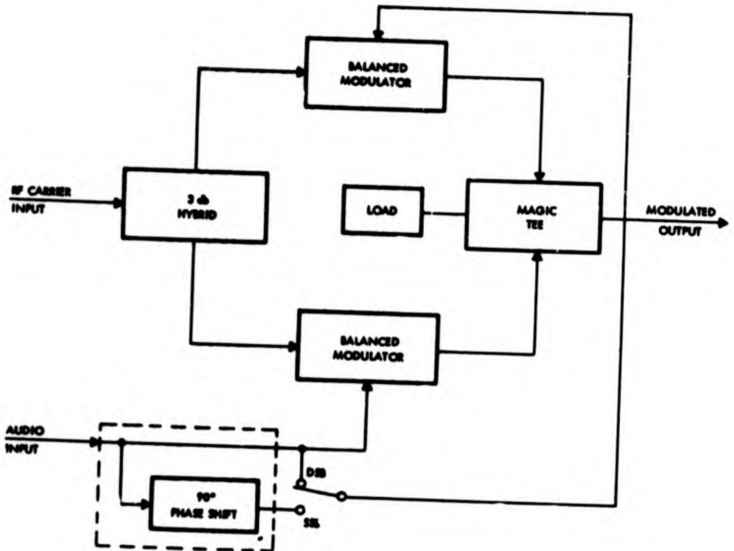
Figure 2-5. Implementation of Phase Discrimination SSB Modulation Technique
