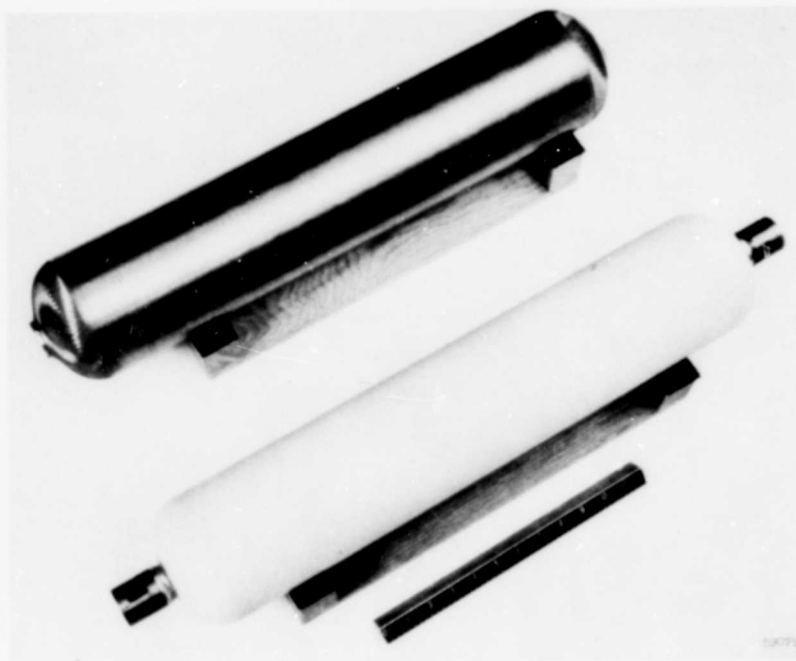
Fig. 1 - A mandrel (below), and finished, cured bottle (above)
