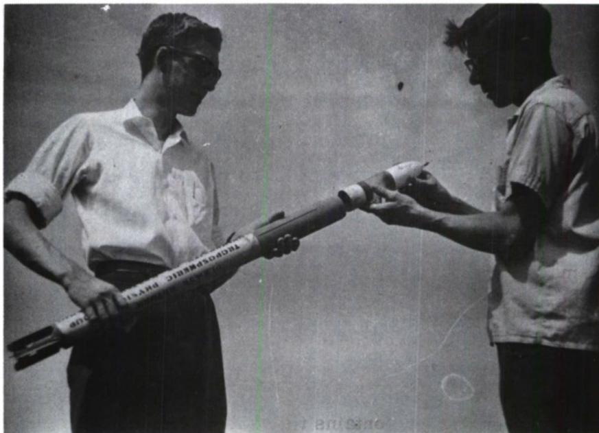
Fig. 2. Fitting the Nose Cone on the Rocket Vehicle
