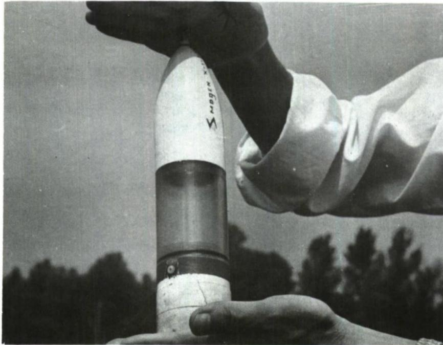
Fig. 3. Smoke-Generating Nose Cone
