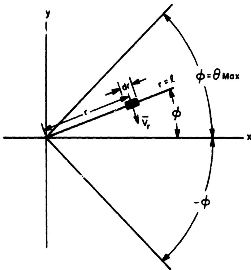
Figure D-1 Geometry for Wire Oscillating in a plane perpendicular to the Earth's Magnetic Field
