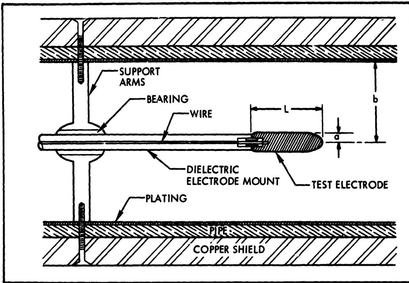
Figure 3 Cross Sectional Detail of Simulator Test Section
