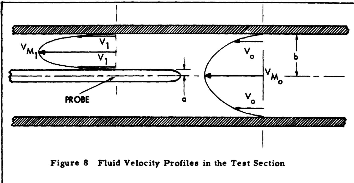
Figure 8 Fluid Velocity Profiles in the Test Section
