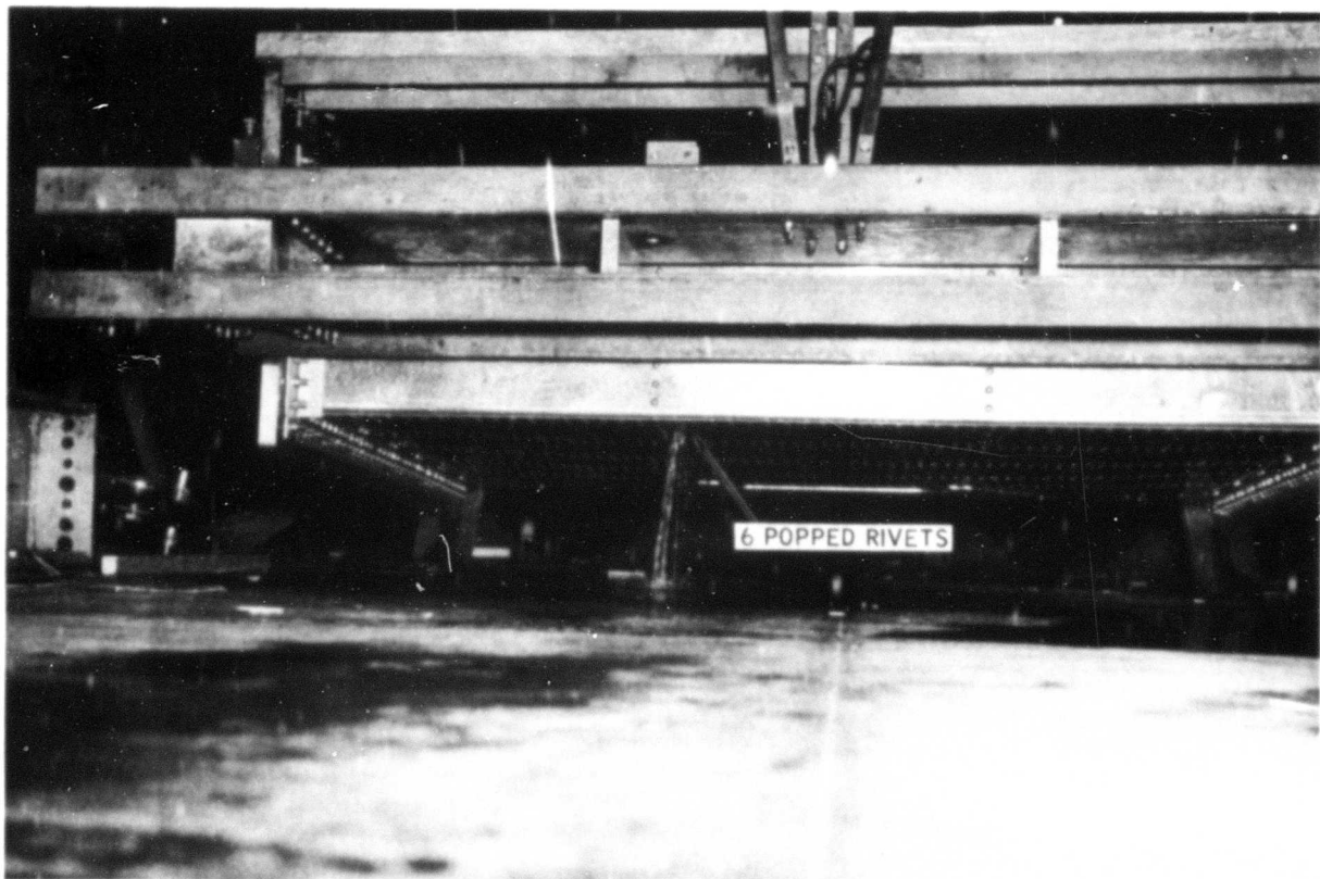
Figure B-20. External Damage to Test Tank No. 4. Tank was rebuilt from Tank No. 3. Steel rivets were added internally and skin doublers were added to the upper and lower surfaces (Figure B-24). Six rivets popped during Drop No. 18 — a 40-g arrested stop.
