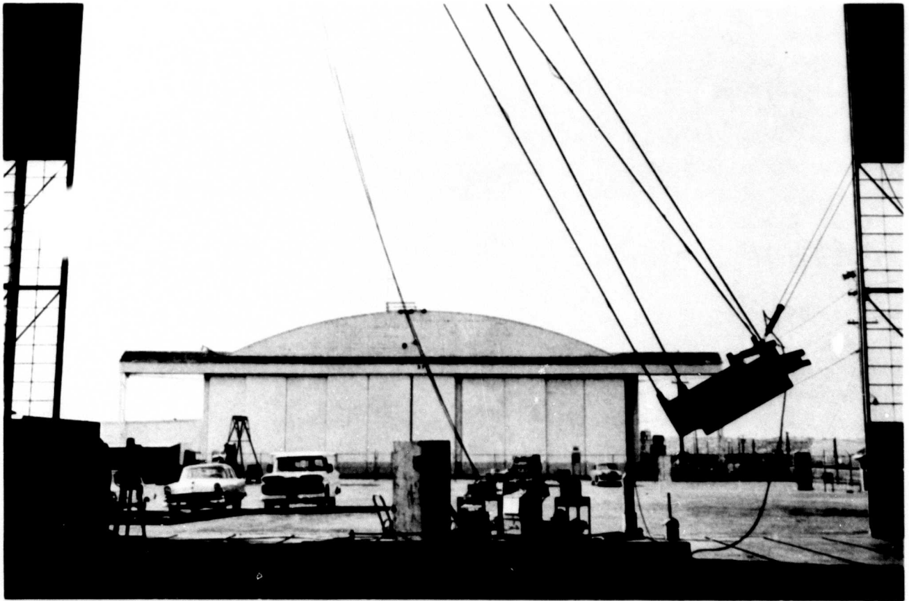
Figure B-2. Swing Test Setup. Tank specimens were suspended by 50-ft. straps. Specimens were arrested by stainless steel straps or were impacted against a log, pole, or sand.
