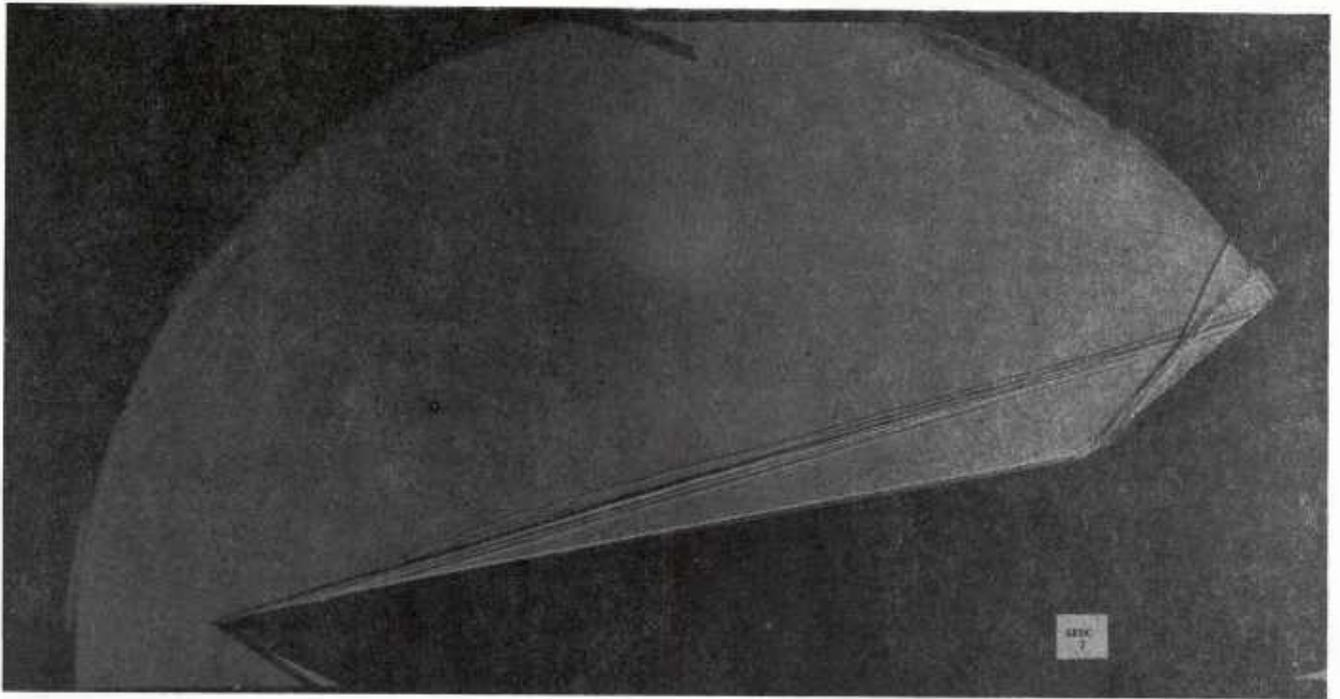
Fig. 27 Shadowgraph Flow Photograph; Ramp On, Maximum Coolant Flow Rate,  $\alpha = -10^\circ$ ,  $Re_\infty/\text{ft} = 3,300,000$
