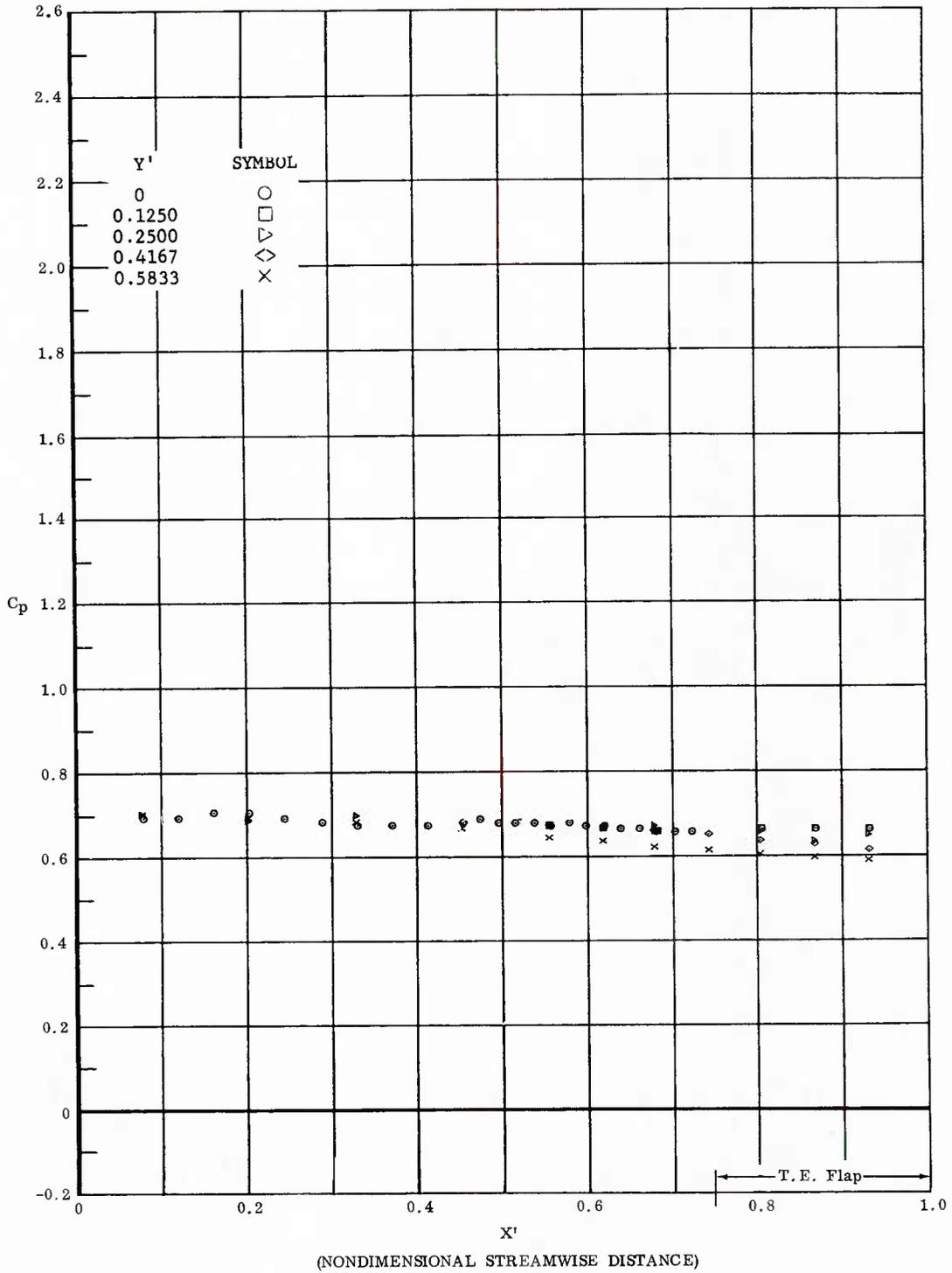
Fig. 72 Streamwise Pressure Distributions; Ramp Off, No Coolant Flow,
