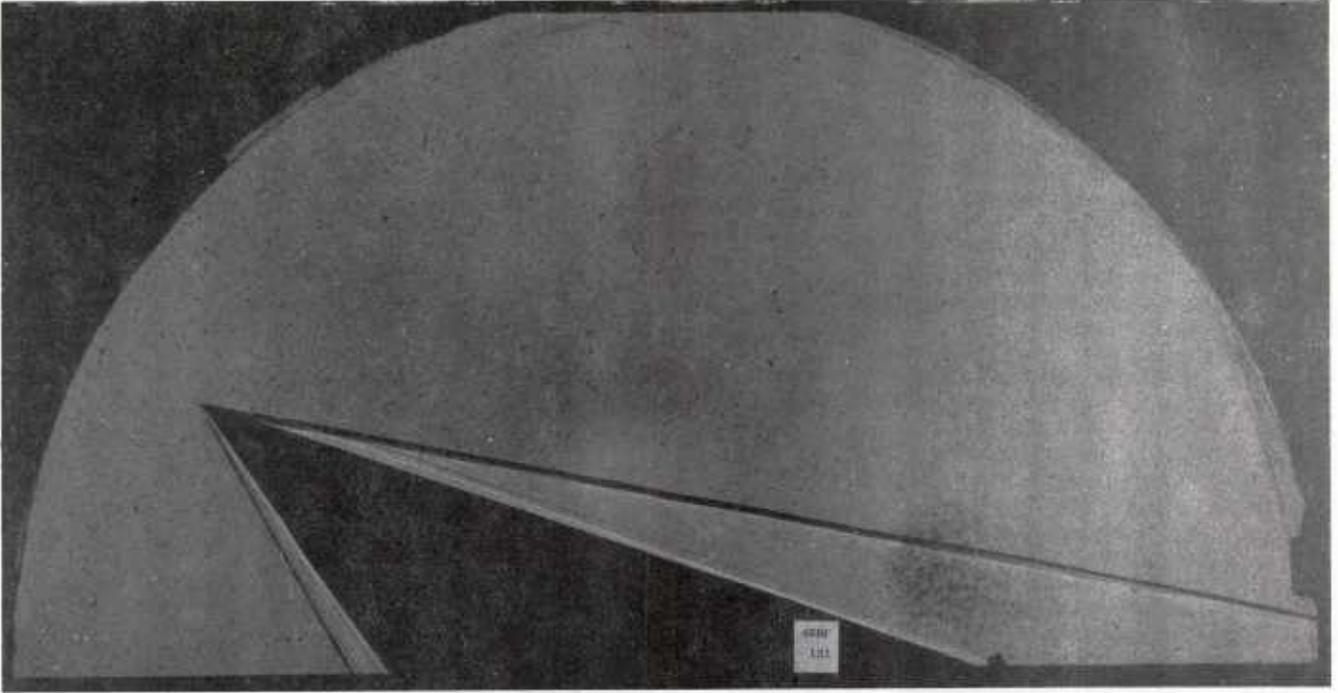
Fig. 11 Shadowgraph Flow Photograph; Ramp Off, No Coolant Flow,
