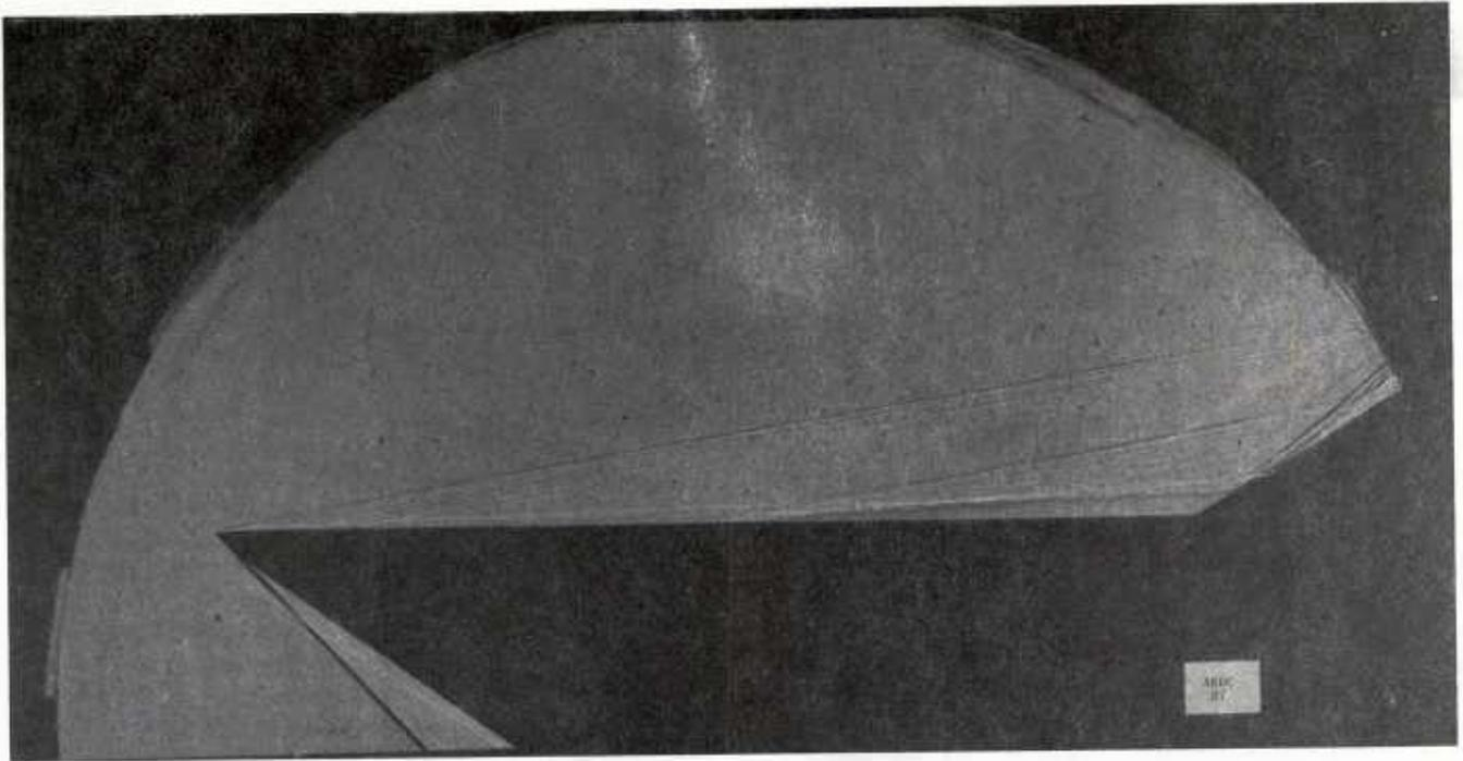
Fig. 47 Shadowgraph Flow Photograph; Ramp On, No Coolant Flow,
