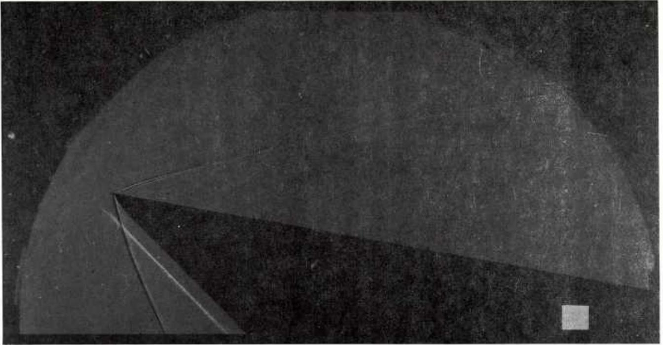
Fig. 57 Shadowgraph Flow Photograph; Ramp Off, No Coolant Flow,  $\alpha = +10^\circ$ ,  $Re_\infty/\text{ft} = 1,100,000$
