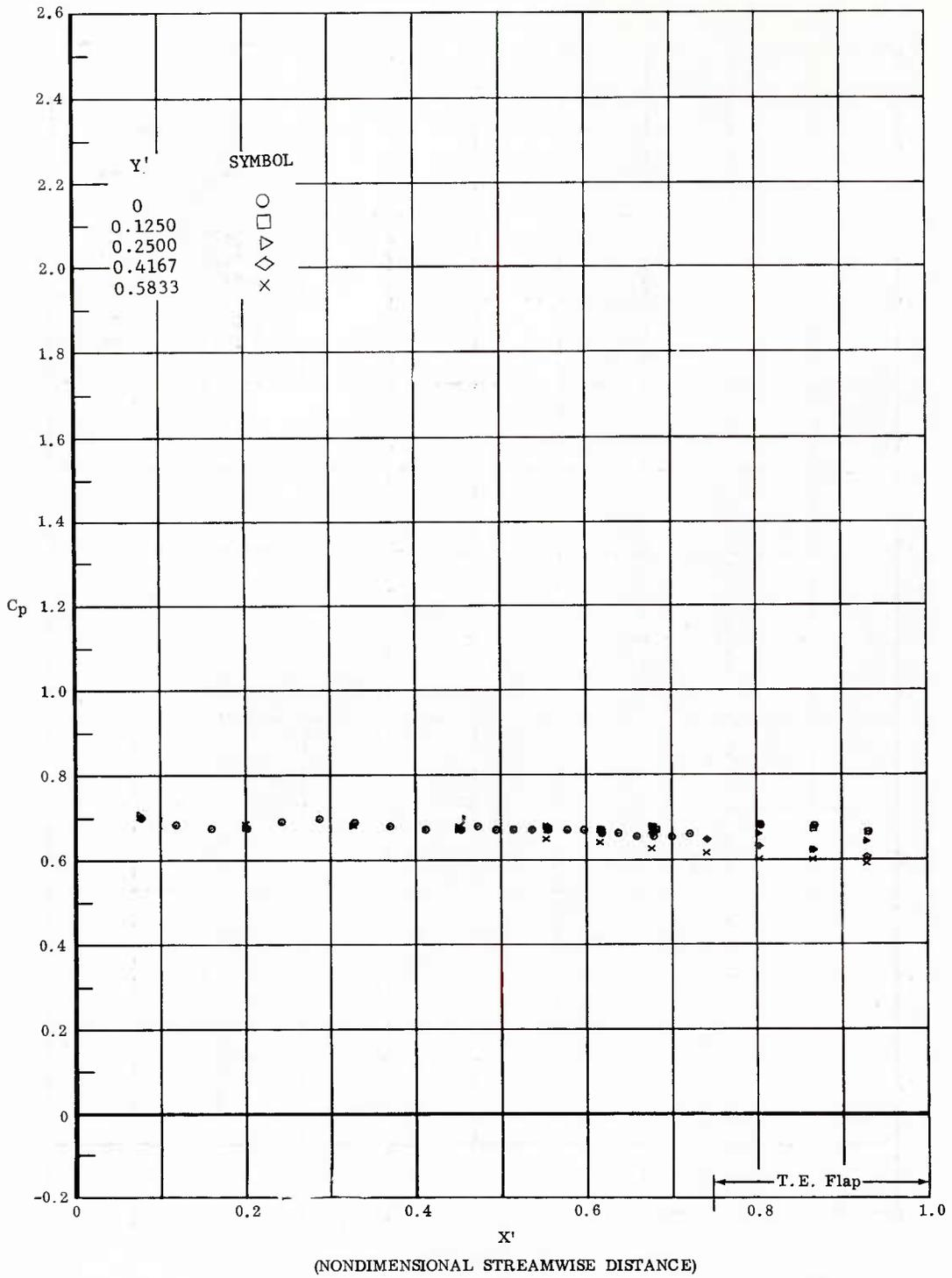
Fig. 73 Streamwise Pressure Distributions; Ramp Off, No Coolant Flow,
