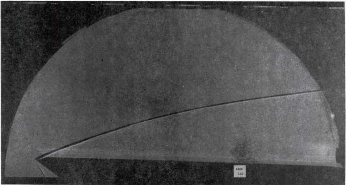
Fig. 6 Shadowgraph Flow Photograph; Ramp off, Maximum Coolant Flow Rate,  $\alpha = -43^\circ$ ,  $Re_\infty/ft = 3,300,000$
