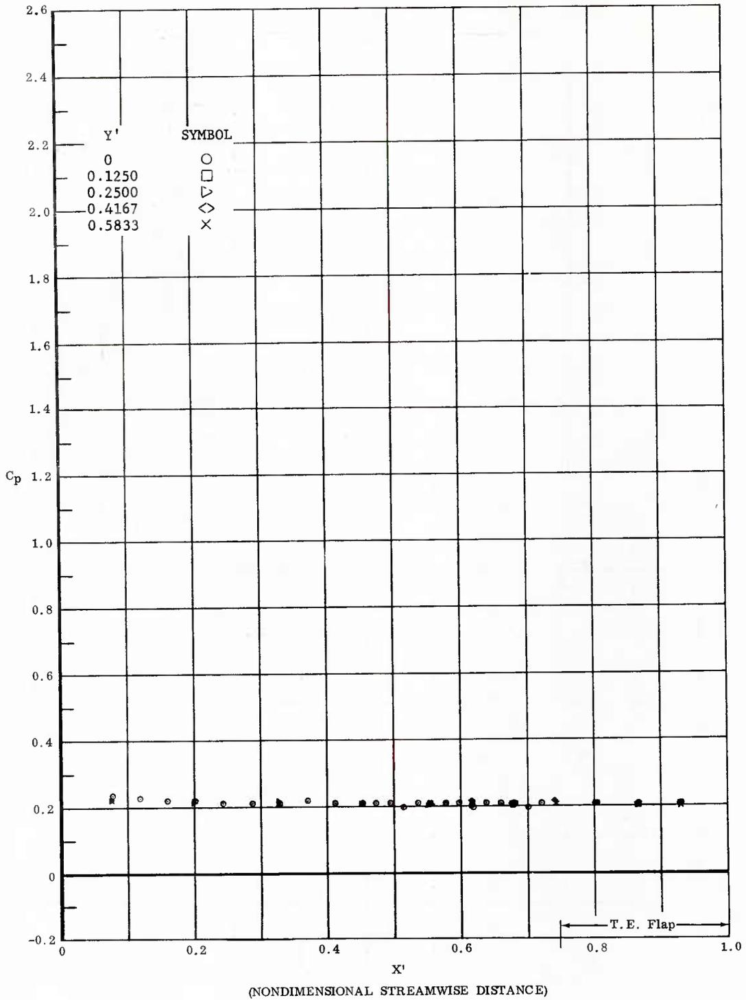
Fig. 81 Streamwise Pressure Distributions; Ramp Off, No Coolant Flow,
