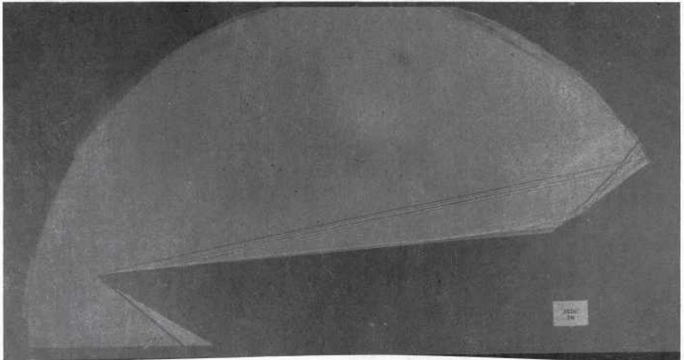
Fig. 34 Shadowgraph Flow Photograph; Ramp On, No Coolant Flow,  $\alpha = -5^\circ$ ,  $Re_\infty/\text{ft} = 3,300,000$
