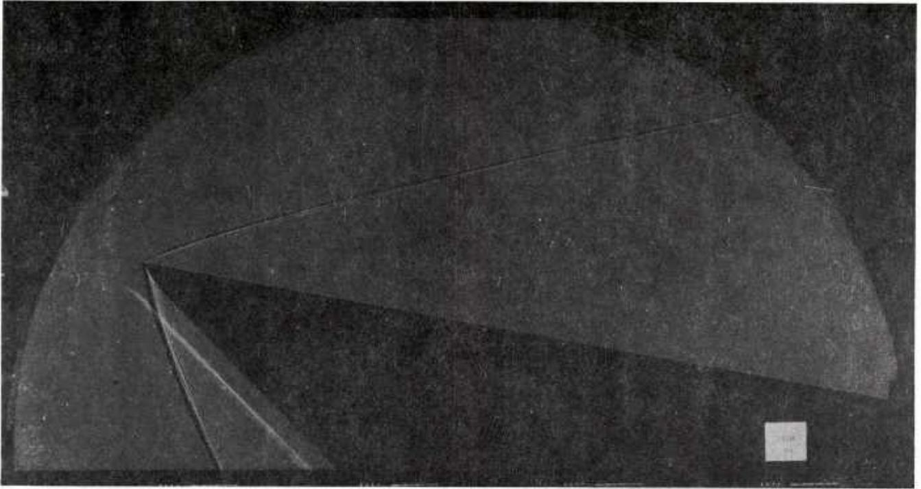
Fig. 59 Shadowgraph Flow Photograph; Ramp Off, No Coolant Flow,
