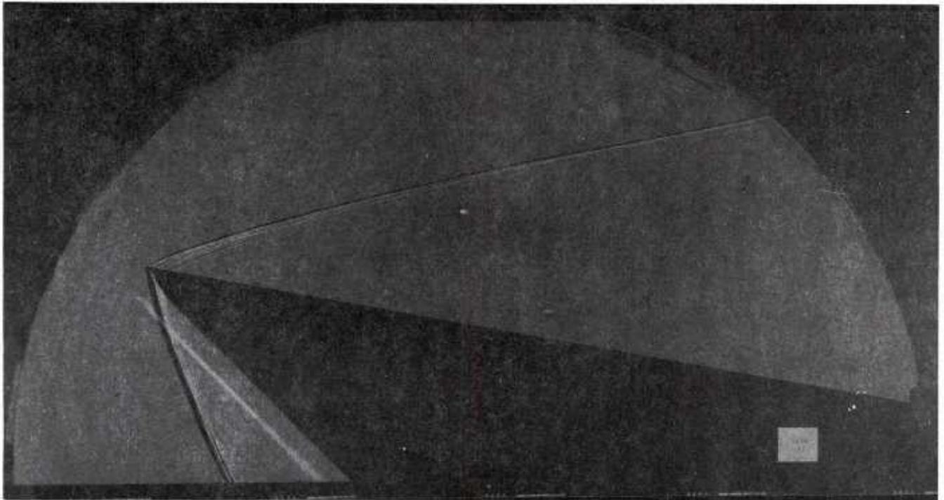
Fig. 60 Shadowgraph Flow Photograph; Ramp Off, No Coolant Flow,
