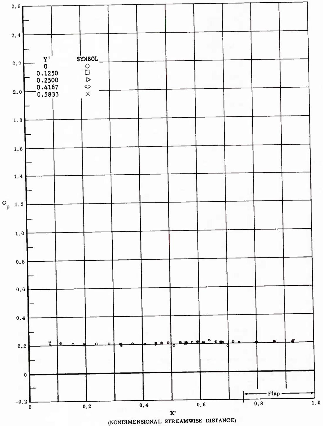
Fig. 83 Streamwise Pressure Distributions; Ramp Off, Maximum Coolant Flow Rate,  $\alpha = -15^\circ$ ,  $Re_\infty/ft = 3,300,000$ .
