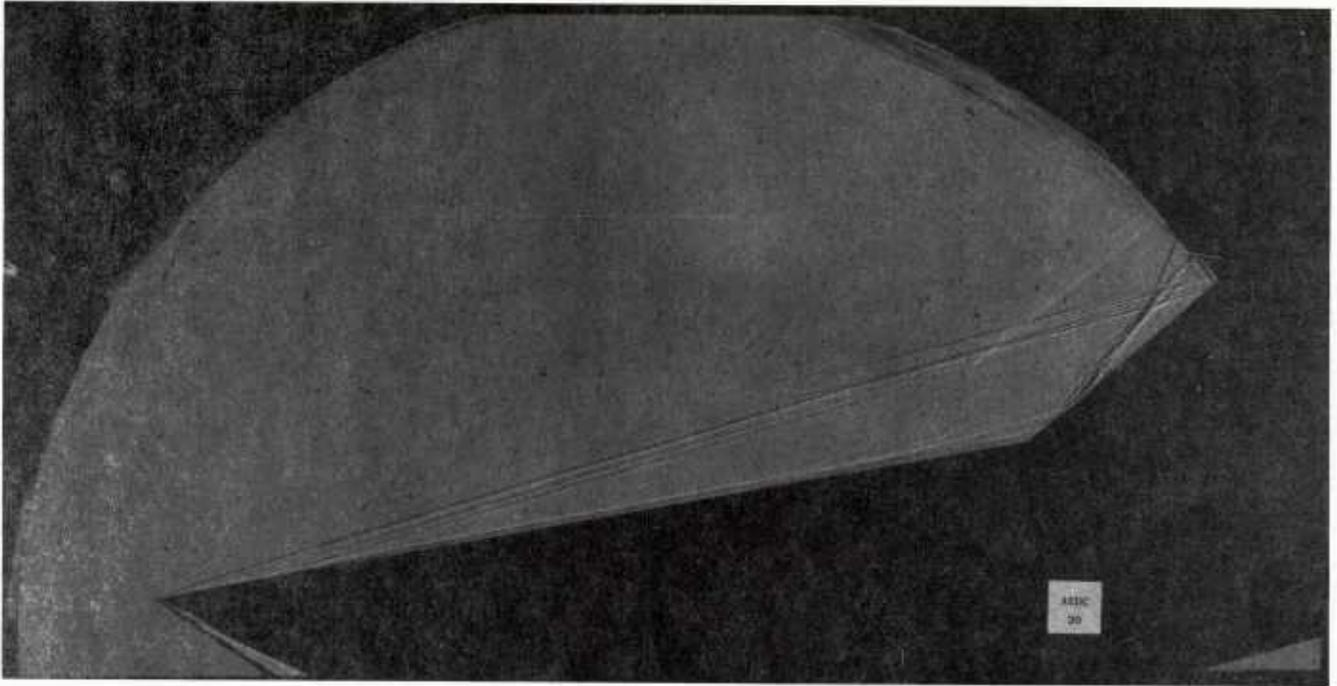
Fig. 25 Shadowgraph Flow Photograph; Ramp On, Maximum Coolant Flow Rate,  $\alpha = -10^\circ$ ,  $Re_\infty/\text{ft} = 1,100,000$
