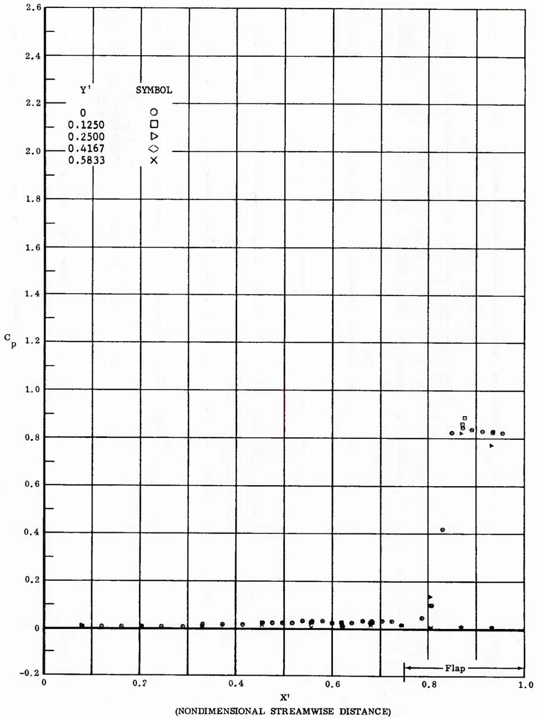
Fig. 113 Streamwise Pressure Distributions; Ramp On, No Coolant Flow,
