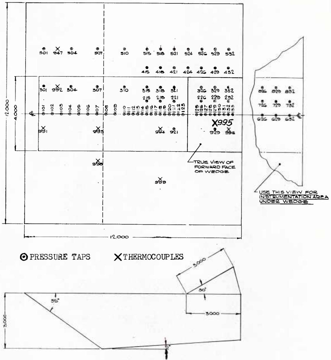
Fig. 4 Model Instrumentation
