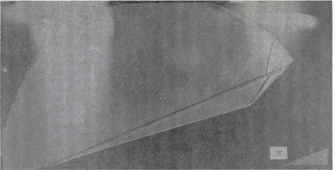
Fig. 19 Shadowgraph Flow Photograph; Ramp On, No Coolant Flow,
