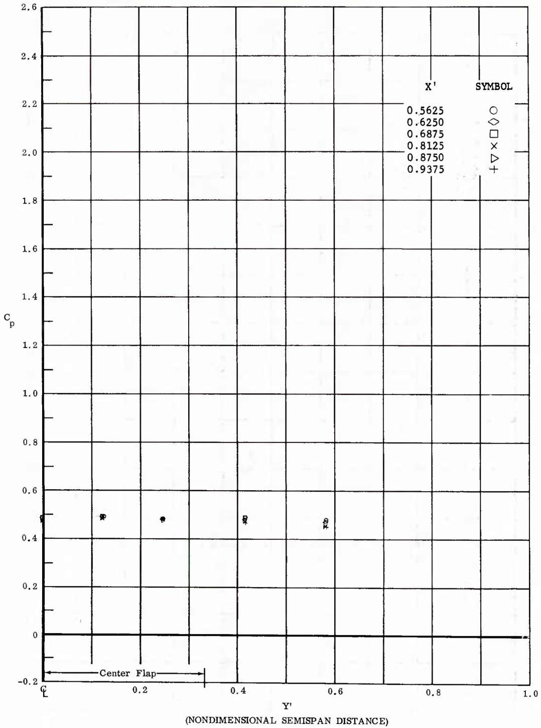
Fig. 75 Spanwise Pressure Distributions; Ramp Off, No Coolant Flow,
