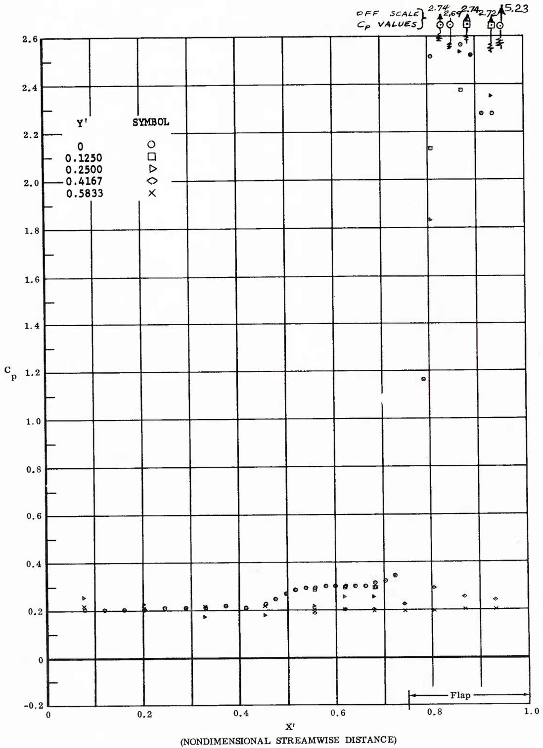
Fig. 84 Streamwise Pressure Distributions; Ramp On, Maximum Coolant Flow Rate,  $\alpha = -15^\circ$ ,  $Re_\infty / ft = 1,100,000$ .
