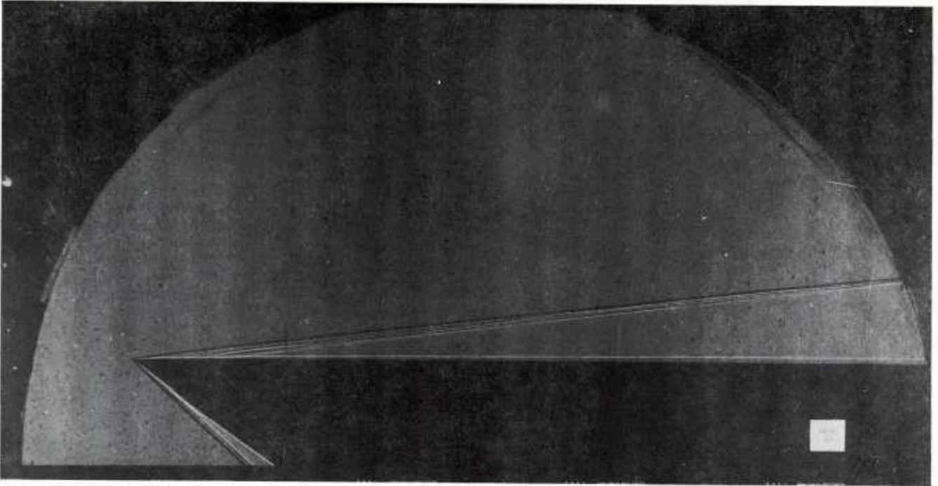
Fig. 13 Shadowgraph Flow Photograph; Ramp Off, No Coolant Flow,
