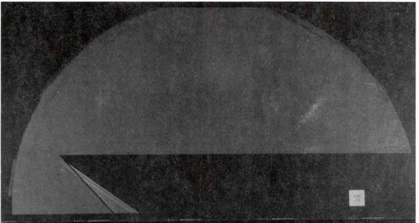
Fig. 36 Shadowgraph Flow Photograph, Ramp Off, No Coolant Flow,  $\alpha = 0$ ,  $Re_{\infty}/ft = 1,100,000$
