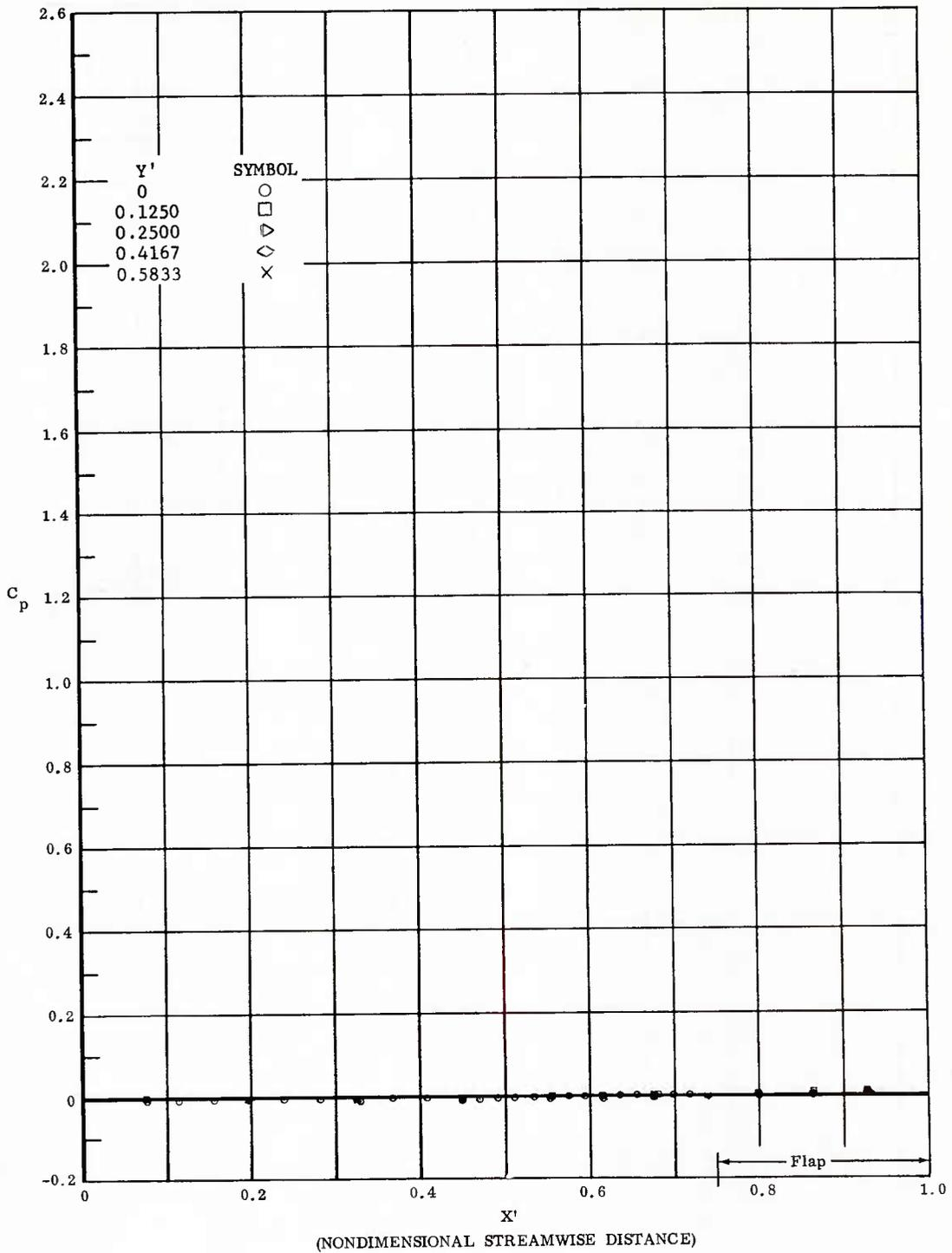
Fig. 118 Streamwise Pressure Distributions; Ramp Off, Maximum Coolant Flow Rate,  $\alpha = +5^\circ$ ,  $Re_\infty/ft = 3,300,000$ .
