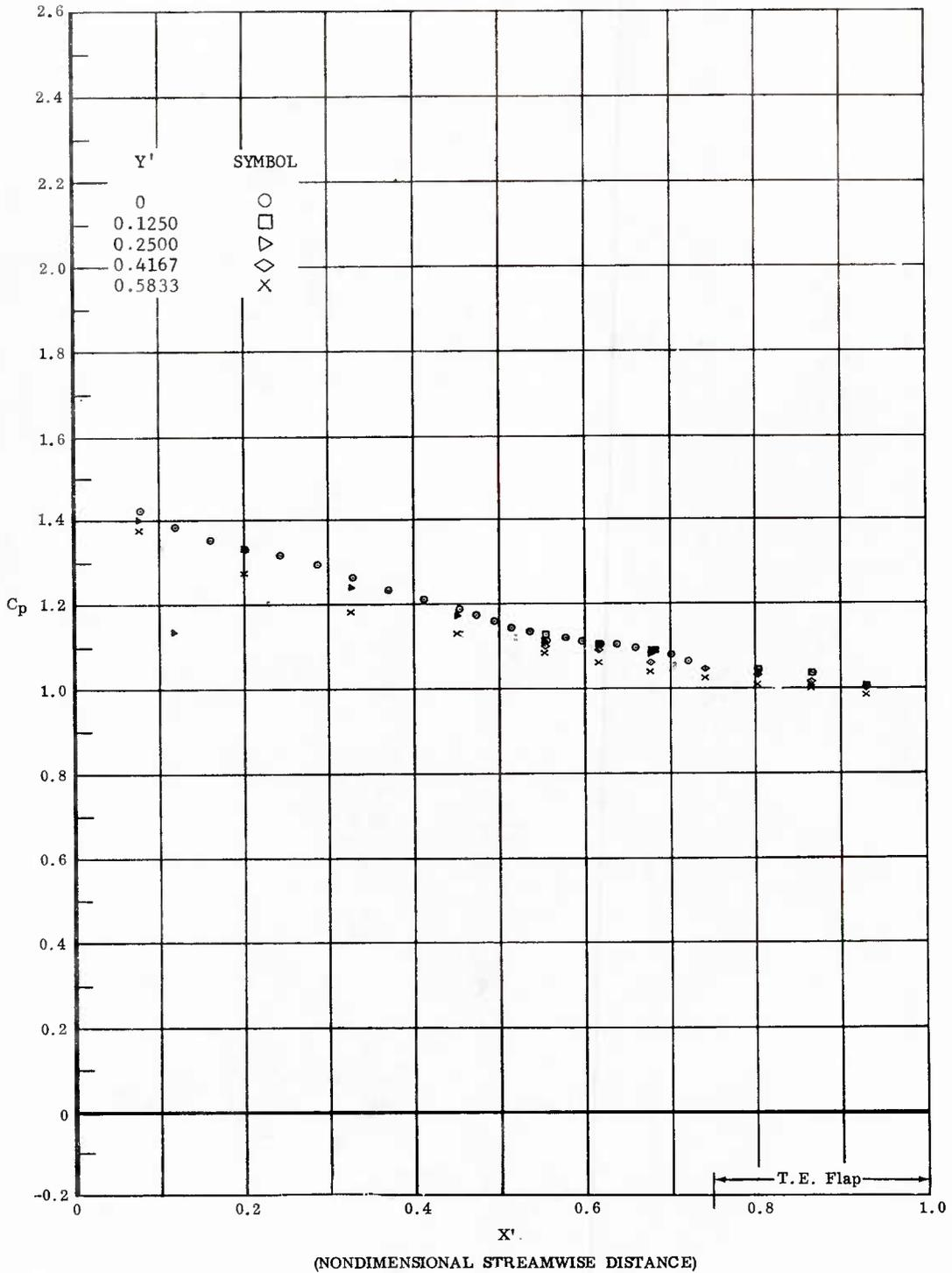
Fig. 65 Streamwise Pressure Distributions; Ramp Off, No Coolant Flow,  $\alpha = -43^\circ$ ,  $Re_{c}/ft = 3,300,000$ .
