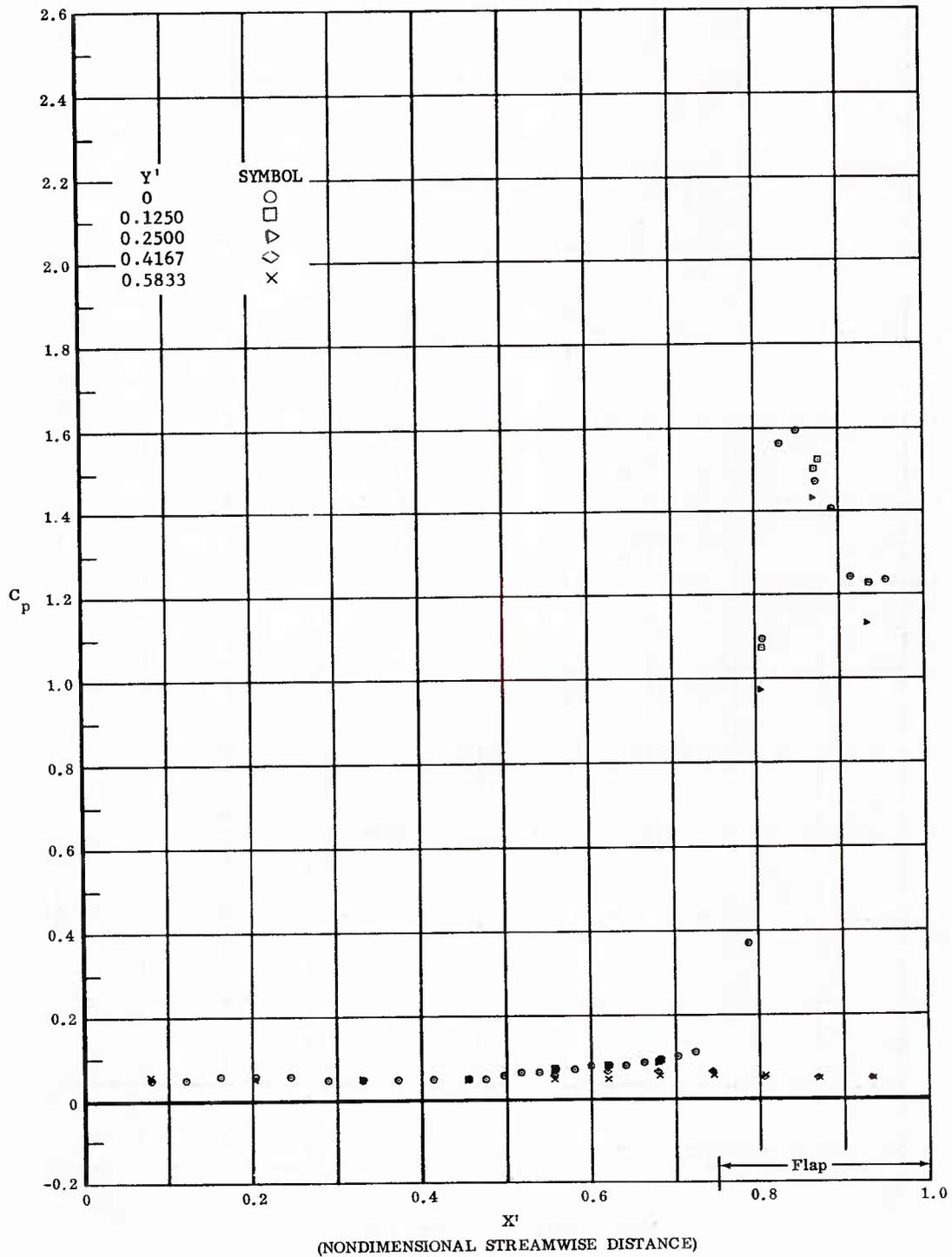
Fig. 100 Streamwise Pressure Distributions; Ramp On, No Coolant Flow,
