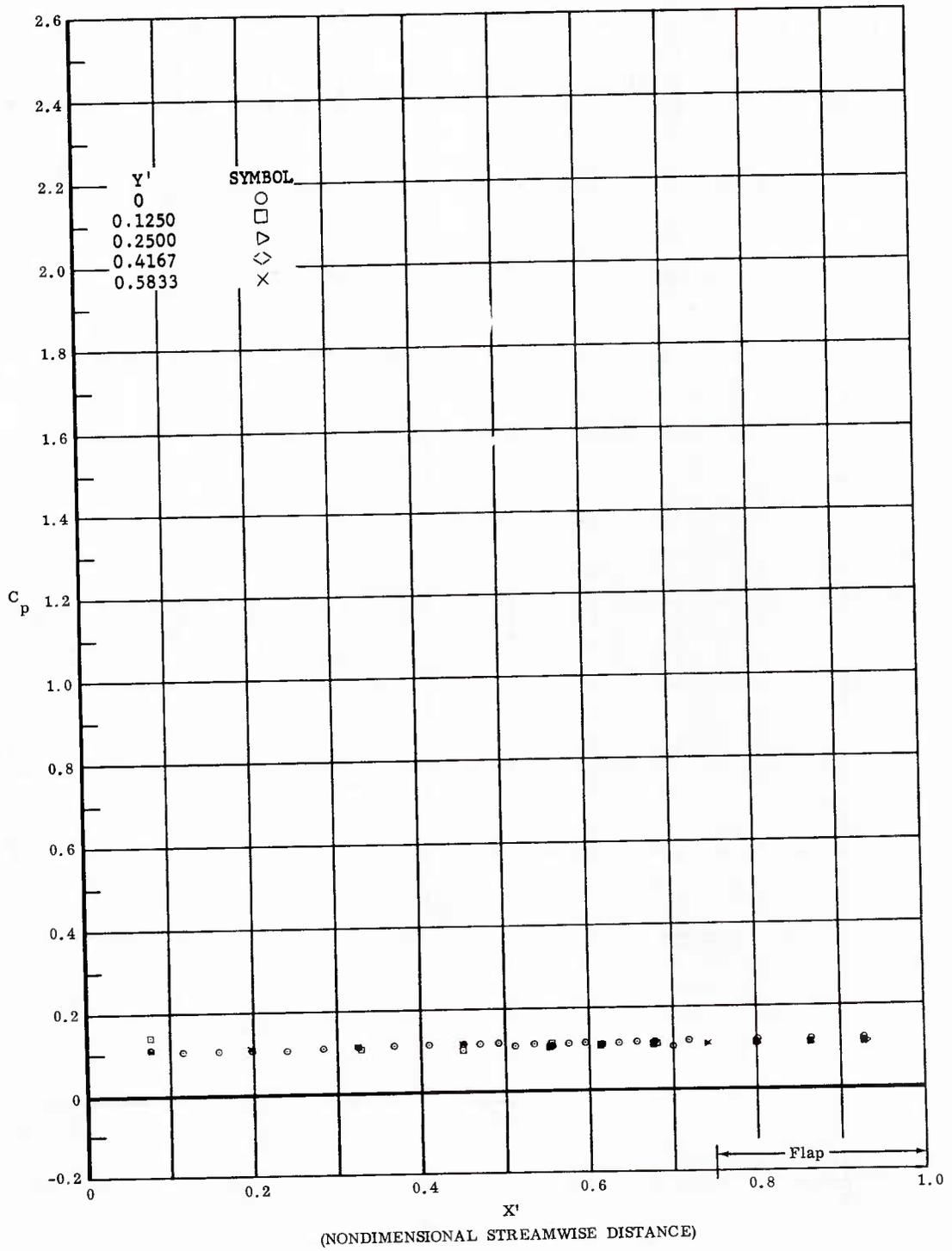
Fig. 90 Streamwise Pressure Distributions; Ramp Off, Maximum Coolant Flow Rate,  $\alpha = -10^\circ$ ,  $Re_\infty / ft = 3,300,000$ .
