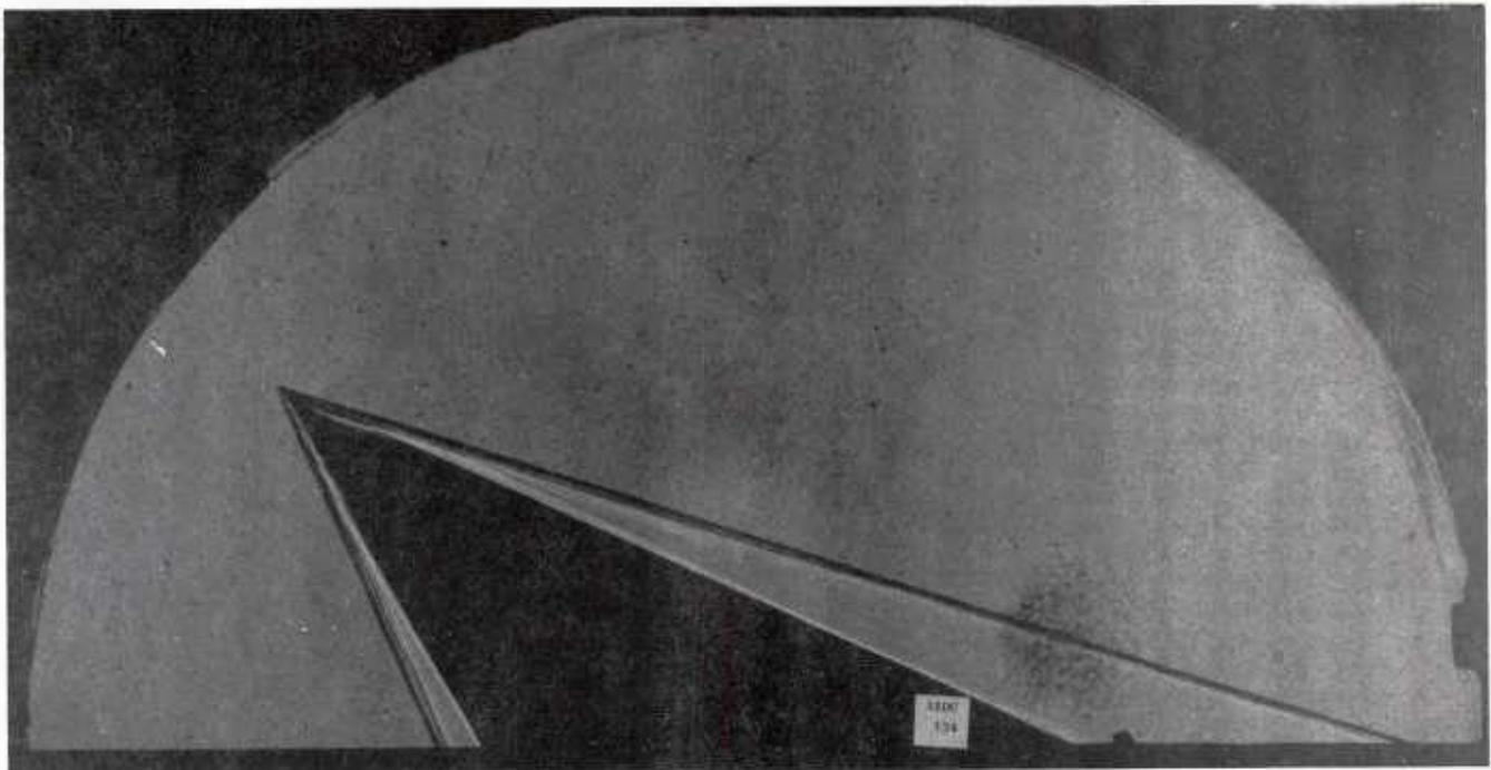
Fig. 12 Shadowgraph Flow Photograph; Ramp Off, No Coolant Flow,
