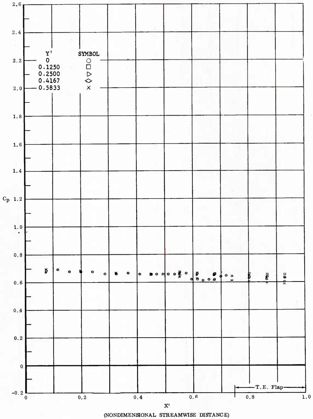
Fig. 71 Streamwise Pressure Distributions; Ramp Off, No Coolant Flow,
