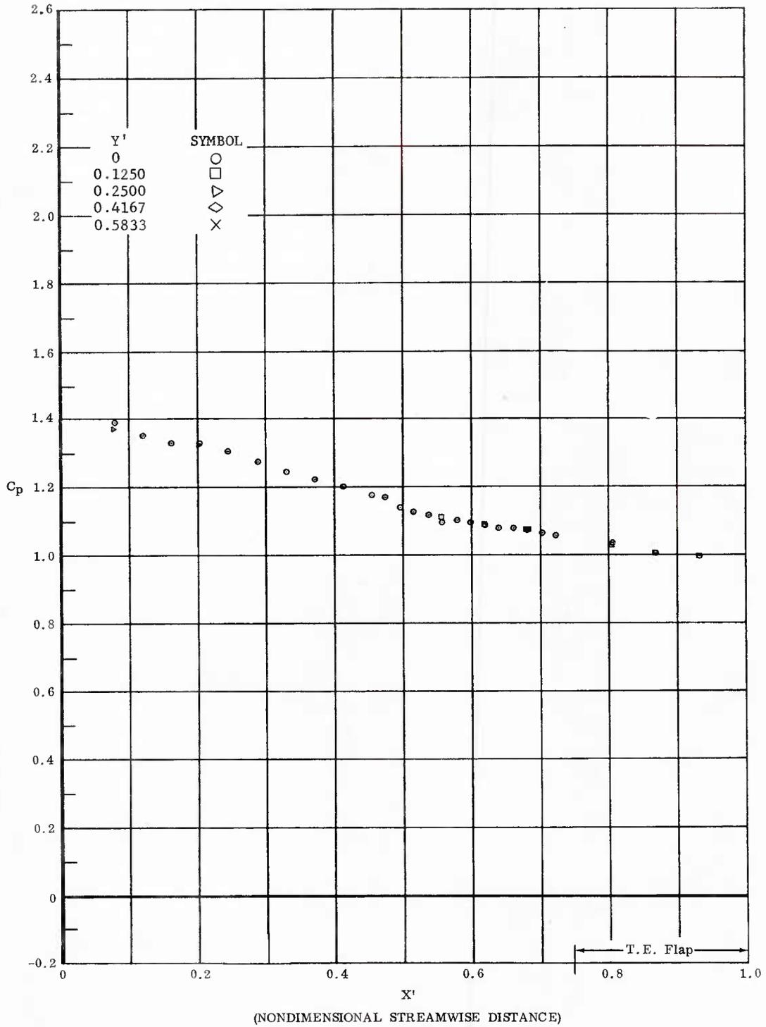
Fig. 64 Streamwise Pressure Distributions; Ramp Off, No Coolant Flow,
