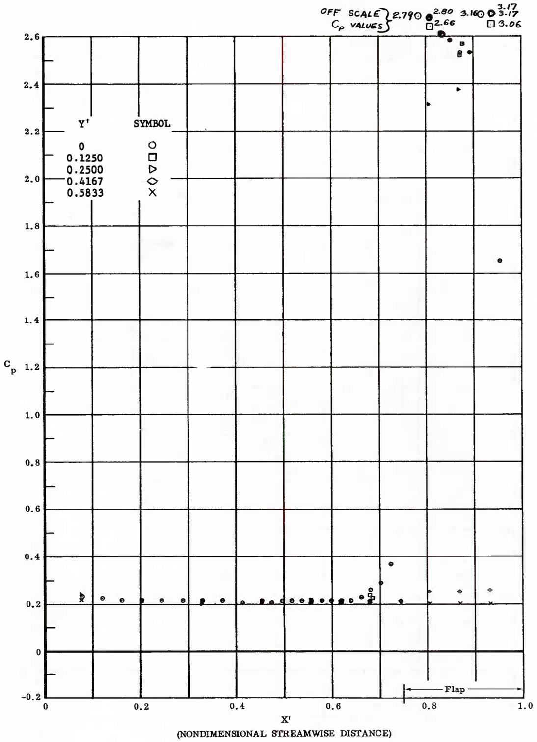
Fig. 86 Streamwise Pressure Distributions; Ramp On, Maximum Coolant Flow Rate,  $\alpha = -15^\circ$ ,  $Re_{\infty}/ft = 3,300,000$ .
