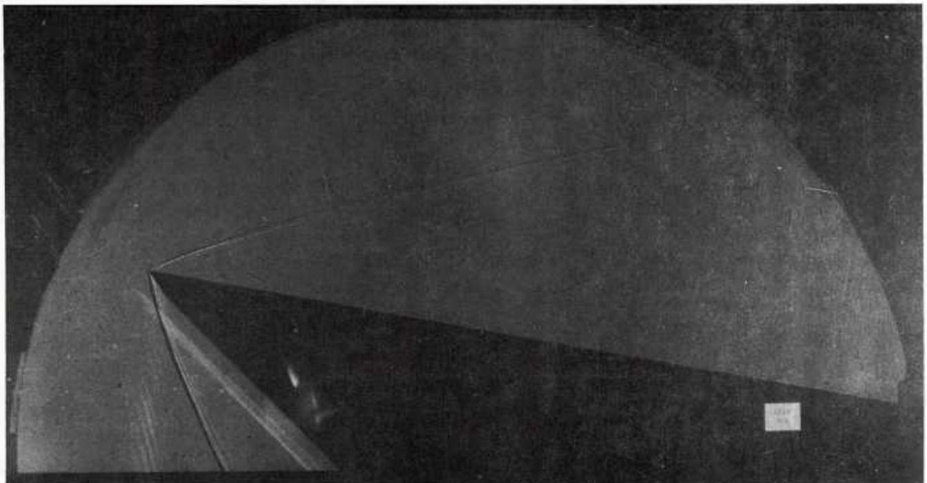
Fig. 58 Shadowgraph Flow Photograph; Ramp Off, Maximum Coolant Flow Rate,  $\alpha = +10^\circ$ ,  $Re_\infty/\text{ft} = 1,100,000$
