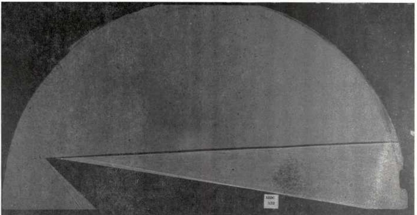
Fig. 8 Shadowgraph Flow Photograph; Ramp Off, No Coolant Flow,
