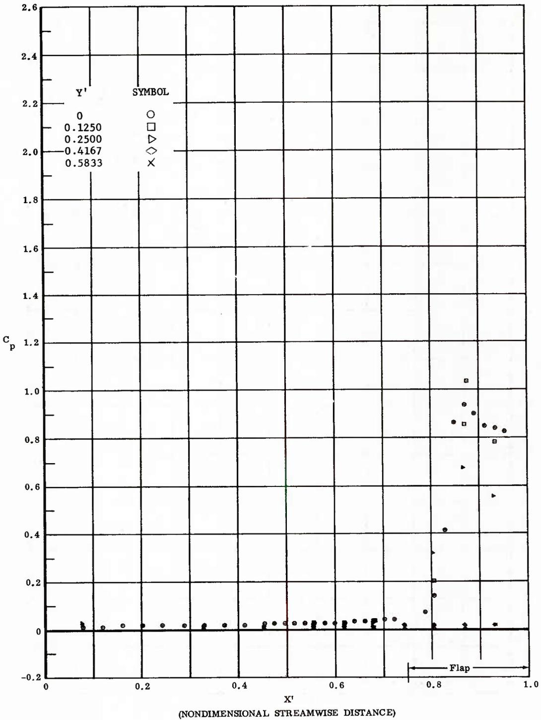
Fig. 114 Streamwise Pressure Distributions; Ramp On, Maximum Coolant Flow Rate,  $\alpha = 0^\circ$ ,  $Re_\infty/ft = 3,300,000$ .
