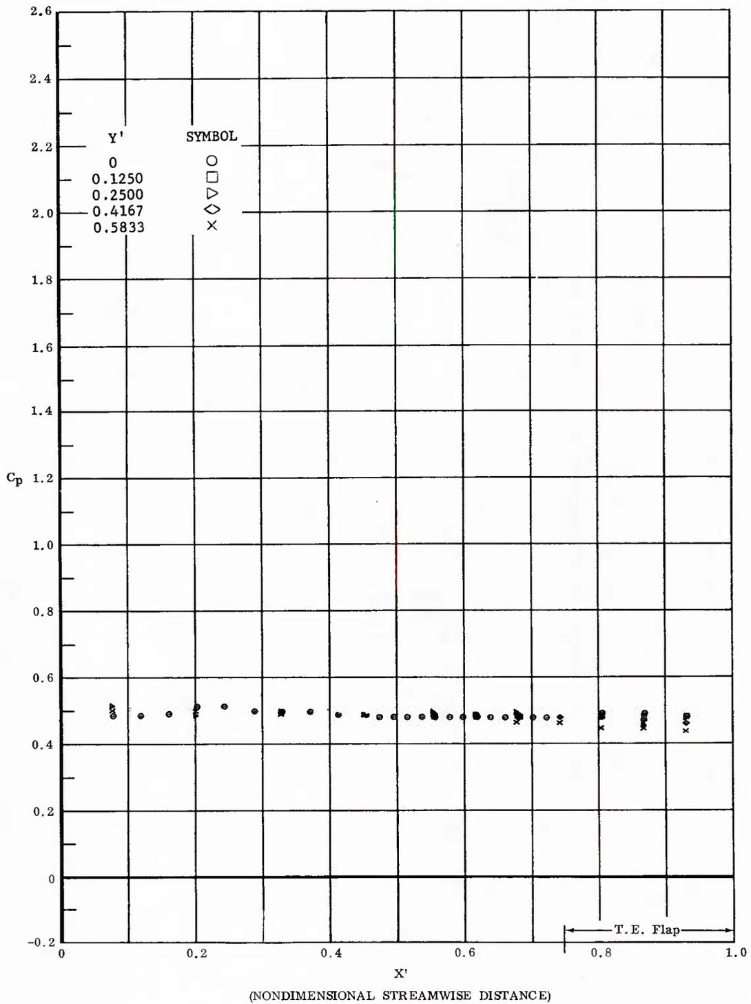
Fig. 76 Streamwise Pressure Distributions; Ramp Off, No Coolant Flow,
