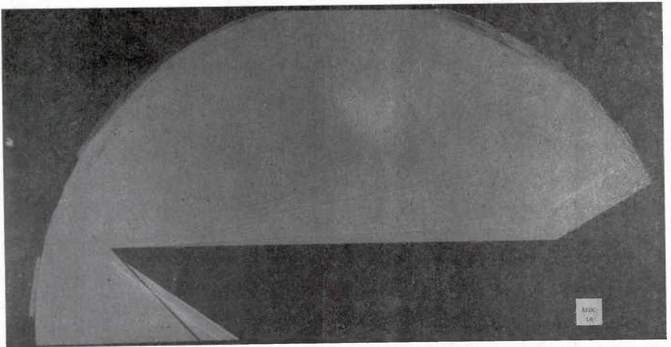
Fig. 44 Shadowgraph Flow Photograph; Ramp On, Maximum Coolant
