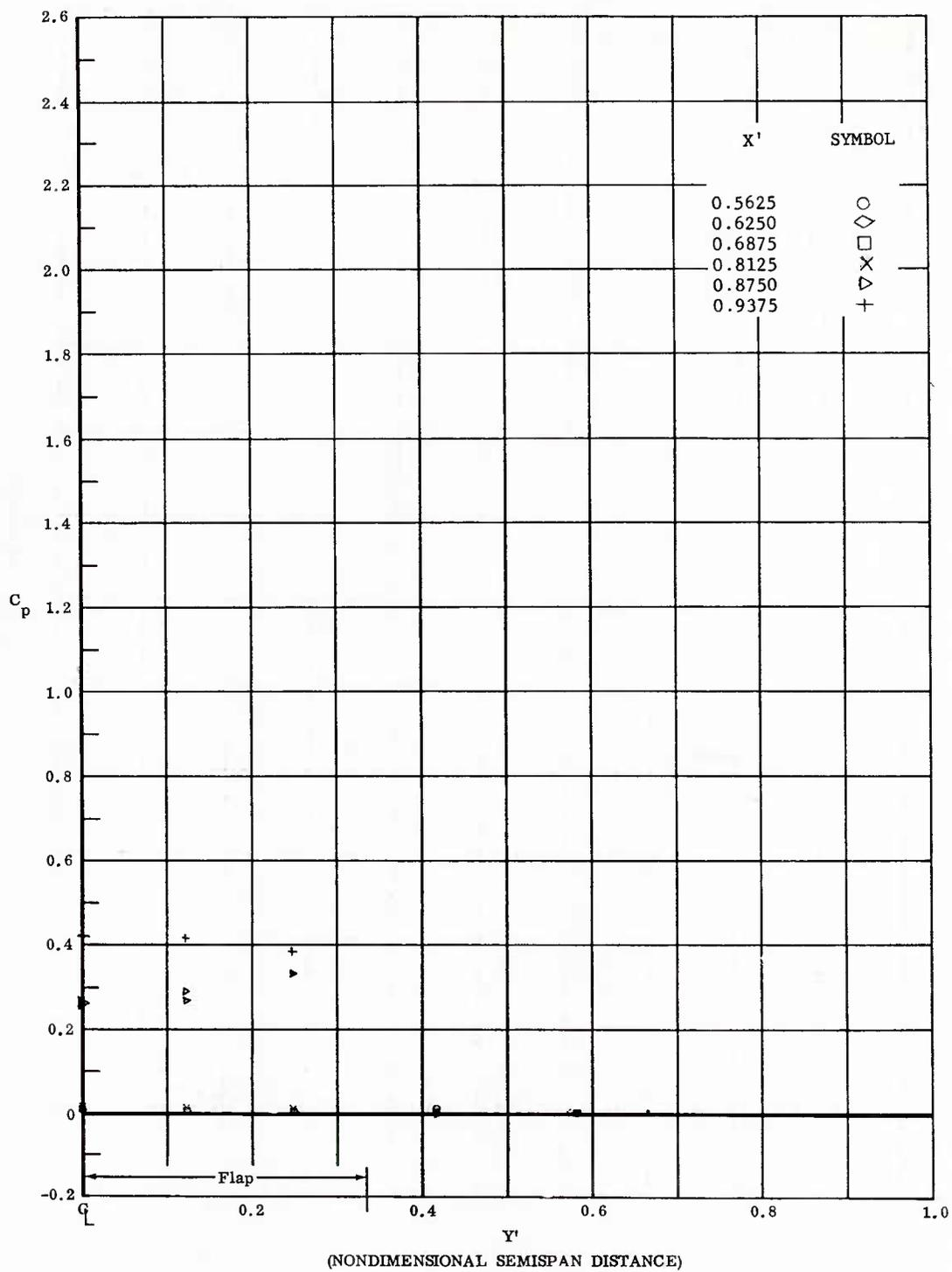
Fig. 121 Spanwise Pressure Distributions; Ramp On, No Coolant Flow,
