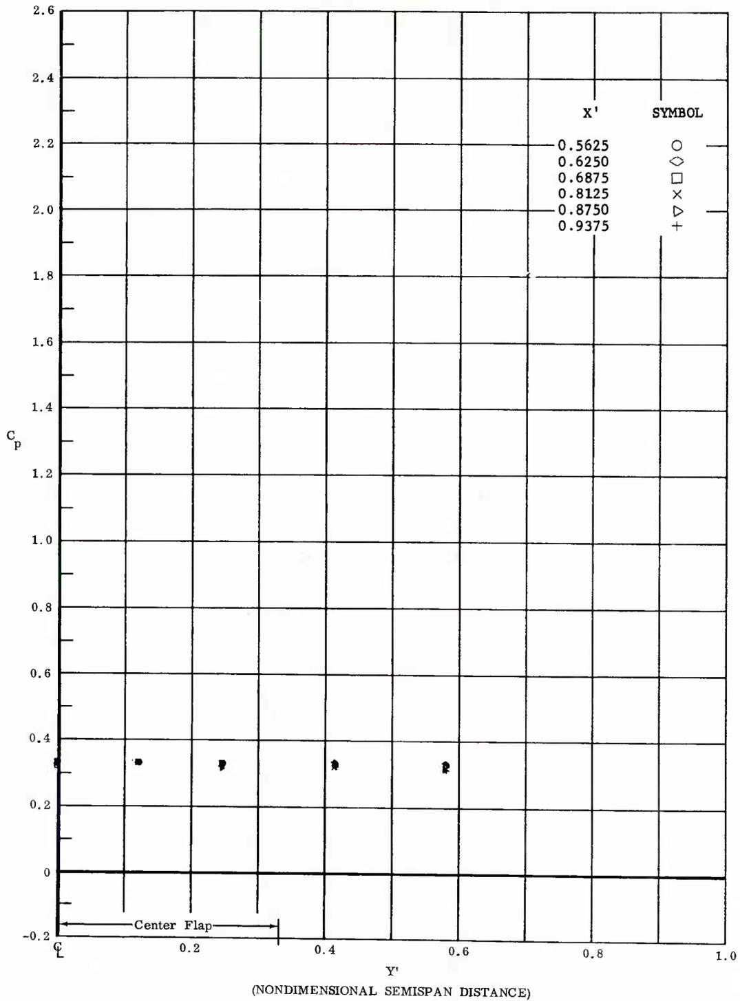
Fig. 78 Spanwise Pressure Distributions; Ramp Off, No Coolant Flow,  $\alpha = -20^\circ$ ,  $Re_\infty/\bar{c}t = 3,300,000$ .
