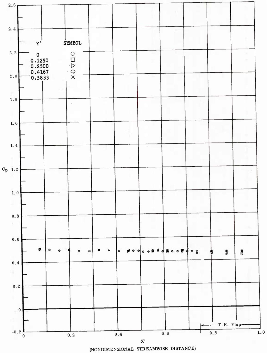
Fig. 75 Streamwise Pressure Distributions; Ramp Off, No Coolant Flow,
