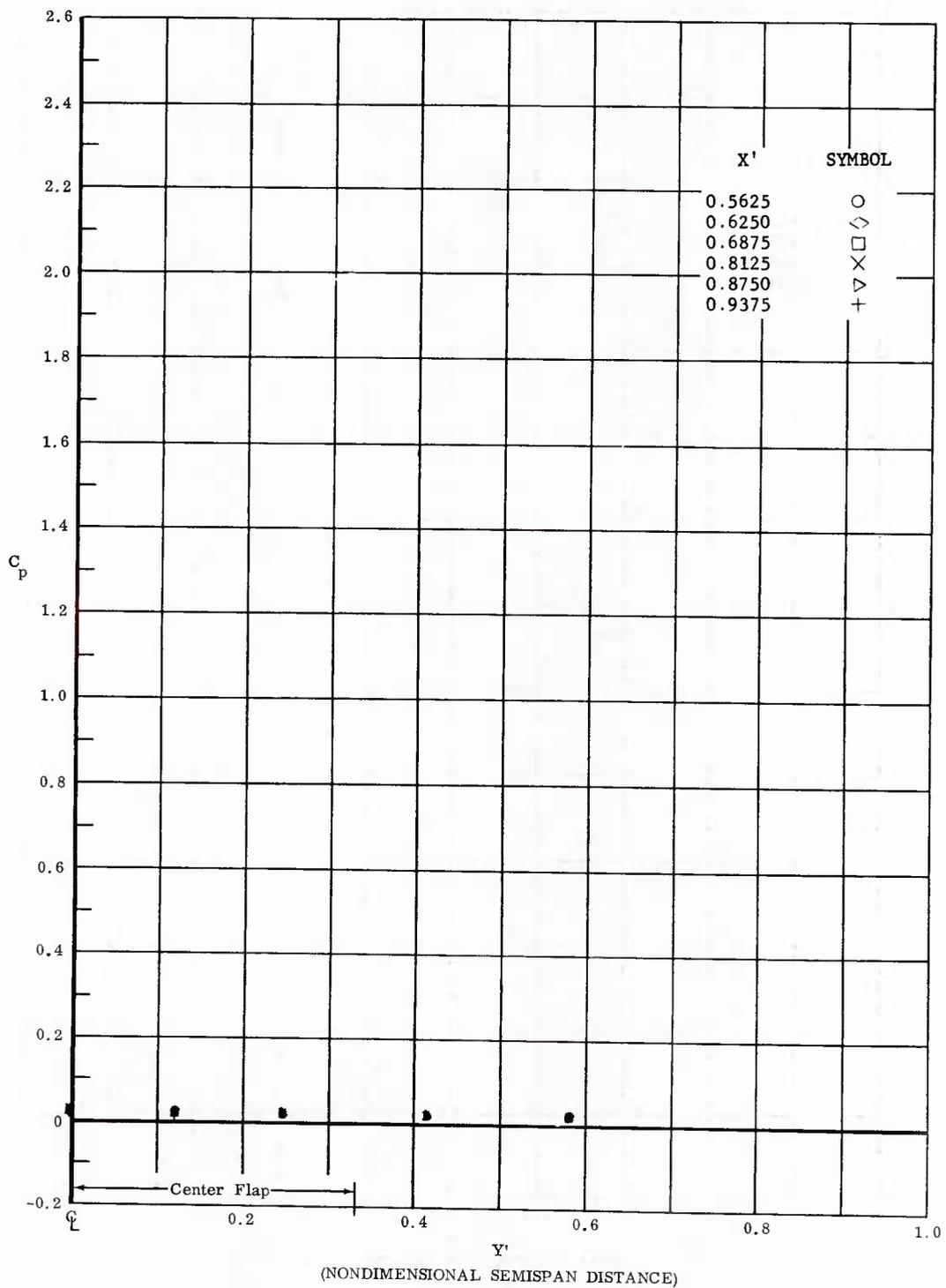
Fig. 106 Spanwise Pressure Distributions; Ramp Off, No Coolant Flow,
