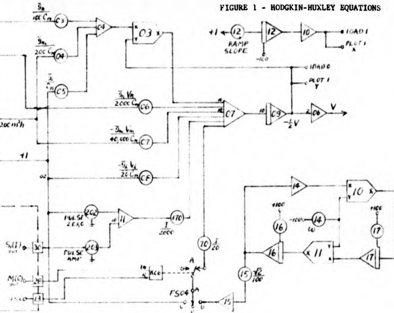
3. To set P 202 and P 203: adjust P 202 for 0V out of All in STANDBY;
