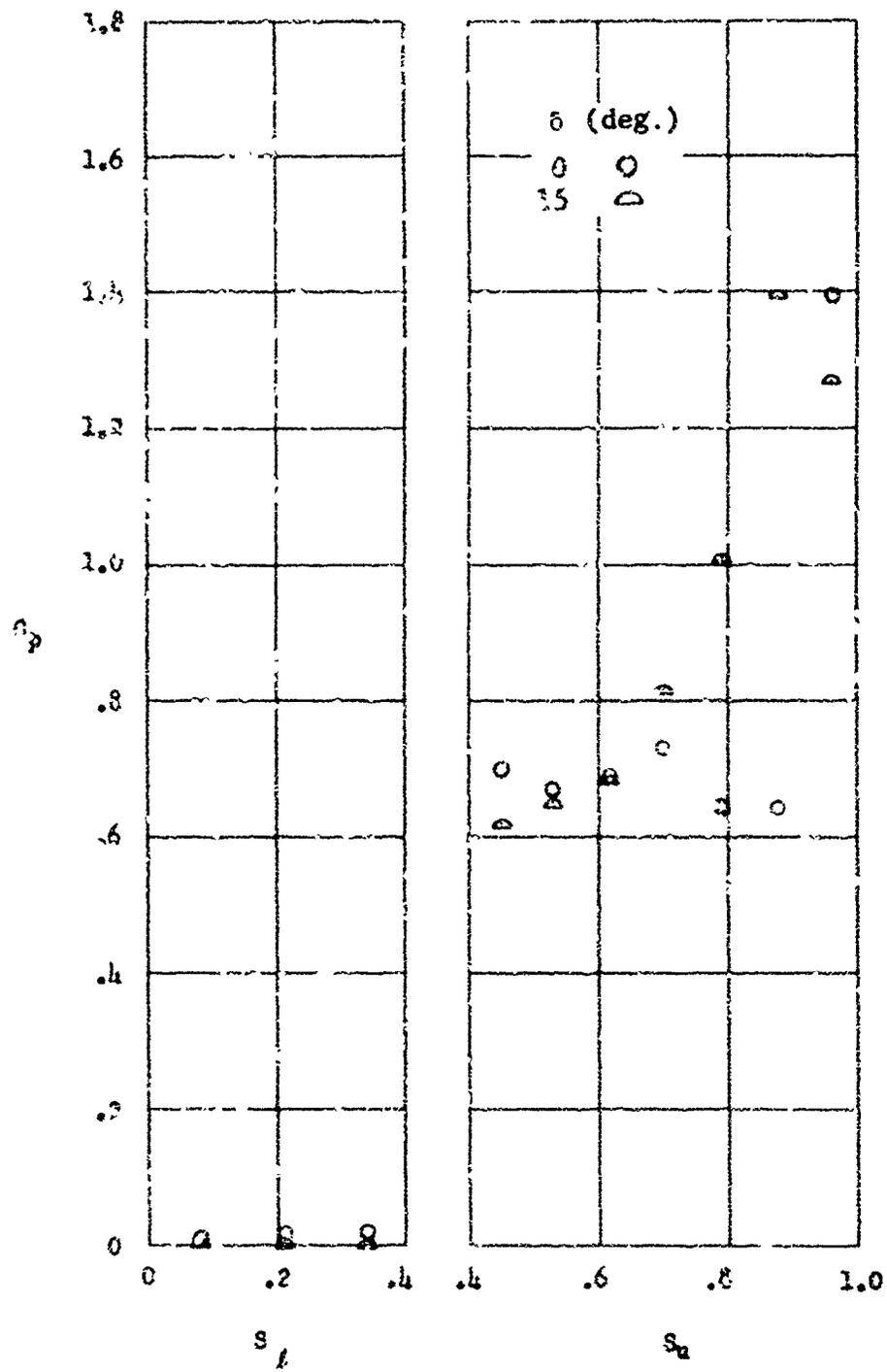
Fig. 14 Chordwise Pressure Distribution for Model A,  $M_\infty = 19$ ,  $\alpha = 30$
