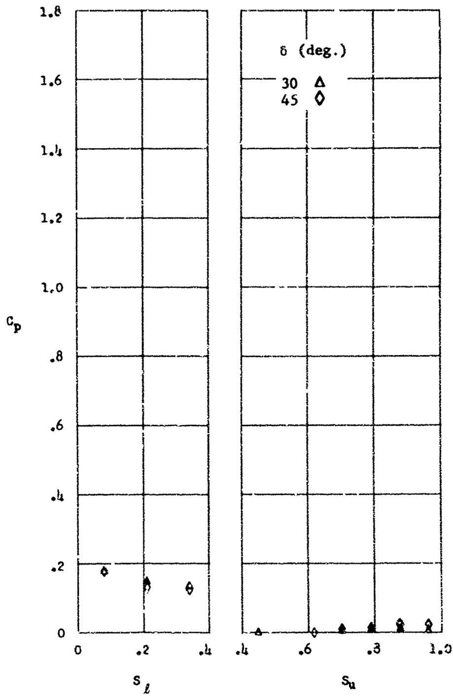
Fig. 10 Chordwise Pressure Distribution for Model A,  $M_\infty = 19$ ,  $\alpha = -10$
