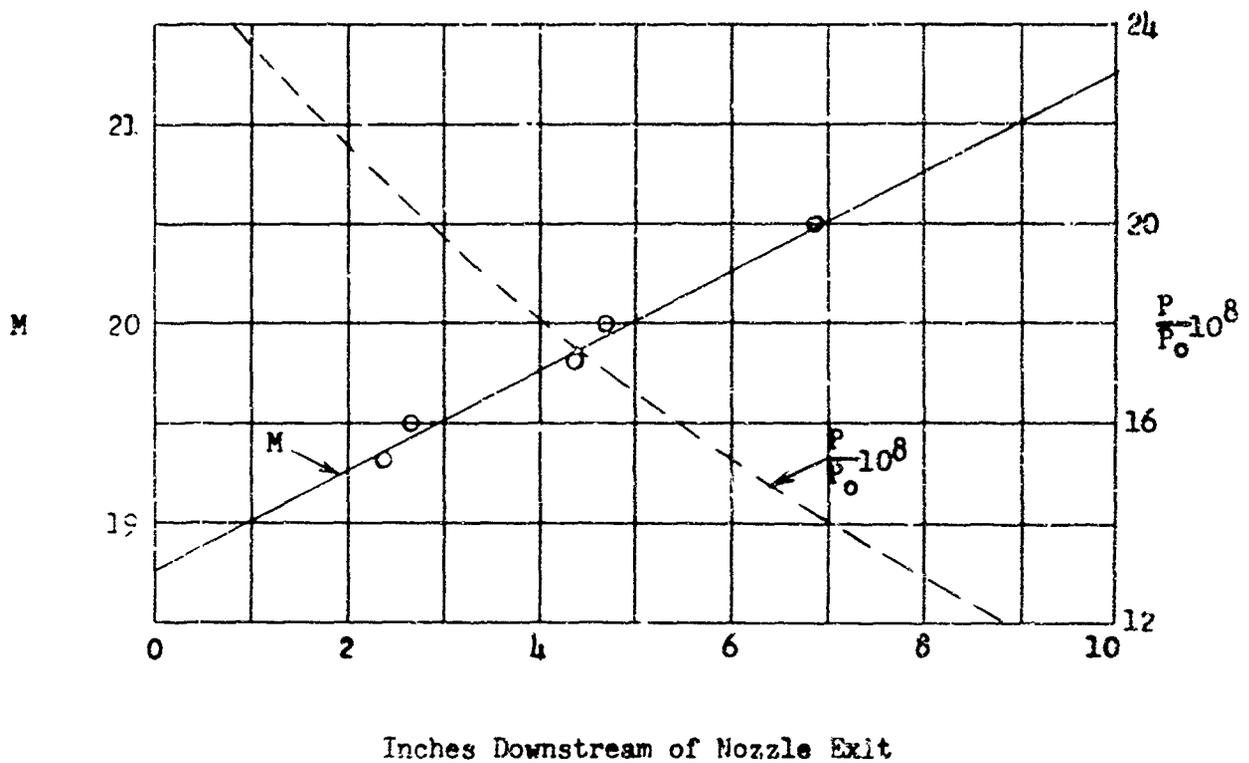
Fig. 6 Tunnel Centerline Distributions of Mach Number and Static to Total Pressure and Temperature Ratios for the M=19 Conditions
