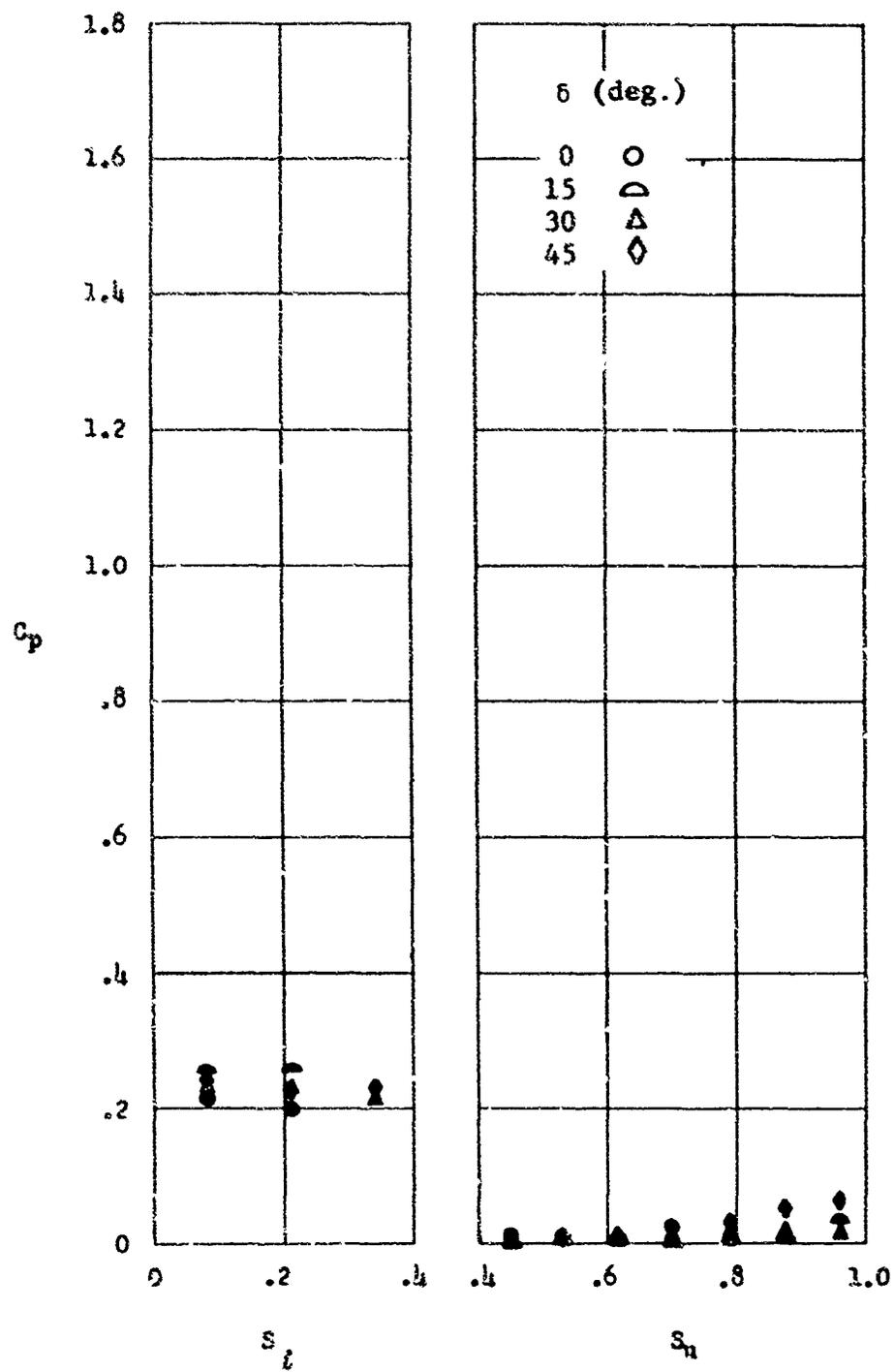
Fig. 9 Chordwise Pressure Distribution for Model A,  $M_\infty = 19$ ,  $\alpha = -15$
