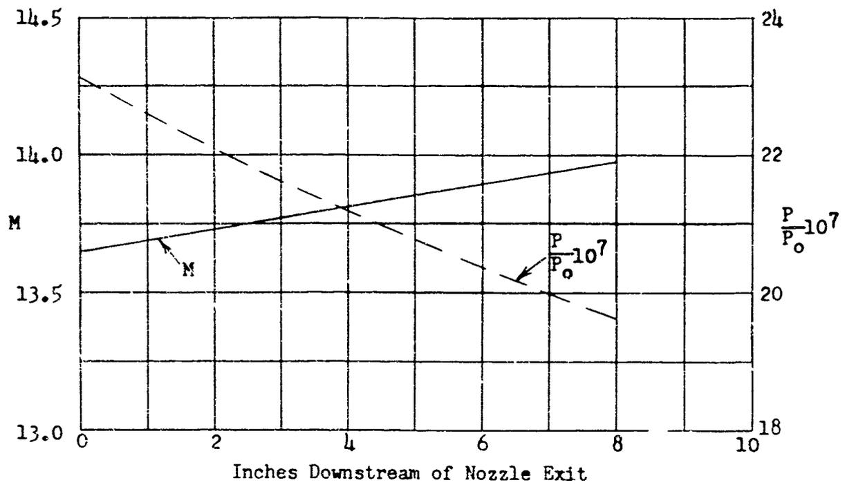
Fig. 5 Tunnel Centerline Distributions of Mach Number and Static to Total Pressure and Temperature Ratios for the M=13 Conditions
