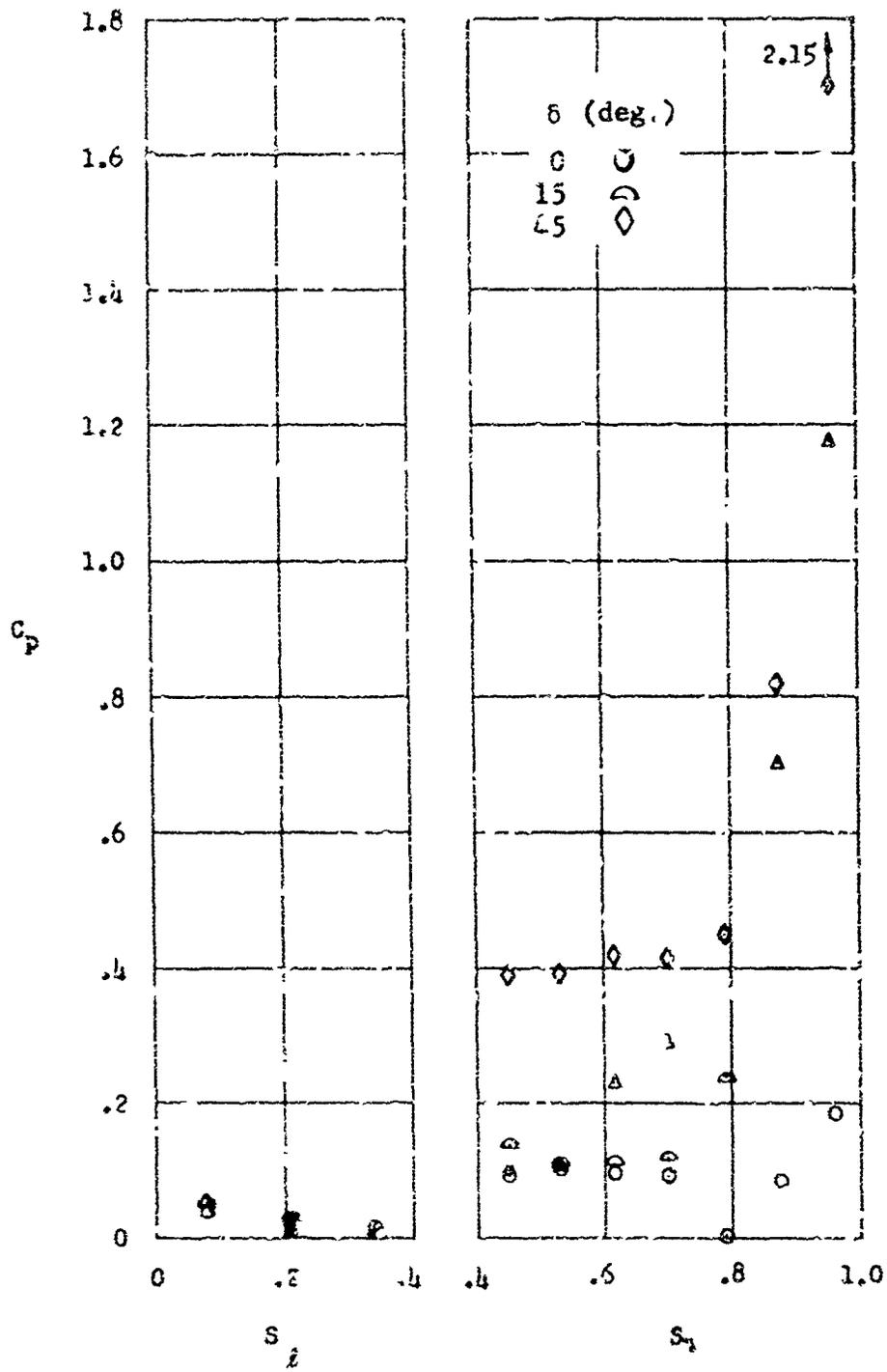
Fig. 13 Chordwise Pressure Distribution for Model A,  $M_\infty = 19$ ,  $\alpha = 10^\circ$
