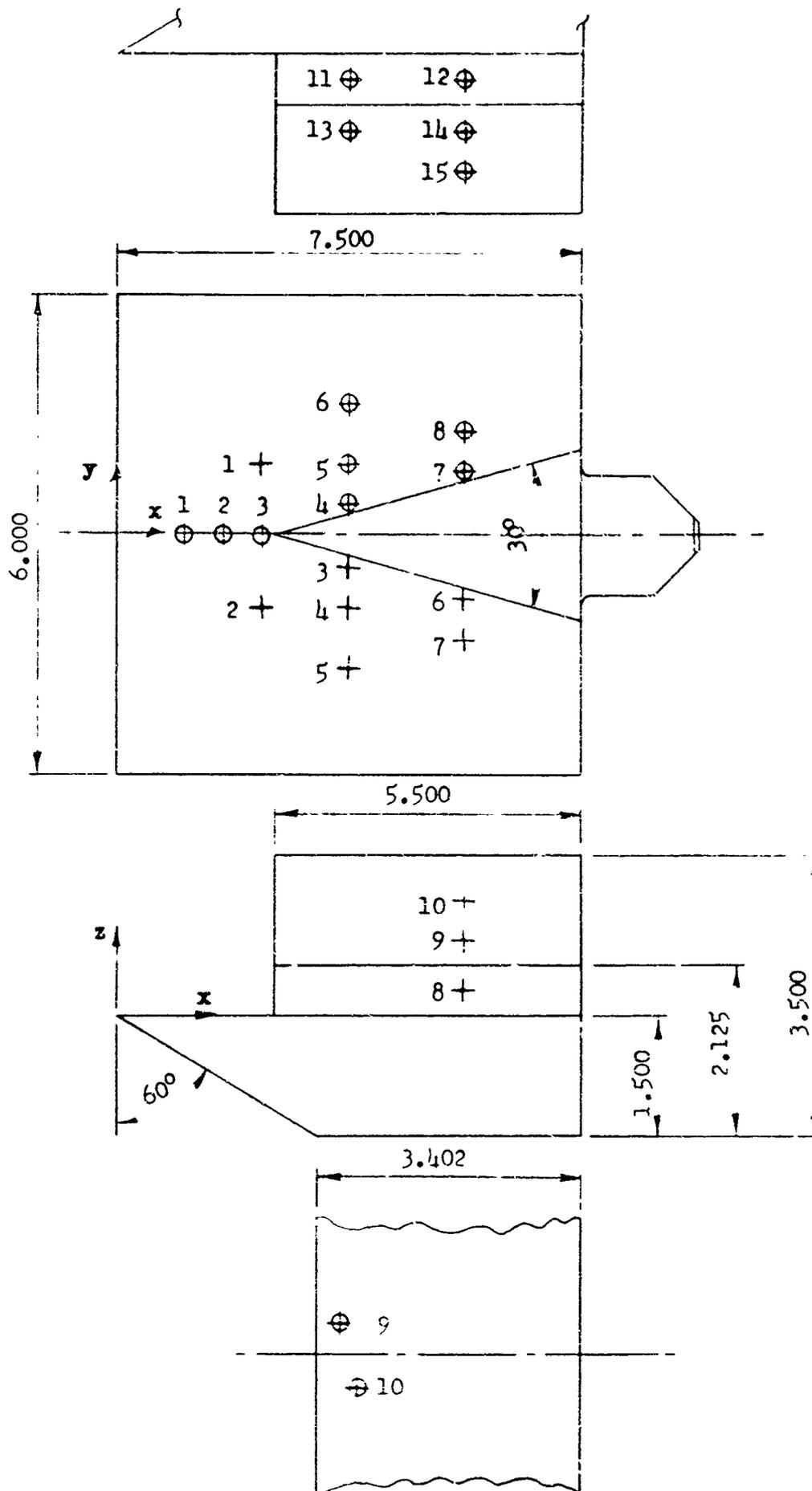
Fig. 4 Dimensions and Instrumentation for Model B
