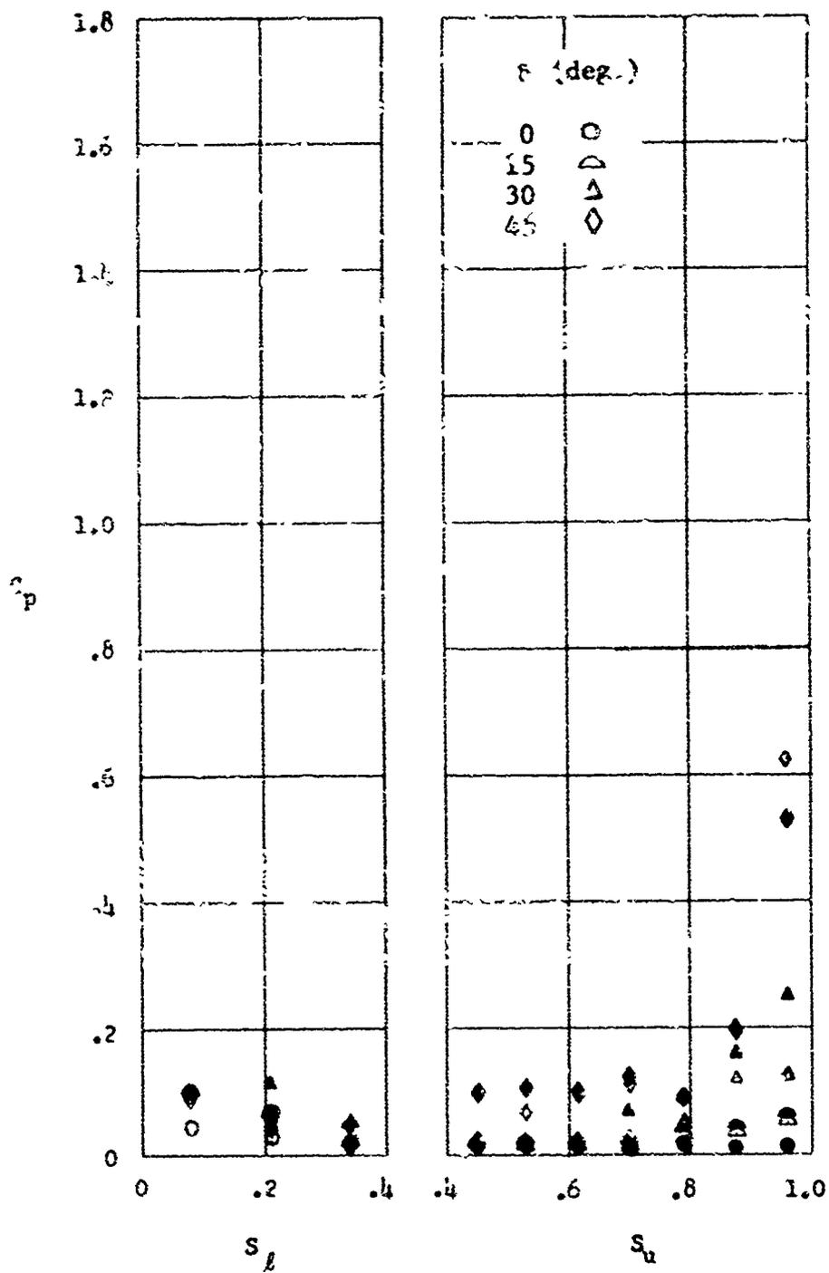
Fig. 12 chordwise Pressure Distribution for Model A<sub>7</sub>,  $M_\infty = 19$ ,  $\alpha = 0^\circ$
