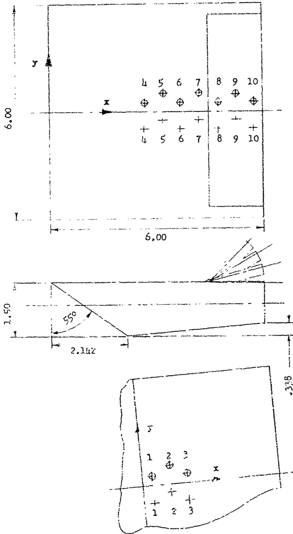
Fig. 2 Dimension and Instrumentation Location for Model A
