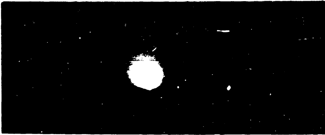
Fig. 4 - Carbon-arc searchlight at 45 km against moonlit sky. The small bright spots are extraneous horizon lights viewed directly.
