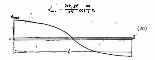
The obtained formula (20) gives the distribution of stresses longitudinally of investigated section of pipe line. In this respect maximum stresses form in places of connection of pipe line to any massive construction or to a well, reservoir, and also in sharp turns there appear significant stresses, equal  $\sigma^{\intercal}$ . Graph of distribution of the stress is shown in the figure.
